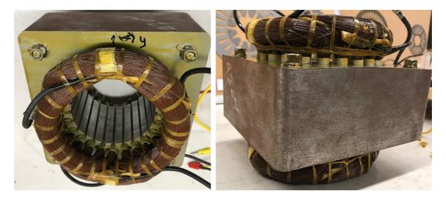
Figure 1.7: 24 Slots Induction Machine Round Single sheet tester
