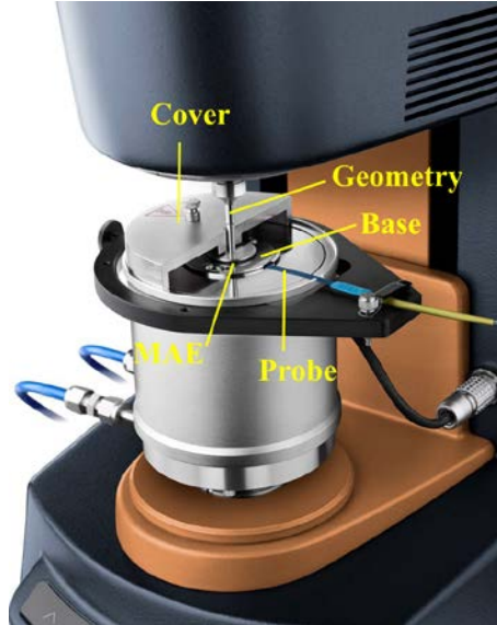
Figure 2-5. Main components of a magneto-rheometer.
