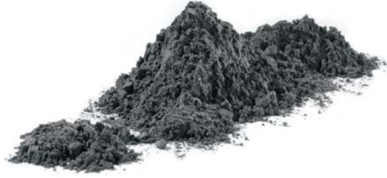
Figure 2-3. Carbonyl iron powder.
