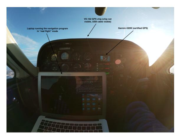
Figure 29: Setup used in flight
