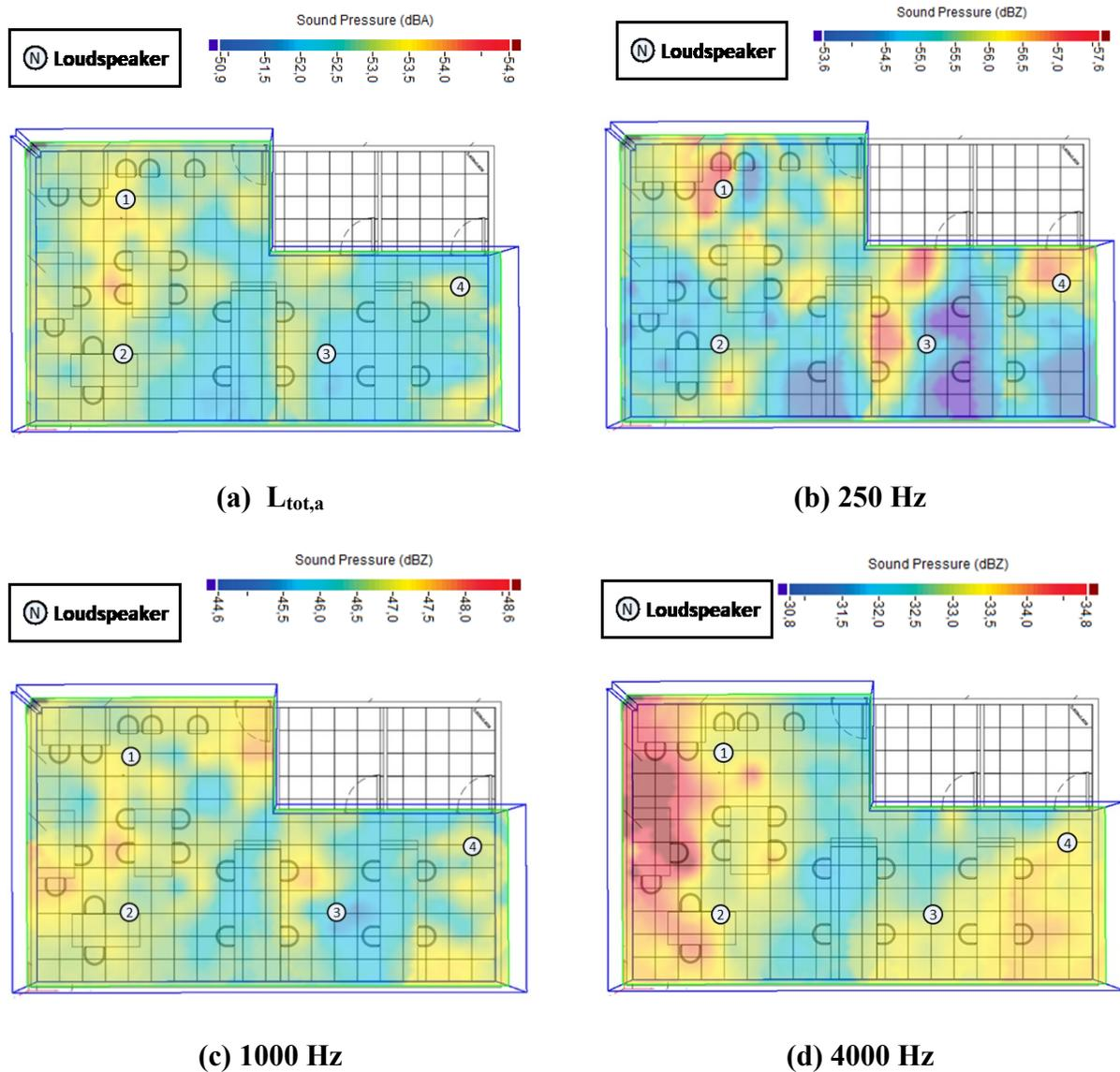
Figure 13. distribution maps using  $\pm 2$  dBA ranges for (a)  $L_{tot}$ , (b) 250 Hz, (c) 1 kHz, and (d) 4 kHz
