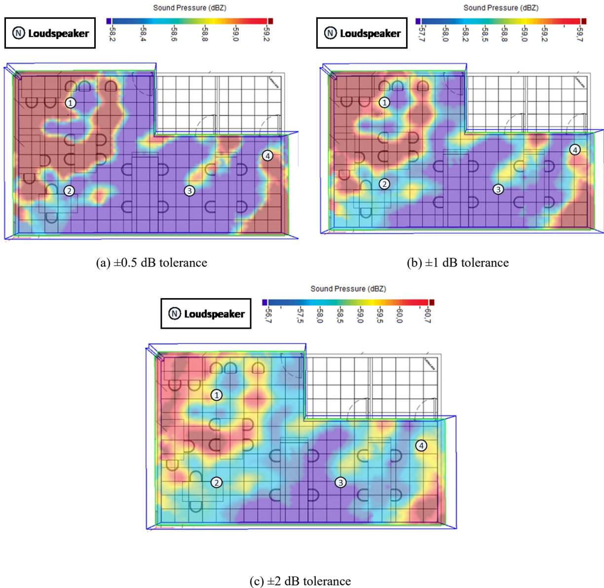
Figure 18. Sound pressure level distribution for 125 Hz using (a) 1 dB, (b) 2 dB and (c) 4 dB ranges
