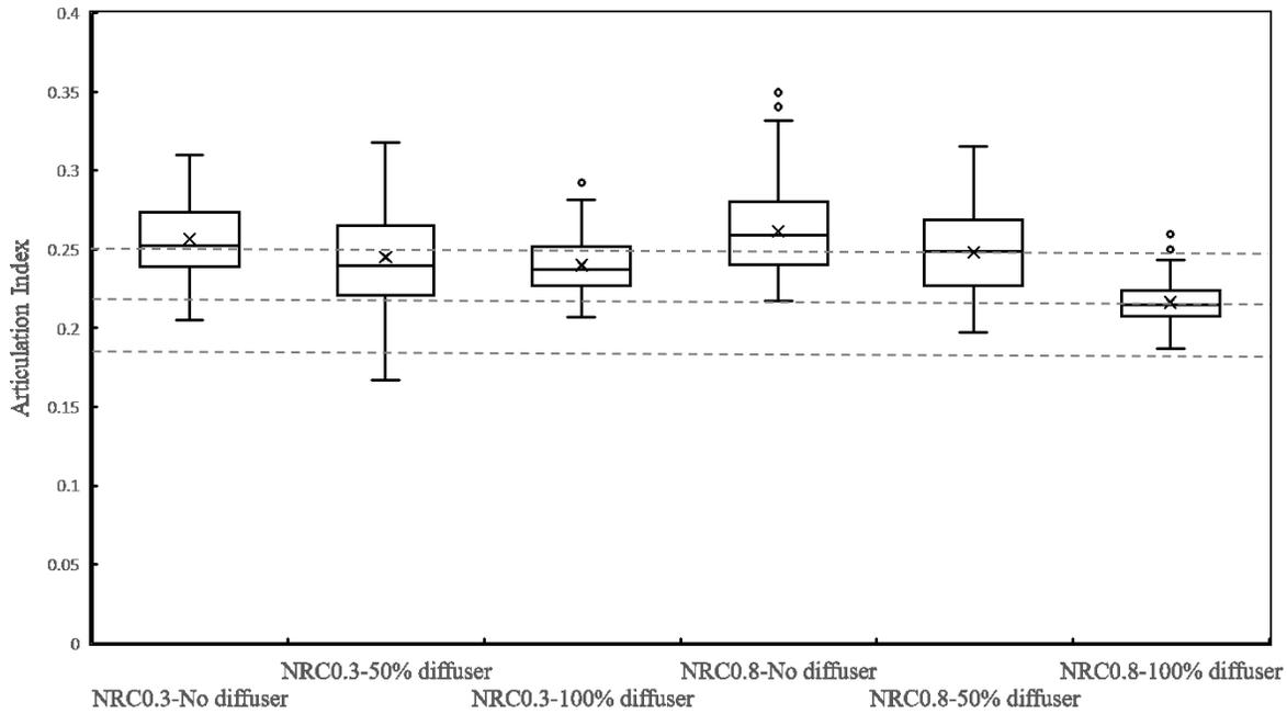
Figure 17. Effects of the scattering coefficient on the speech intelligibility. The  $L_{tot,a}$  variation of the SMS for 90% of the space for the condition with: (a) NRC 0.3-no diffuser is  $\pm 2.5$  dBA, (b) NRC 0.3-50% diffuser is  $\pm 1.5$  dBA, (c) NRC 0.3-100% diffuser is  $\pm 1$  dBA, (d) NRC 0.8-no diffuser is  $\pm 2$  dBA, (e) NRC 0.8-50% diffuser is  $\pm 1.5$  dBA, and (f) NRC 0.8-100% diffuser is  $\pm 1$  dBA.
