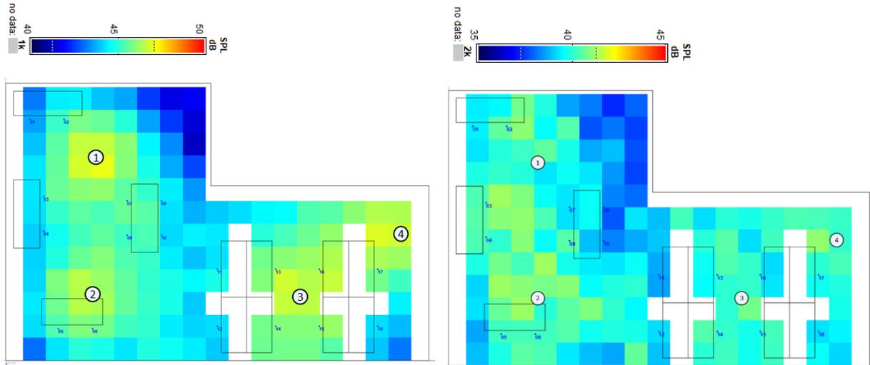
(c) Simulation results at 1k Hz ( $\pm 2.5$  dB tolerance)
