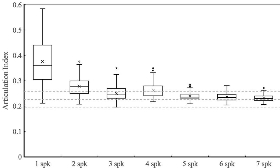
Figure 15. Effect of the number of the speakers on the speech intelligibility. The  $L_{tot,a}$  variation of the SMS for 90% of the space for the condition with: (a) 1spk for SMS is  $\pm 8.5$  dBA, (b) 2spk for SMS is  $\pm 3.5$  dBA, (c) 3spk for SMS is  $\pm 2.5$  dBA, (d) 4spk for SMS is  $\pm 2$  dBA, and (e) 5spk for SMS is  $\pm 1.5$  dBA, (f) 6spk for SMS is  $\pm 1.5$  dBA, and (g) 6spk for SMS is  $\pm 1$  dBA
