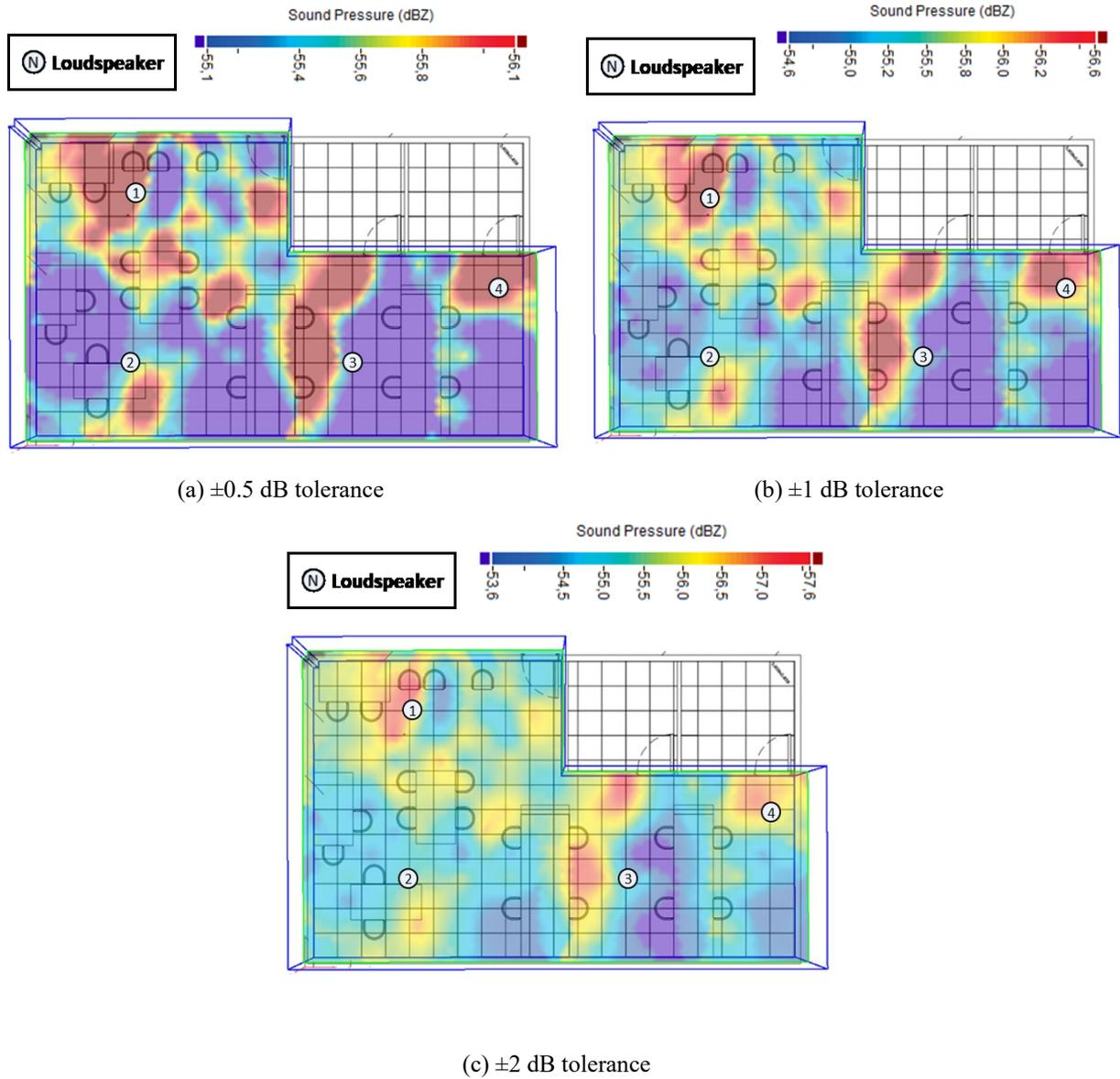
Figure 19. Sound pressure level distribution for 250 Hz using (a) 1 dB, (b) 2 dB and (c) 4 dB ranges
