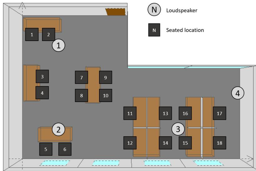
Figure 6. Office layout and the location of the sources and receivers
