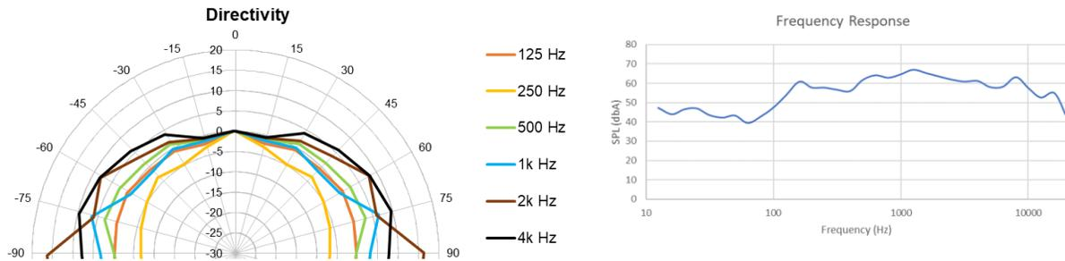
Figure 8. Directivity and the frequency response of the STR loudspeaker [57]
