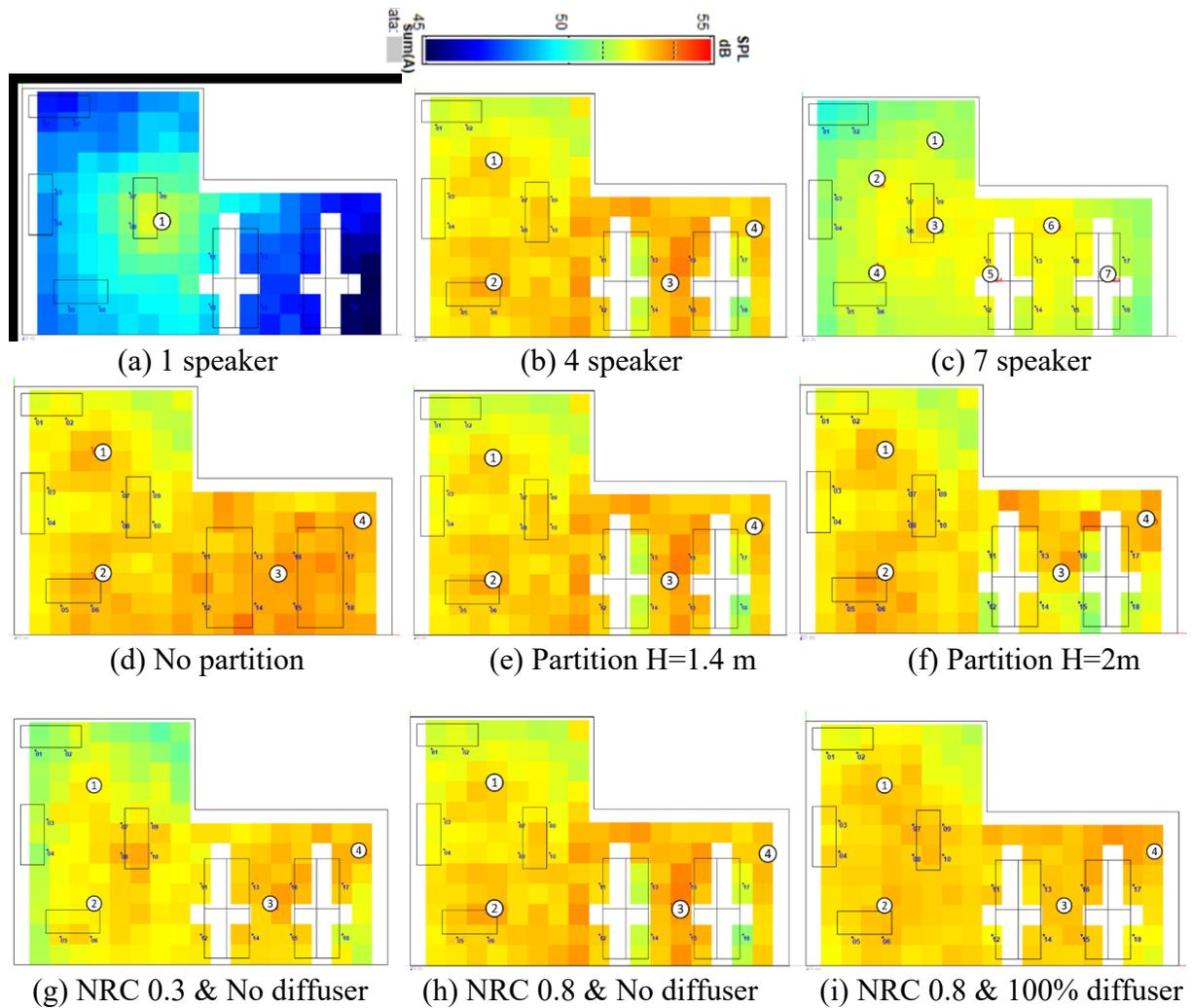
Figure 14. SPL distributions with physical parameters (loudspeakers, partitions' height and ceiling absorption & scattering properties)
