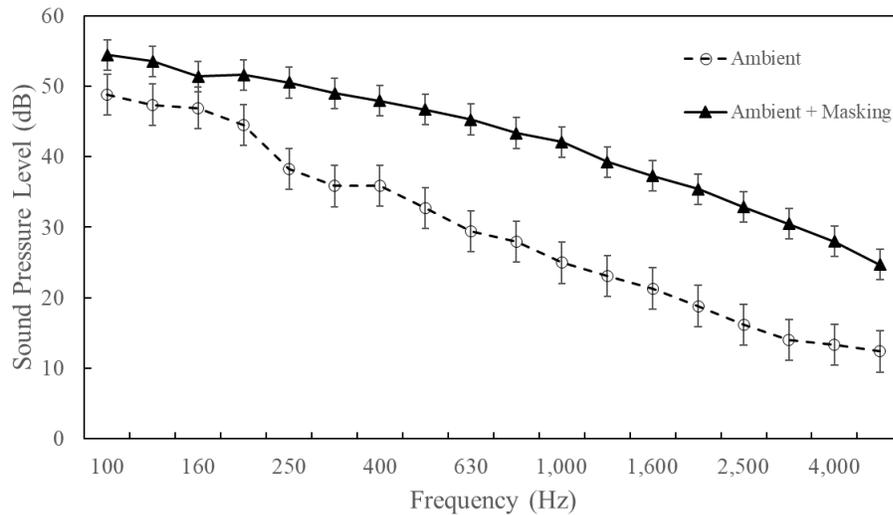
Figure 5. Average SPL of the whole space without the masking sound (Ambient) and with the masking sound (Ambient + Masking)
