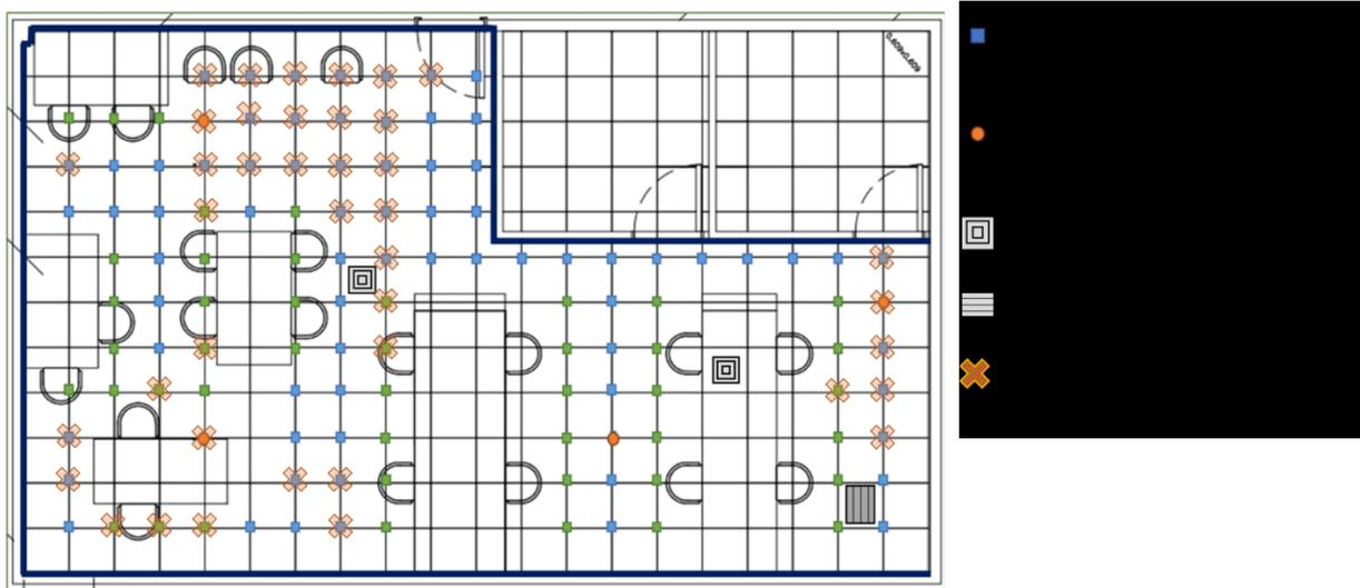
Figure 11. Positions of the excluded measured points which are affected by the background sound
