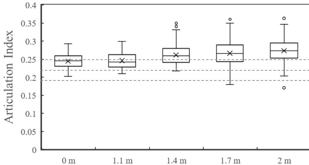
Figure 16. Effect of the partition height on the speech intelligibility. The  $L_{tot,a}$  variation of the SMS for 90% of the space for the condition with: (a) No partition is  $\pm 1.5$  dBA, (b) 1.1m partition height is  $\pm 1.5$  dBA, (c) 1.4m partition height is  $\pm 2$  dBA, (d) 1.7m partition height is  $\pm 2.5$  dBA, and (e) 2m partition height is  $\pm 2.5$  dBA
