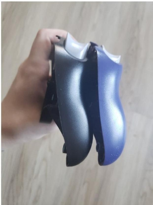
**Figure VI 2** shell backs of a GameCube controller. The black/first one includes the spring resistance in the triggers, the second/purple shell has the springs removed. This is a common hardware mod for SSBM. This image shows the slight height difference for controller triggers. Many people only do this mod to one side. It is entirely player specific and subjective to a player's preferred controller feel.
