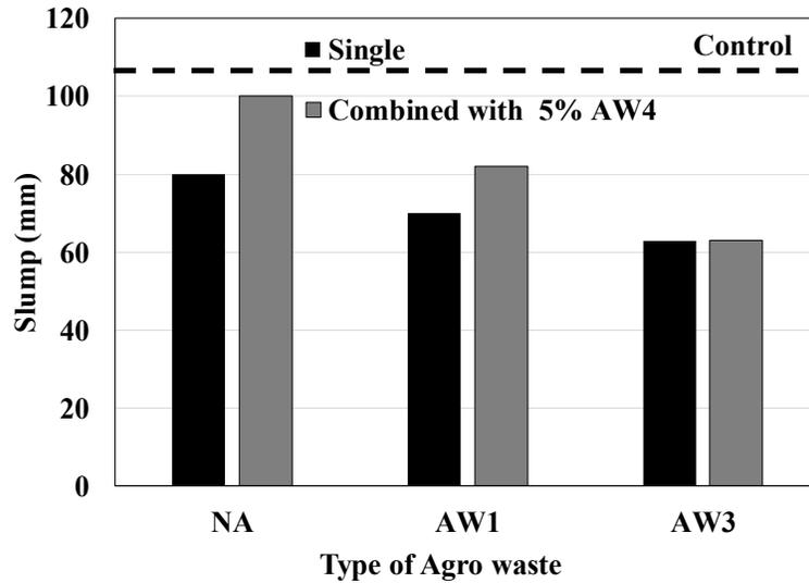
Figure 3.13 Slump for mixtures incorporating natural aggregate and agro-waste materials separately and combined.
