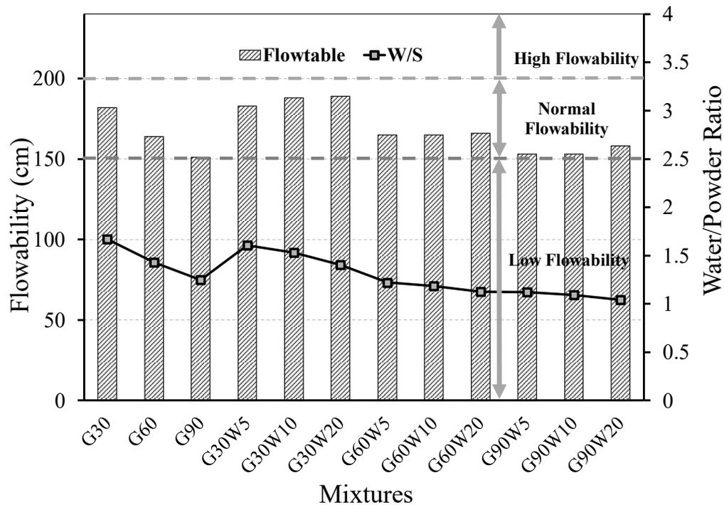
Figure 4.1: Flowability results for all tested CLSM mixtures.
