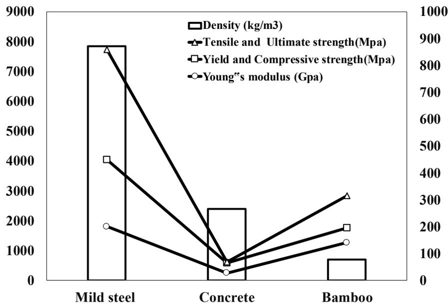
Figure 2.5: Comparison of properties between Mild Steel, Concrete and Bamboo [85, 87]
