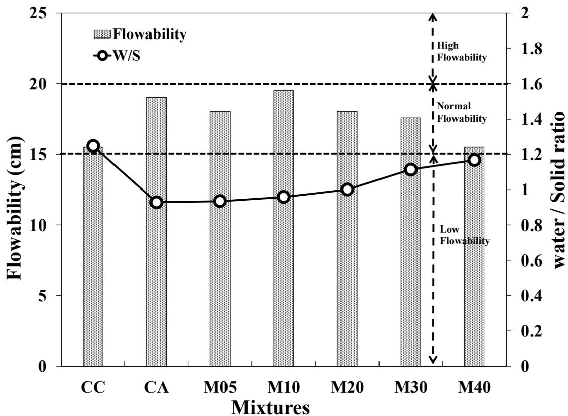
Figure 5.1 Flowability for all tested CLSM mixtures
