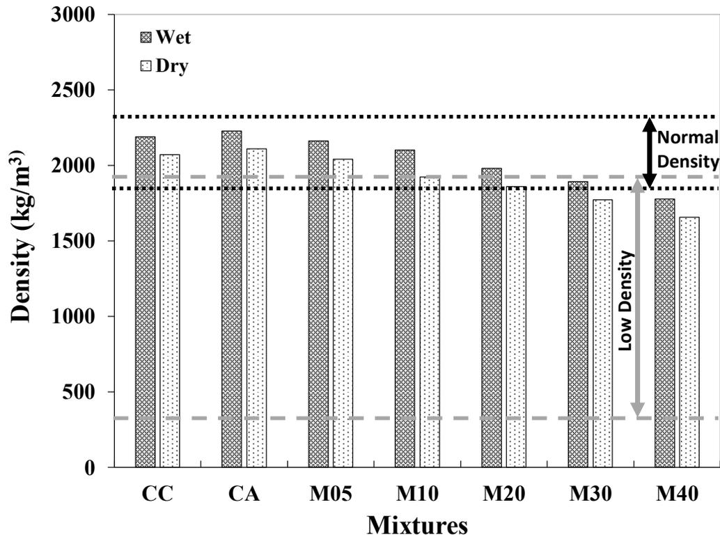
Figure 5.4 Wet and Dry densities for CLSM mixtures
