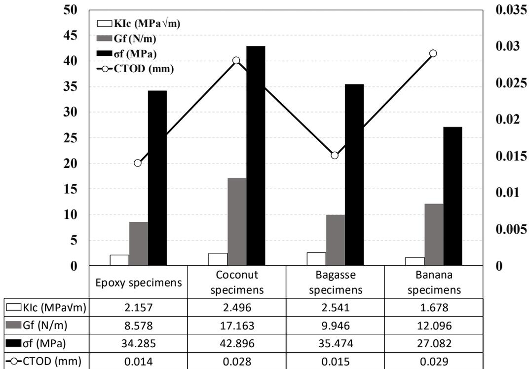
Figure 2.6 Comparison between bananas, bagasse, coconut agro-waste as fibre and epoxy concrete [after 94]
