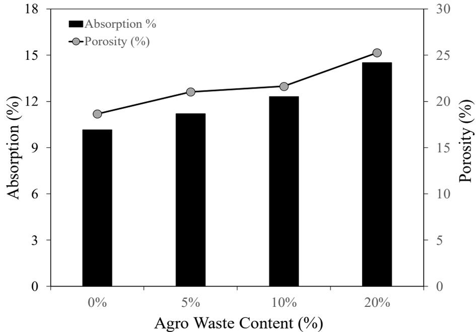
Figure 4.8 Absorption and porosity for 90 kg/m<sup>3</sup> CLSM mixture with various agro-waste contents
