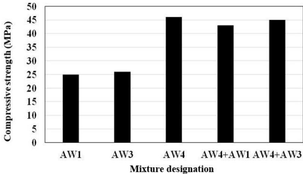
Figure 3.17 Compressive strength for concrete mixtures incorporating 40% agro-waste materials.
