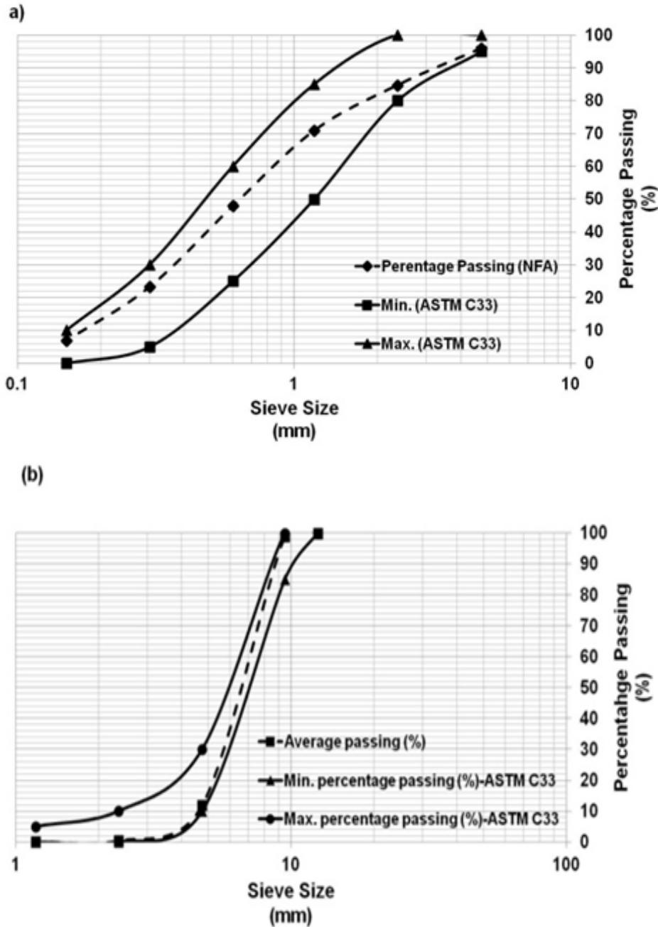
Figure 3.9 Sieve analysis of aggregate (a) Fine aggregate, and (b) Coarse aggregate
