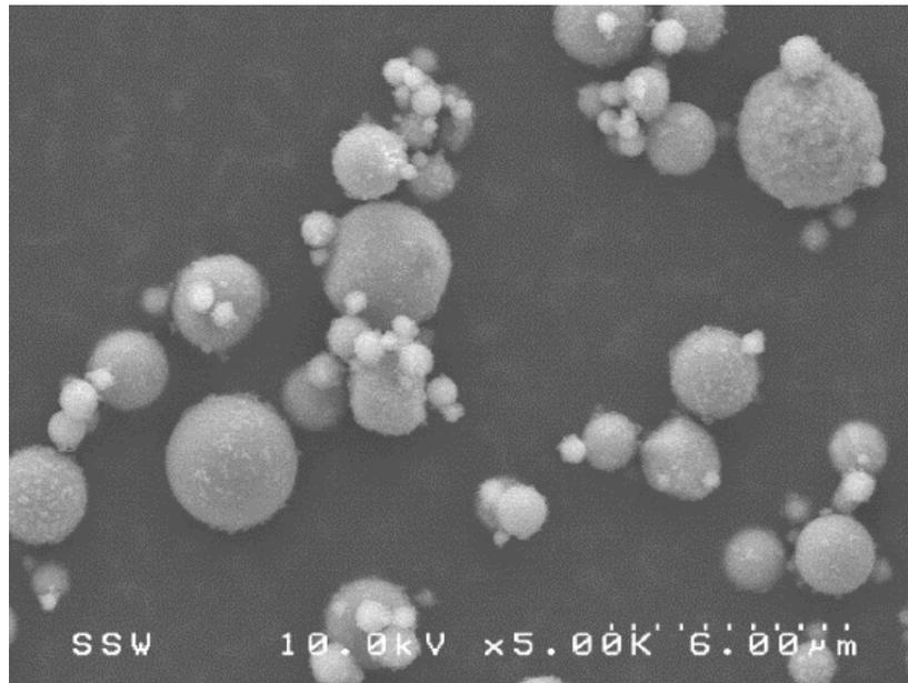
Figure 5.2 spherical particle shape for the used FA.
