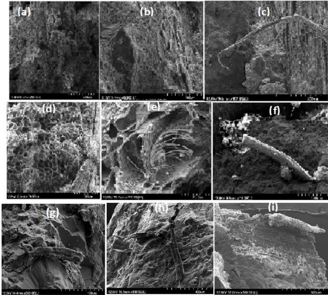
Figure 3.20 SEM images of fresh fracture of different sample concrete used the ago waste materials(a) AWM1-20%, (b) AWM1-30%, (c) AWM1-40%, (d): AWM3-20%, (e) AWM3-30%, (f): AWM3-40%, (g) AWM4-3%, (h) AWM4-5%, (i) AWM4-7%.
