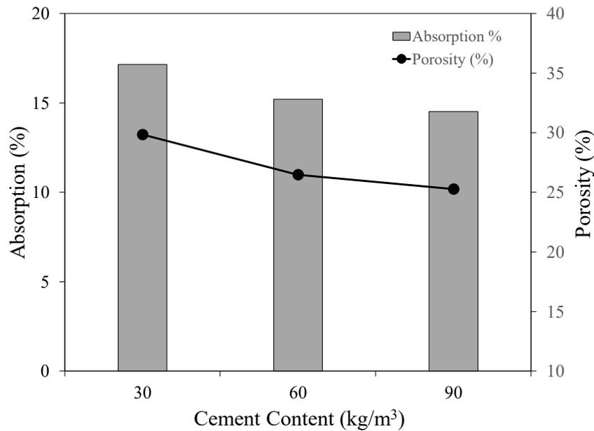
Figure 4.9 Absorption and porosity for CLSM mixture with 20% agro-waste and different cement contents
