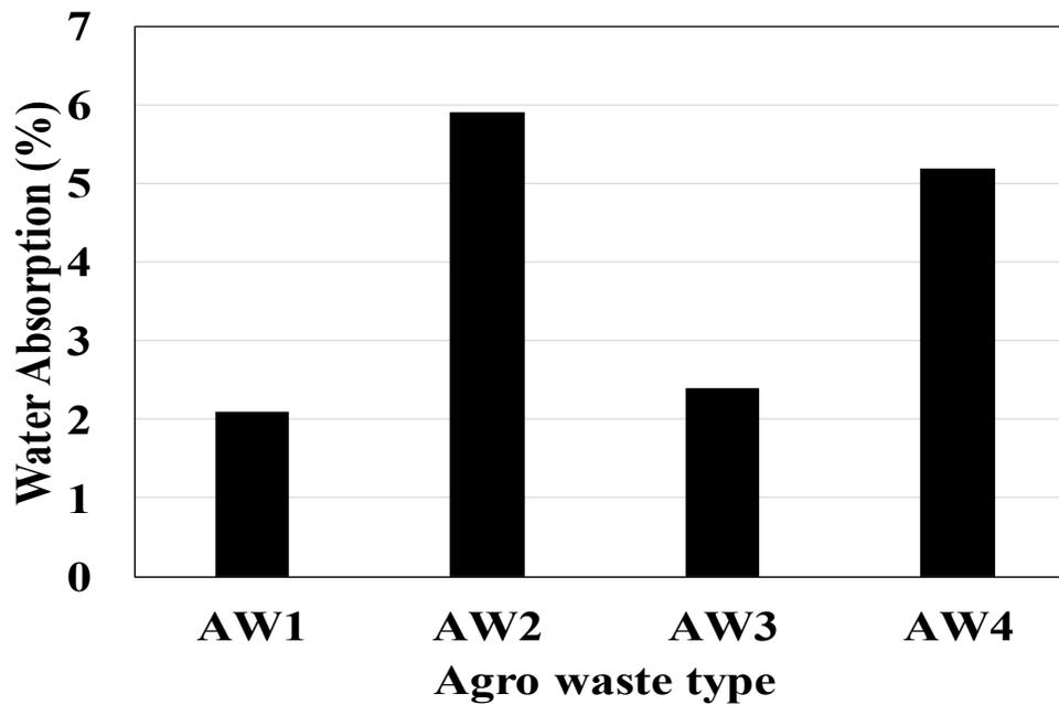
Figure 3.5 Water absorption values as received samples of different agro-waste materials.
