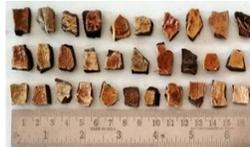
Figure 2.13 Coconut shell as Aggregates[114]
