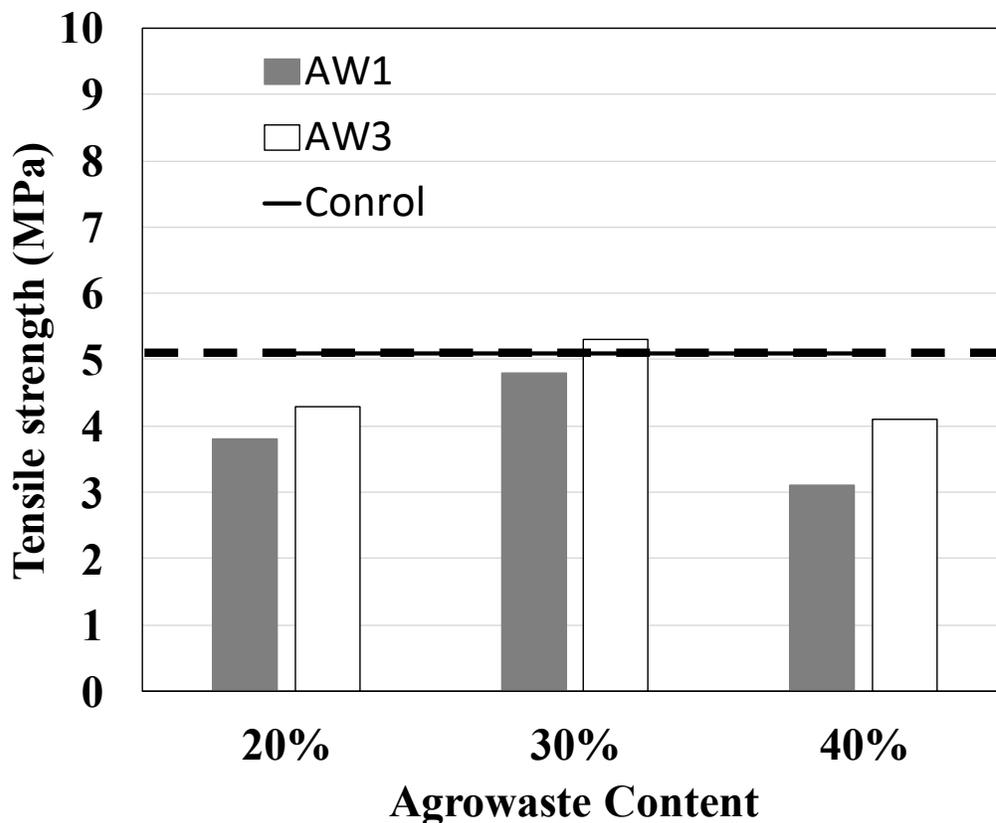
Figure 3.18 Tensile strength for agro concrete with various contents.
