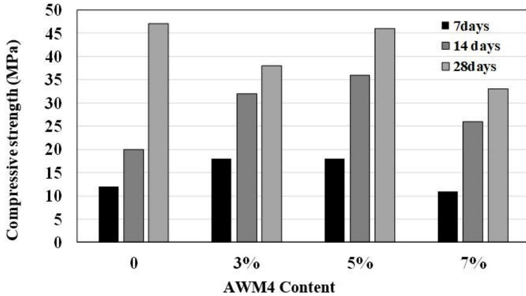
Figure 3.16 Compressive strength for concrete mixtures incorporating various contents of AWM4.
