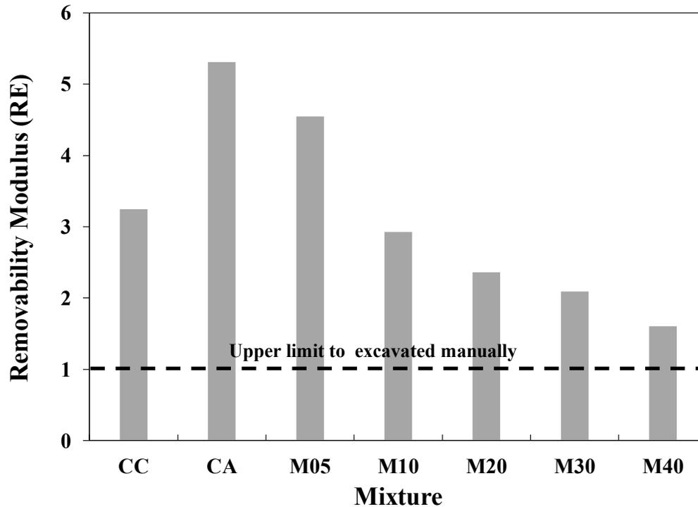
Figure 5.6 RE values for all tested CLSM mixtures.
