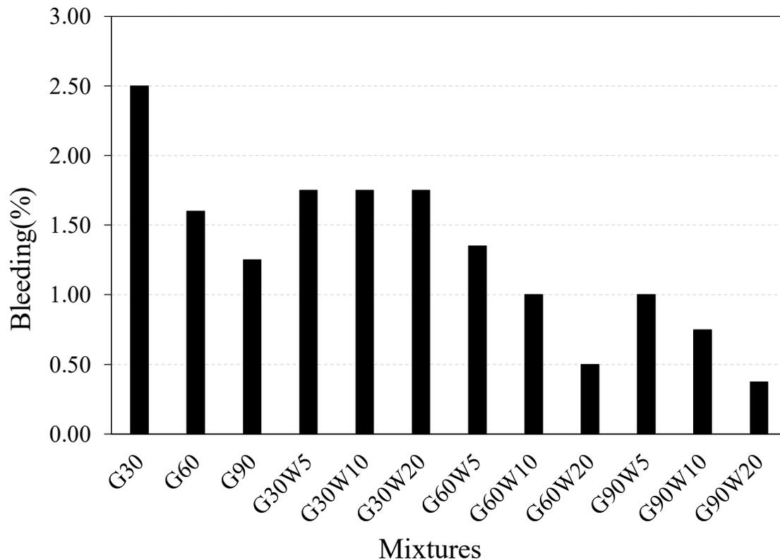
Figure 4.2 Bleeding results for all tested CLSM mixtures
