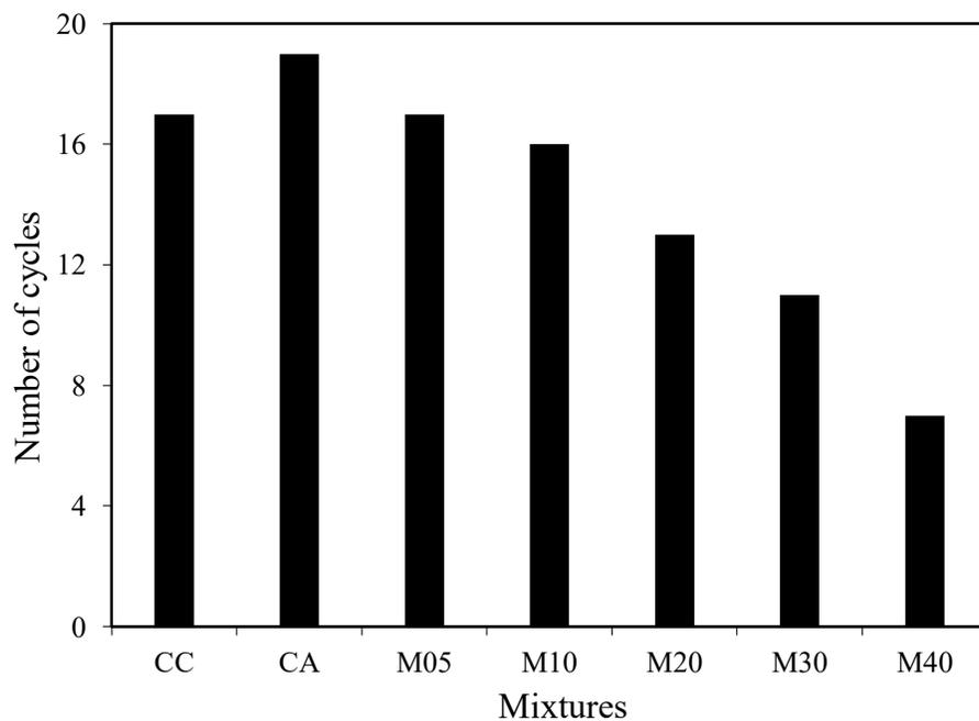
Figure 5.13 Numbers of sustained cycles in sulphate solution for all CLSM mixtures.
