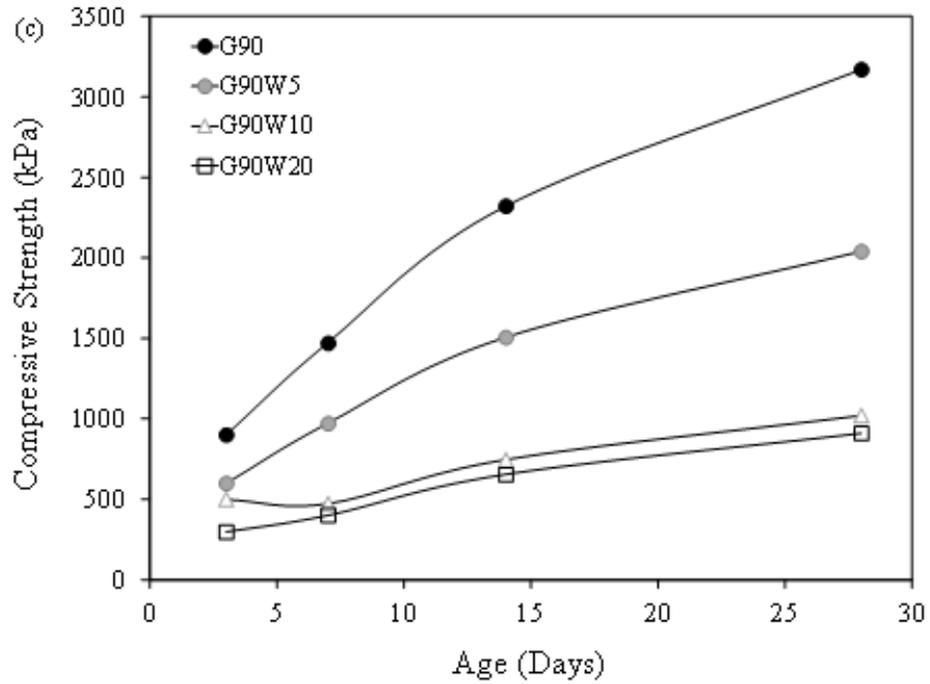
Figure 4.4 Compressive strength development for tested CLSM with cement contents a) 30 kg/m<sup>3</sup>, b) 60 kg/m<sup>3</sup> and c) 90 kg/m<sup>3</sup>.
