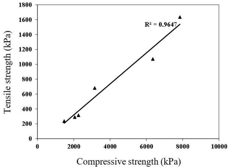
Figure 5.8 Correlation between splitting tensile strength and corresponding compressive strength.
