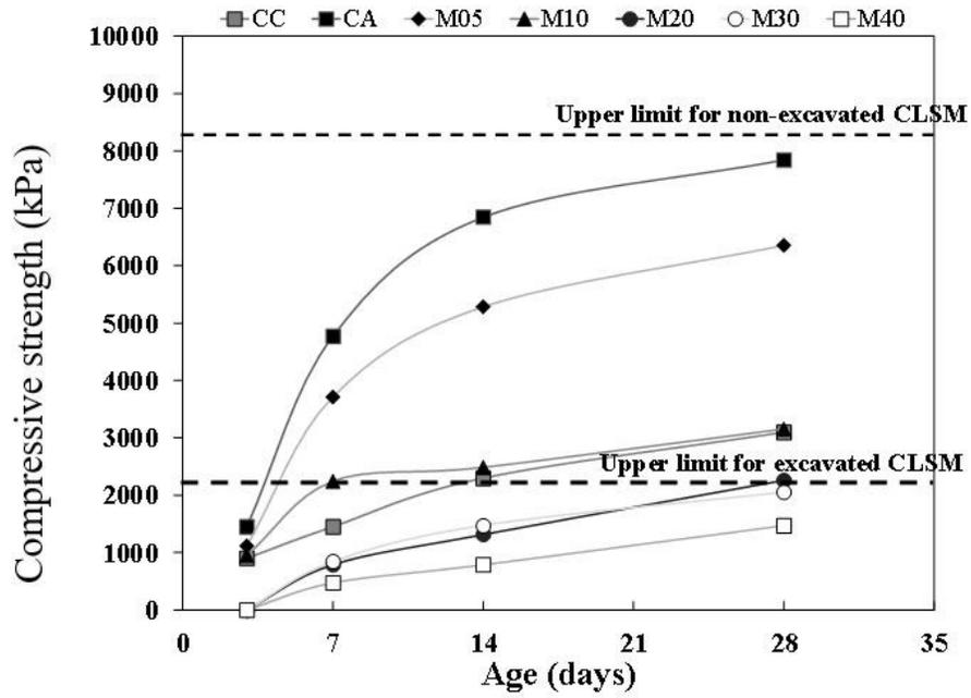
Figure 5.5 Compressive strength development for CLSM mixtures
