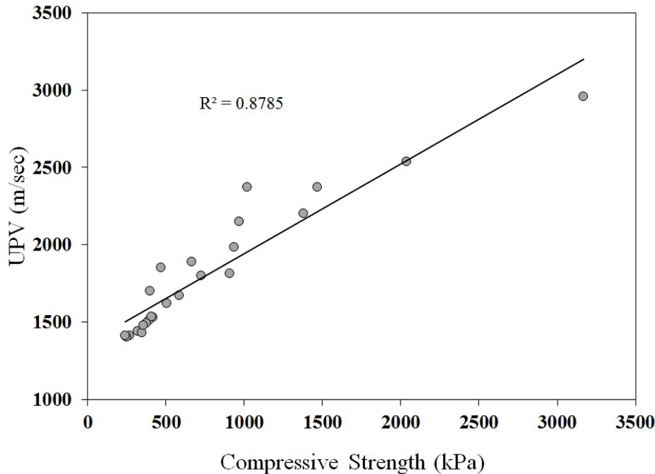
Figure 4.11 Relationship between measured Ultrasonic pulse velocity and achieved compressive strength for all CLSM mixtures.
