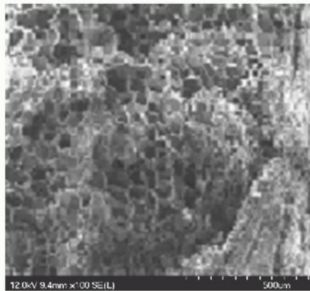
Figure 5.10 SEM showing the porous microstructure for agro-waste materials
