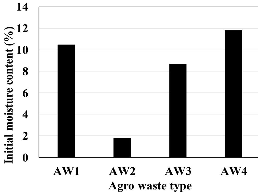
Figure 3.3 Moisture contents for as received samples of different agro-waste materials
