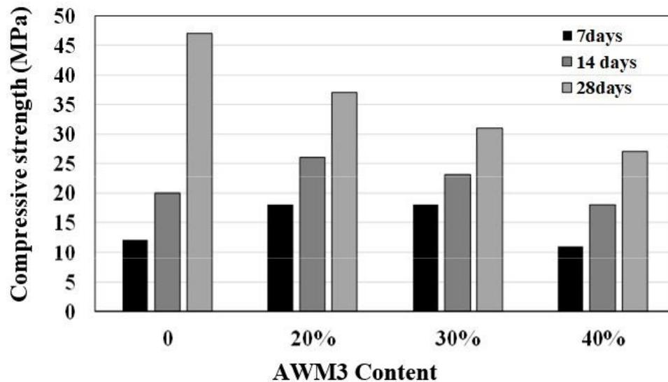
Figure 3.15 Compressive strength for concrete mixtures incorporating various contents of AWM3.
