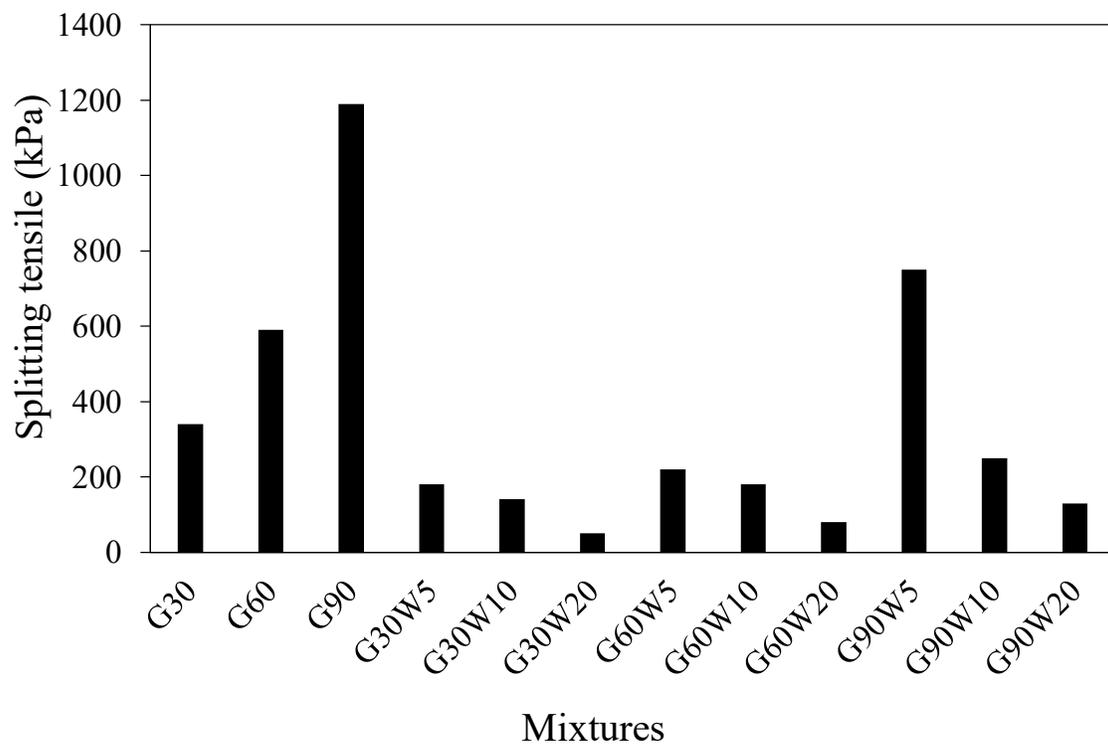
Figure 4.6 Splitting tensile strength for all CLSM mixtures.
