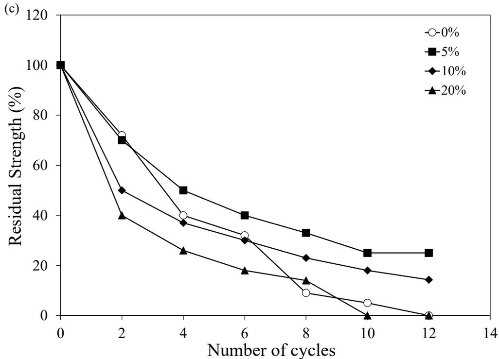
Figure 4.14 Contd': Residual strength for CLSM mixtures incorporating different agro-waste content and cement content of a) 90 kg/m<sup>3</sup>, b) 60 kg/m<sup>3</sup>, and c) 30 kg/m<sup>3</sup>.
