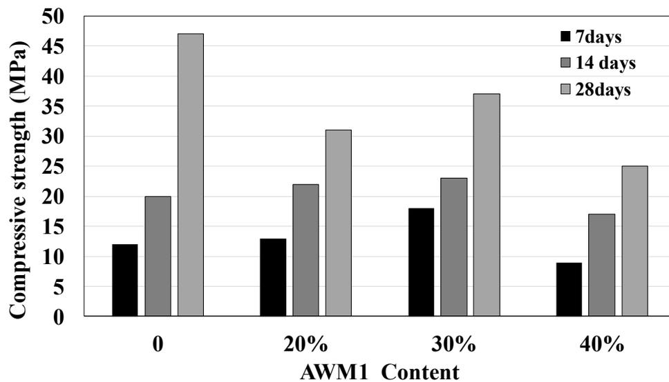
Figure 3.14 Compressive strength for concrete mixtures incorporating various contents of AWM1
