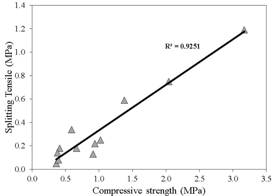
Figure 4.7 Relationship between splitting tensile strength and achieved compressive strength for all CLSM mixtures.
