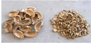
Figure 2.12 Rubber seed shell (left side) and crushed rubber seed shell (right side)[110]
