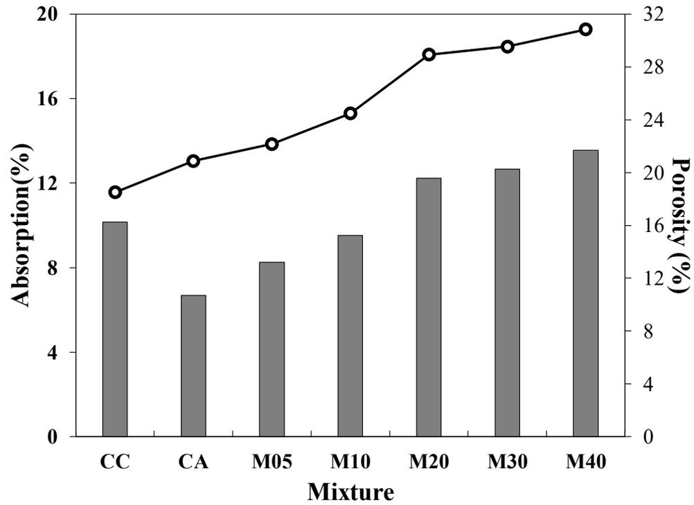
Figure 5.9 Absorption rate and total porosity for tested CLSM mixtures
