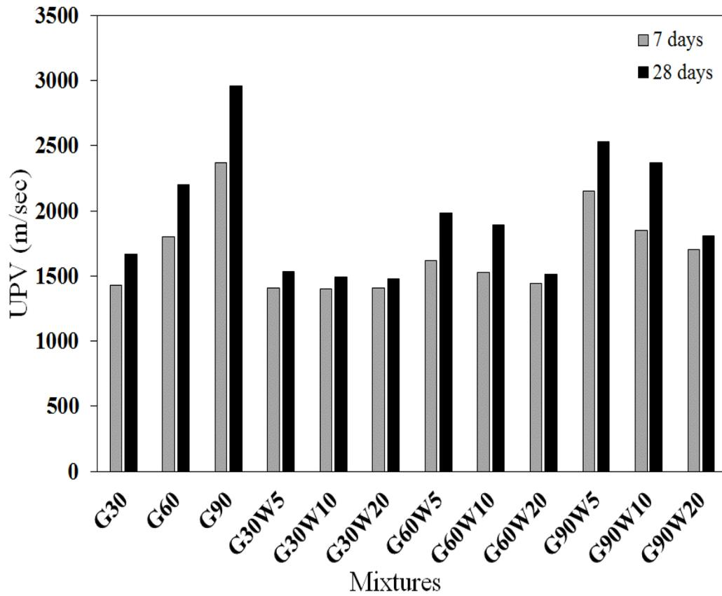
Figure 4.10 Ultrasonic pulse velocity for all tested CLSM mixtures at different ages
