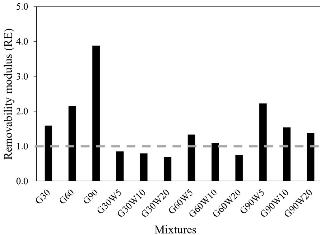
Figure 4.5 RE values for all tested CLSM mixtures.
