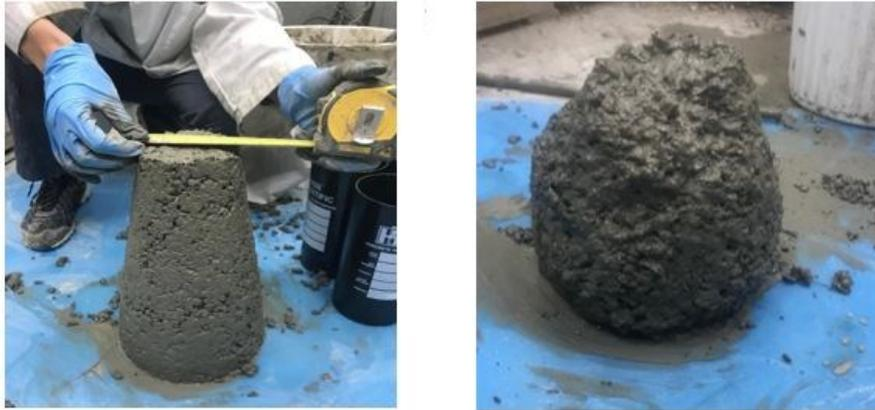
Figure 3.10 Slump test for mixtures with different agro-waste materials
