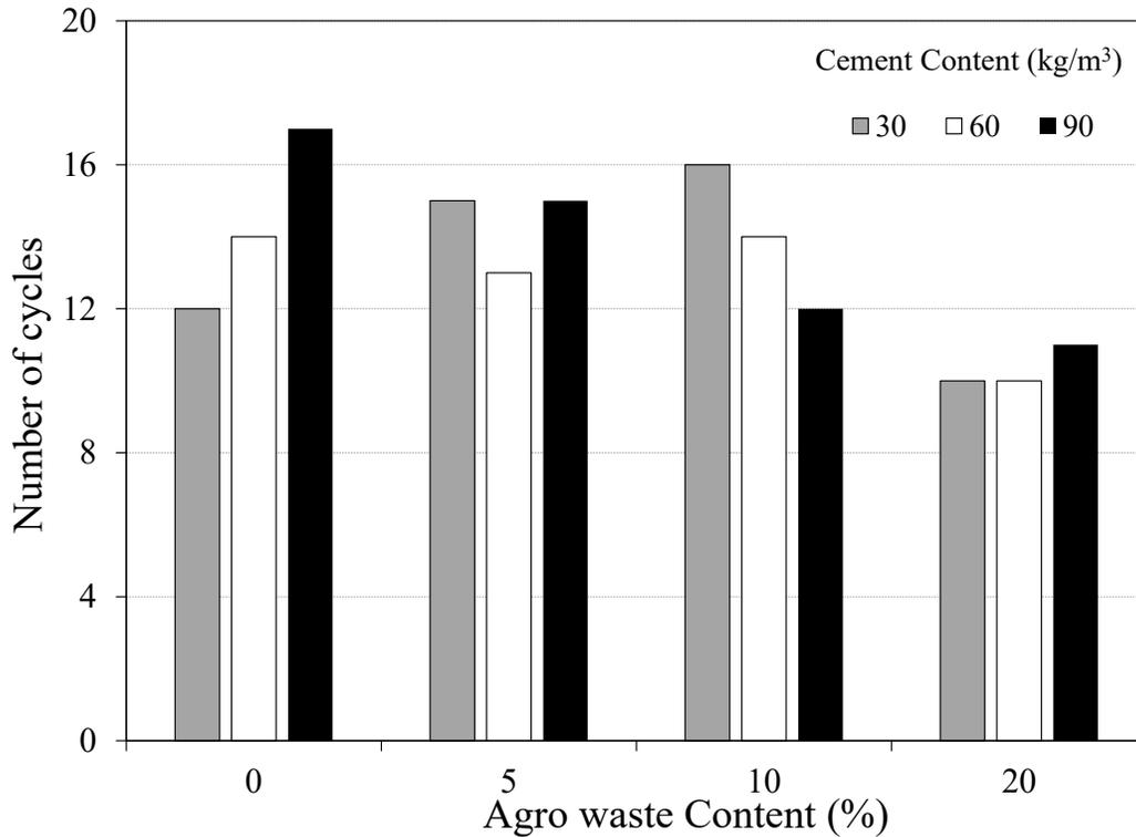
Figure 4.13 Numbers of sustained cycles in sulphate solution for all CLSM mixtures
