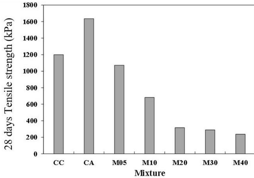
Figure 5.7 Tensile strength for CLSM mixtures at age 28 days.
