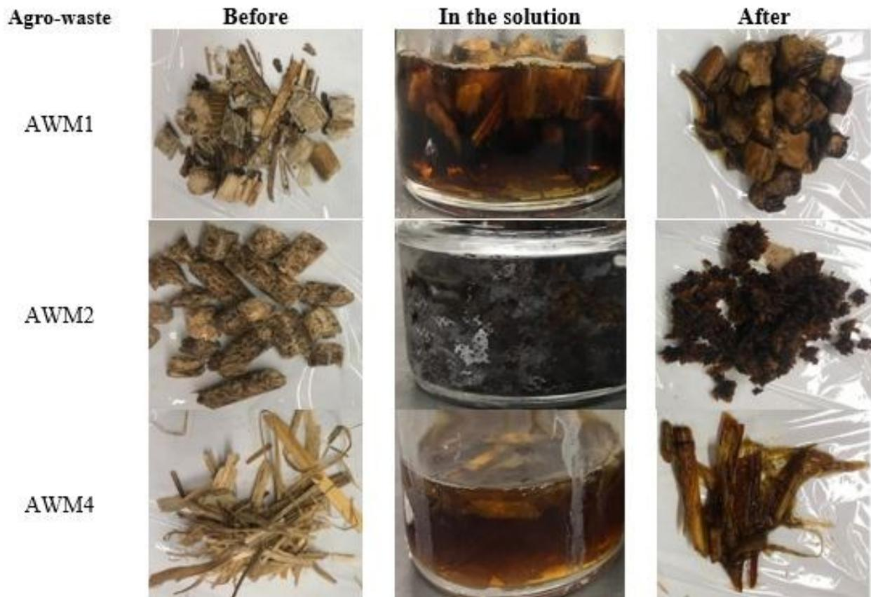
Figure 3.8 Agro-waste materials before and after submerging in alkali solution.
