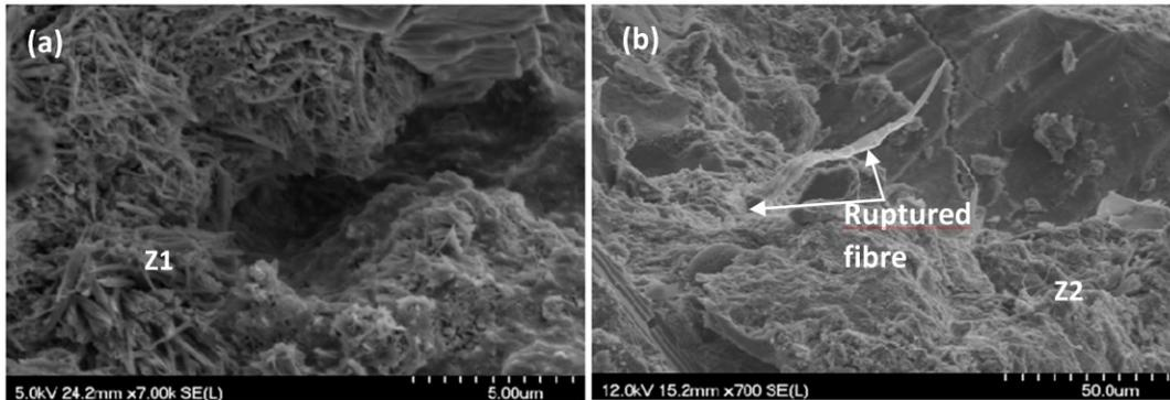
Figure 3.22 Microscope image of concrete made of agro-waste materials: a) 35%AWM1+5%AWM4, (b) 35%AWM3+5%AWM4. Z1 fewer ettringite needles, Z2: C-S-H gel
