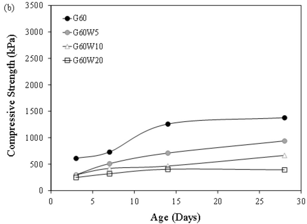
Figure 4.3 Compressive strength development for tested CLSM with cement contents a)  $30 \text{ kg/m}^3$ , b)  $60 \text{ kg/m}^3$  and c)  $90 \text{ kg/m}^3$ .
