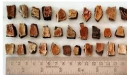
Figure 2.13 Coconut shell as Aggregates[114]
