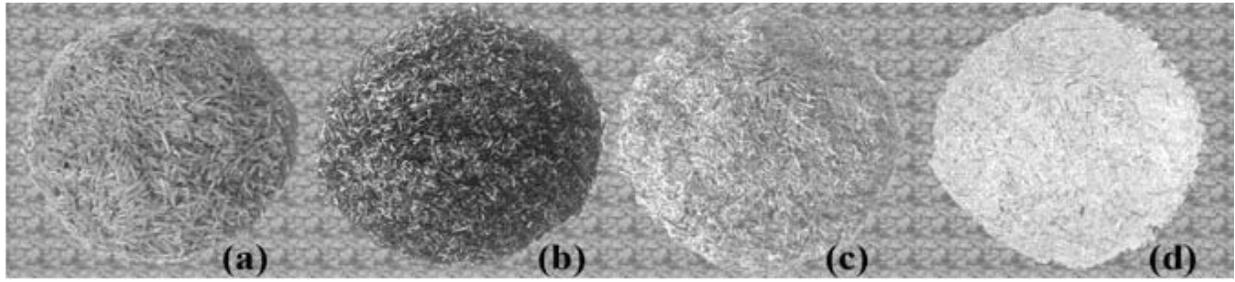
Figure 2.18 (a) Rice husk, (b) Rice Husk Ash with high carbon amount, (c) optimum Rice Husk Ash, (d) Rice Husk Ash with crystalline silica [14]
