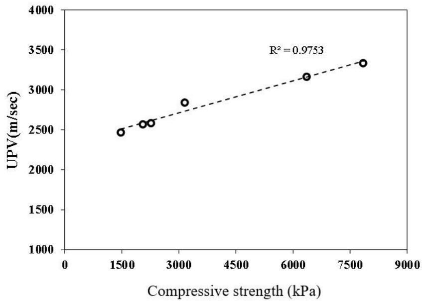
Figure 5.12 Relationship between measured UPV and 28 days compressive strength for AAM-CLSM mixtures
