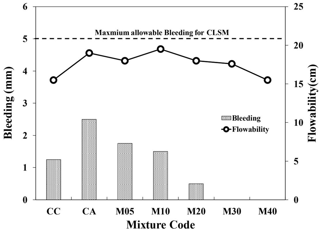
Figure 5.3 Bleeding for all tested CLSM mixtures
