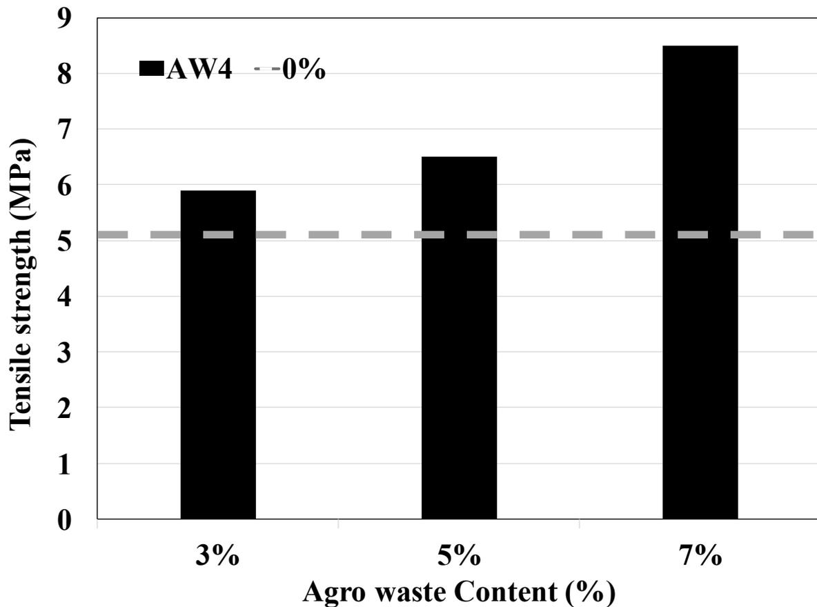
Figure 3.19 Tensile strength for agro concrete with various contents of AWM4
