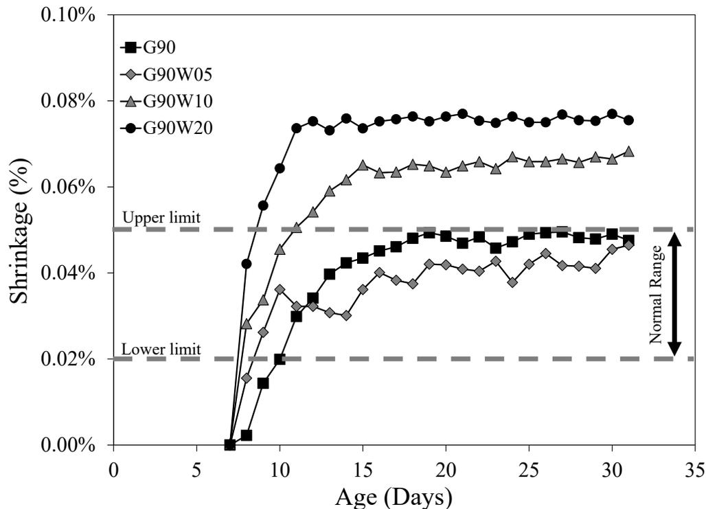
Figure 4.12 Shrinkage development for 90 kg/ m<sup>3</sup> CLSM mixtures.
