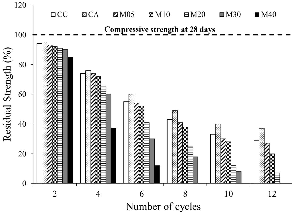
Figure 5.14 Residual strength for CLSM mixtures incorporating different agro-waste content.
