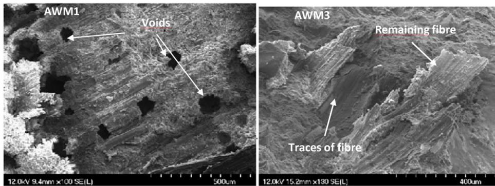
Figure 3.21 Microscope image of concrete made of agro-waste materials (AWM1 and AWM3).
