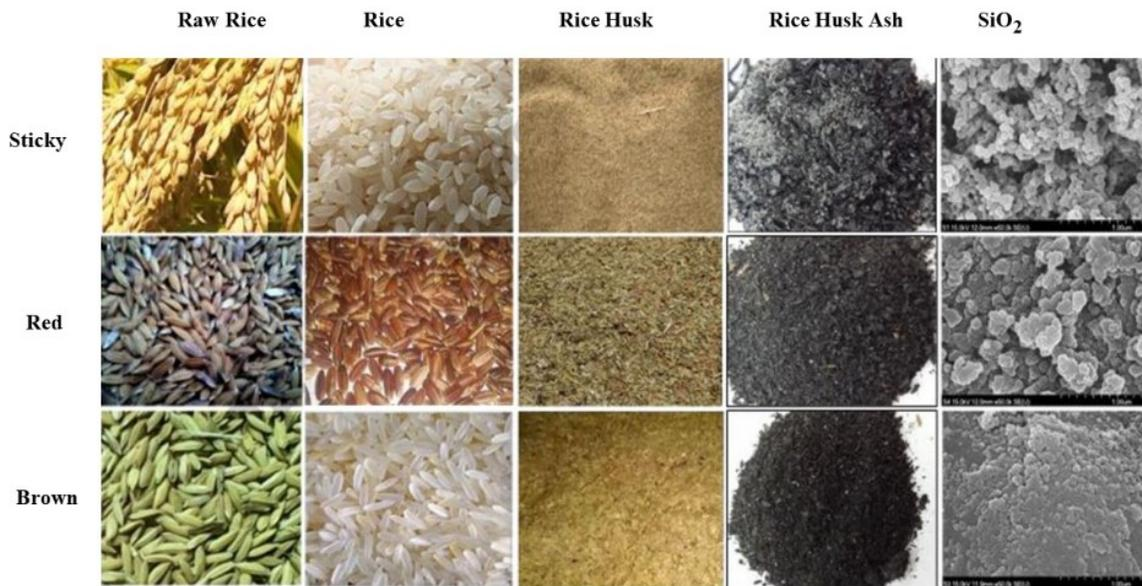
Figure 2.19 Rice from different locations and type in the process of preparation[81]
