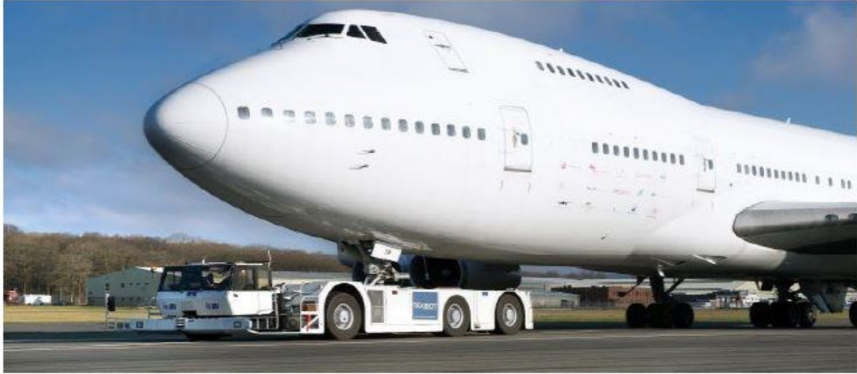
Figure 33. Operation of a Towbarless towing truck((Ricardo, 2011)
