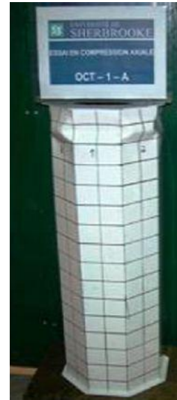
(b) Deformed shape of Octagonal section obtained from experiment (Godat et. al. 2012)
