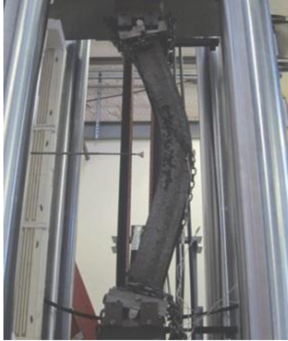
(a) Global buckling failure
