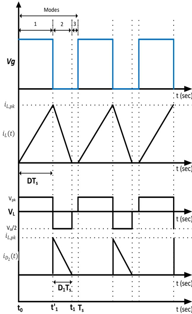
Fig. 3. 9. Waveforms for one switching cycle
