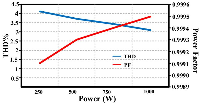
Fig. 3. 15. THD and power factor at various power levels
