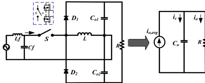
Fig. 3. 11. Equivalent circuit for small signal modelling
