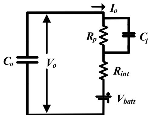
Fig. 2.15 Battery Equivalent circuit when connected to battery charger.
