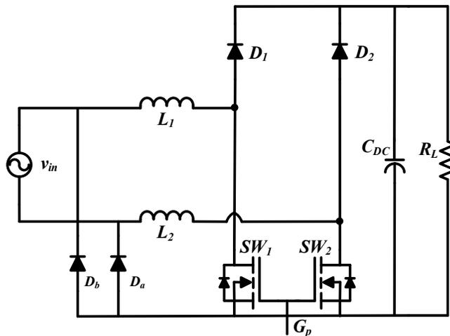
Fig. 3. 2. Semi-bridgeless boost PFC converter
