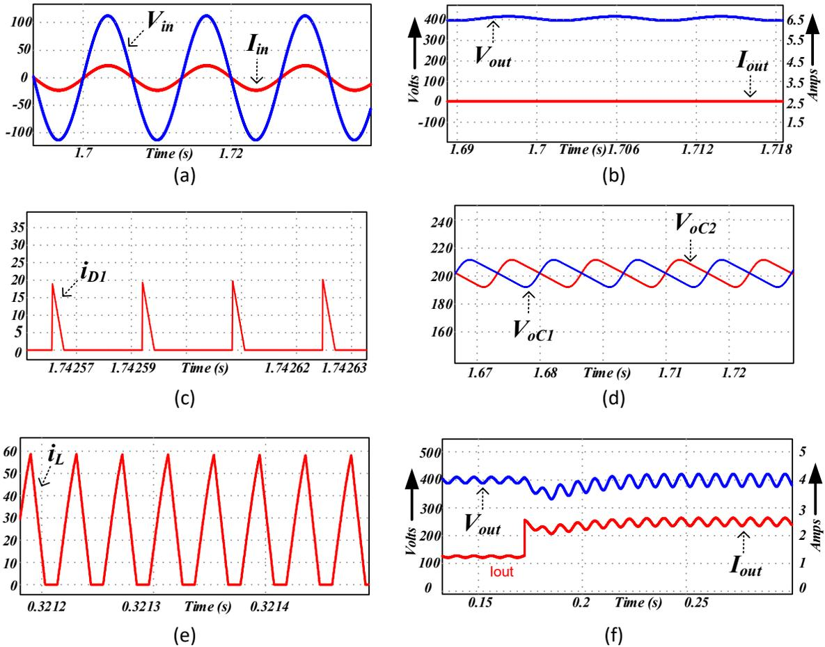
Fig. 3. 12. Simulation results (a) input voltage and input current; (b) output voltage and output current; (c) output diode  $D_{01}$  current; (d) output capacitors voltages; (e) inductor current; (f) converter response for load change 50 % to 100 %.
