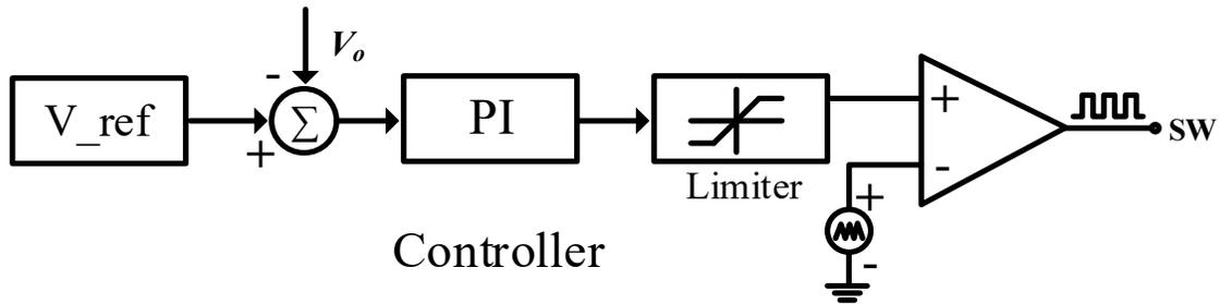
Fig. 2.6. The control circuit for the studied converter.
