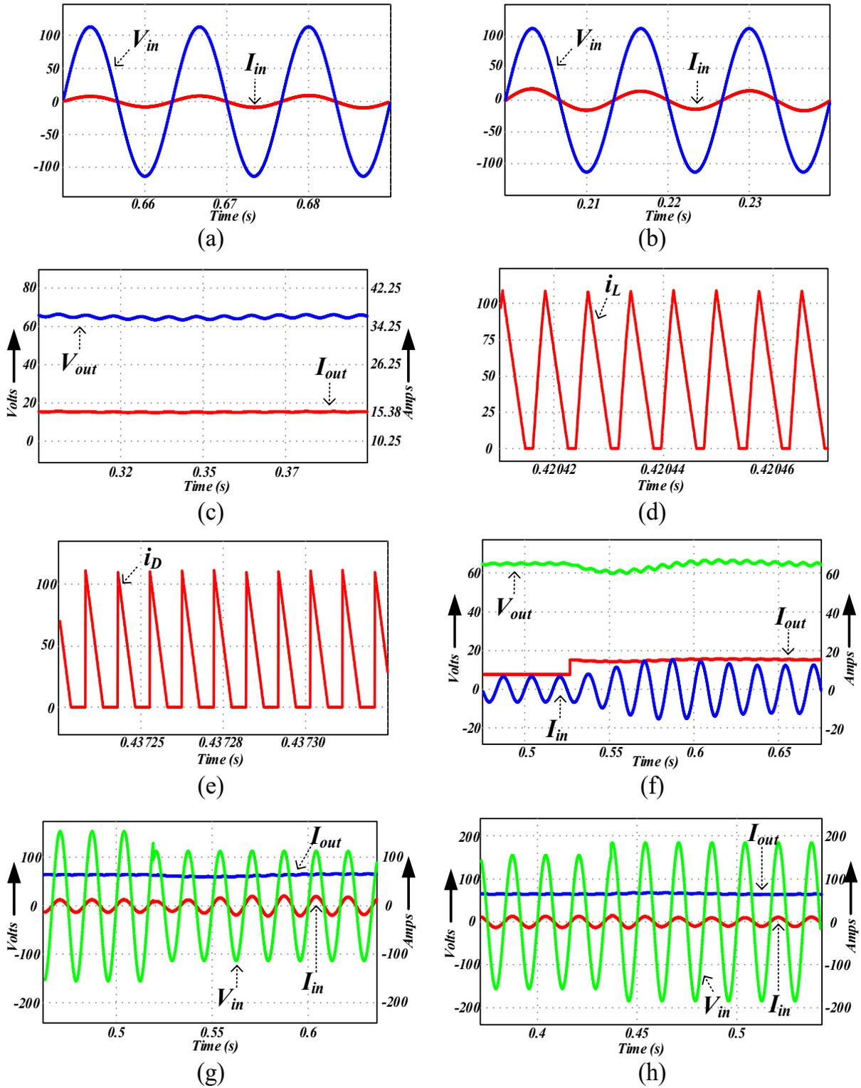
Fig. 2. 10. Simulation results (a) input voltage and input current at 250W; (b) input voltage and input current at 1kW (c) output voltage and output current; (d) inductor current; (e) output diode current; (f) load change from 100% to 10%; (g) input voltage change from 110 V to 80 V. (h) input voltage change from 110 V to 130 V.
