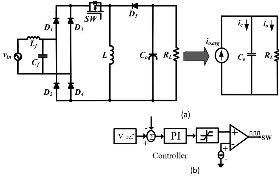
Fig. 2. 9. (a) Equivalent circuit for small signal modelling. (b) Control Diagram.
