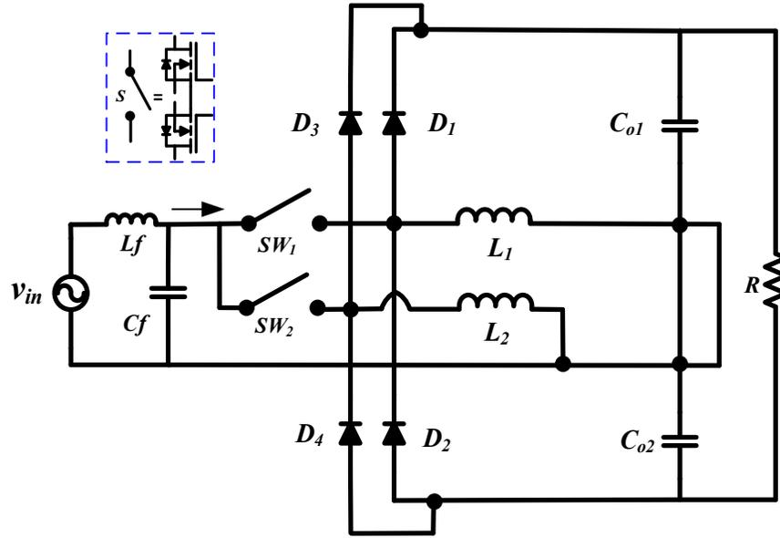
Fig. 5.1. Schematic of interleaved bridgeless buck-boost derived PFC converter
