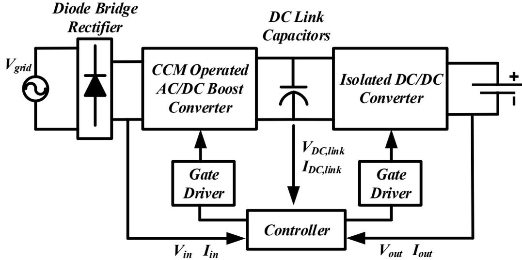
Fig. 1. 4. Block diagram of two-stage PFC technique
