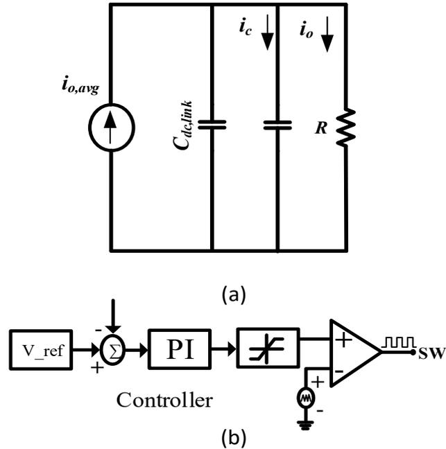
Fig. 4.7. (a) Equivalent circuit for small signal modelling. (b) Control Diagram.
