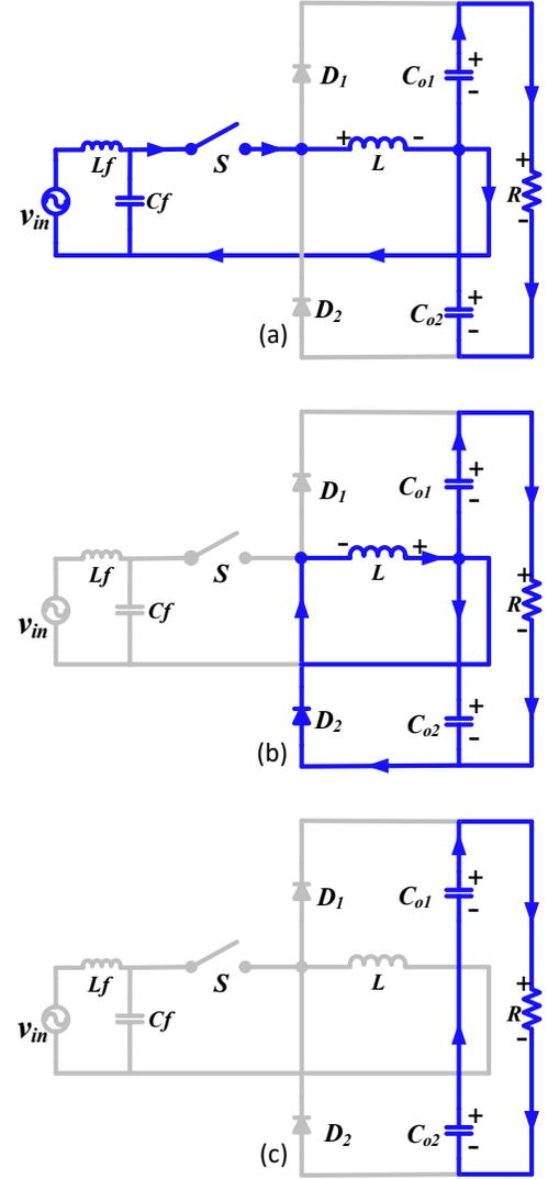
Fig. 3. 10. Equivalent circuits during positive half-cycle; (a) Mode-a; (b) Mode-b; (c) Mode-c.
