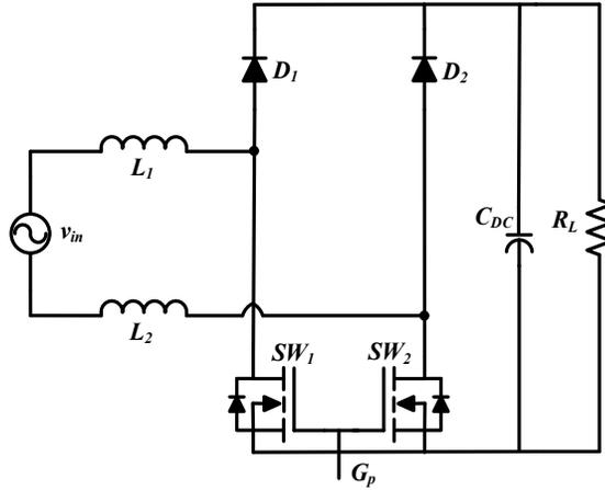
Fig. 3. 1. Bridgeless boost PFC converter
