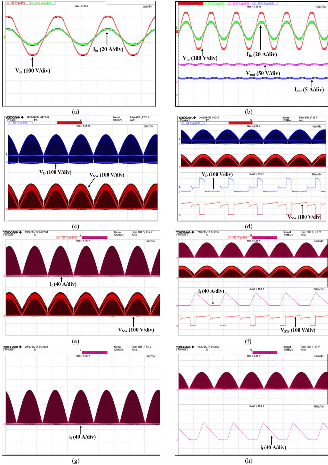
Fig. 2. 12. Experimental results (a) PFC operation at 1.0 kW. (b) Efficiency of single-cell converter (c) Single-cell diode and switch voltage stresses (d) Zoomed in version for single-cell voltage stresses on diode and switch. (e) Switch voltage and inductor current waveform. (f) Zoomed in version for switch voltage and inductor current waveform. (g) Inductor current waveform. (h) Zoomed in inductor current waveform at 1.0 kW.
