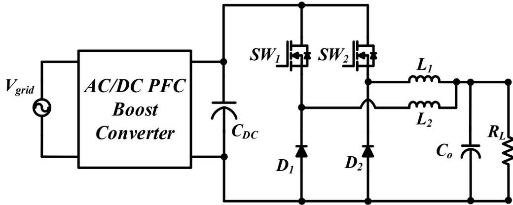
Fig. 2. 1. Two-stage interleaved buck converter
