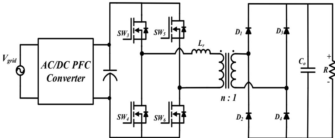
Fig. 4.2. Full bridge phase-shift PWM converter
