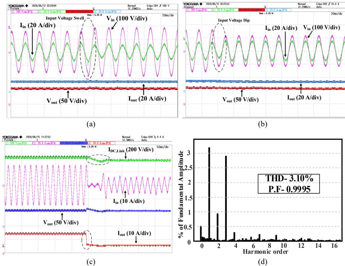
Fig. 4. 11. Converter response (a) Input voltage swell (b) input voltage dip (c) Load change from 100% to 20% (d) input current FFT at 1.0 kW
