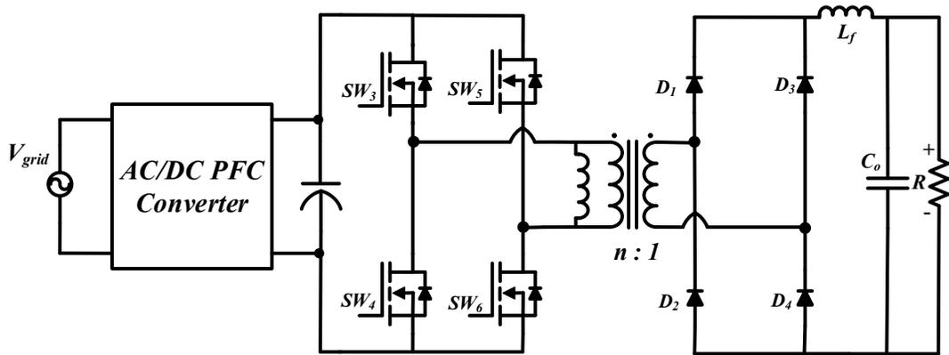
Fig. 4.1. Full-bridge isolated buck converter
