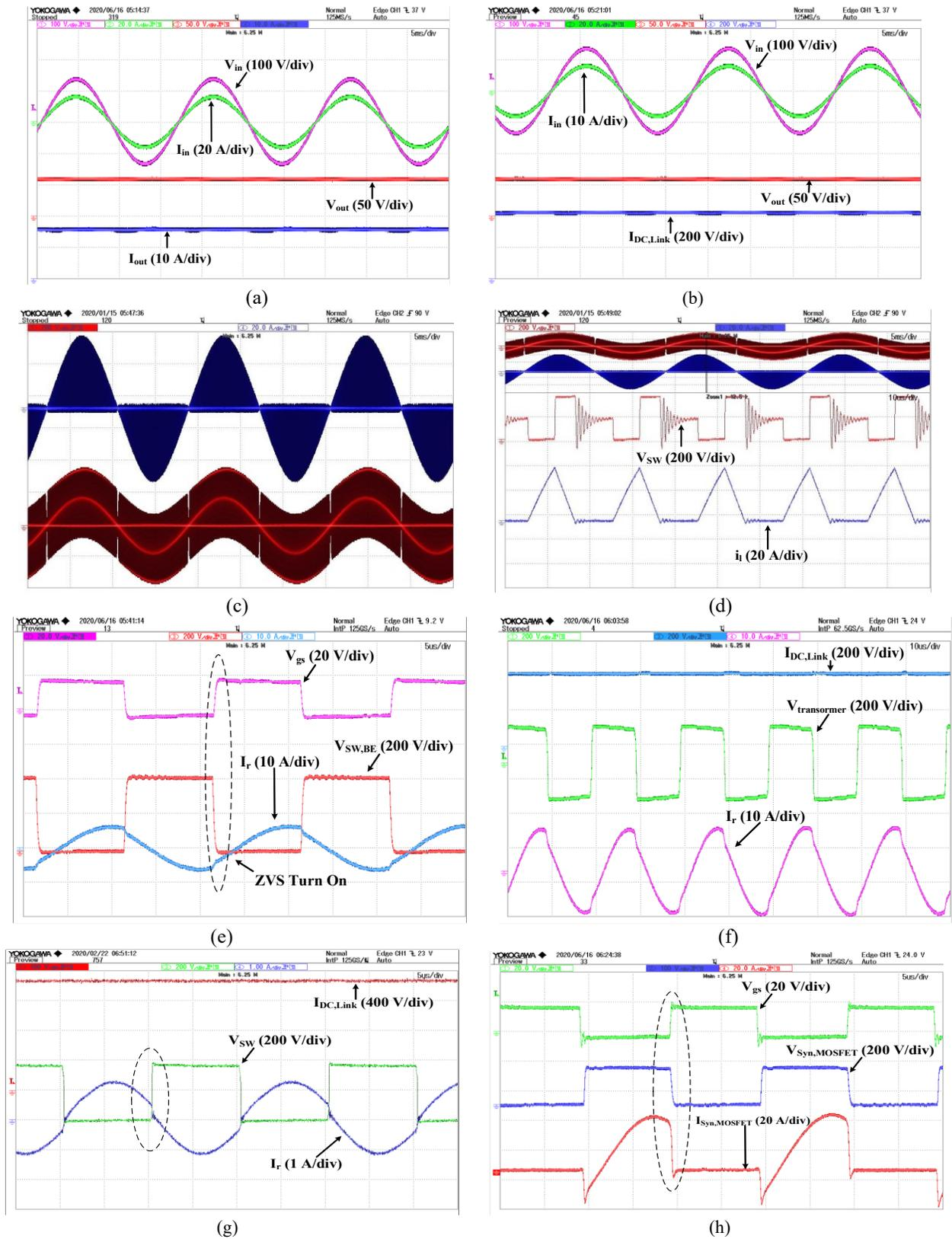
Fig. 4. 10. Experimental results (a) PFC operation at 1.0 kW (b) input PFC and DC link voltage. (c) Switch voltage and inductor current (d) ZCS turn-on of switch. (e) Switch voltage, gate and resonant current. (f) Transformer primary voltage and current. (g) Resonance operation at a low load. (h) Synchronous rectification operation.
