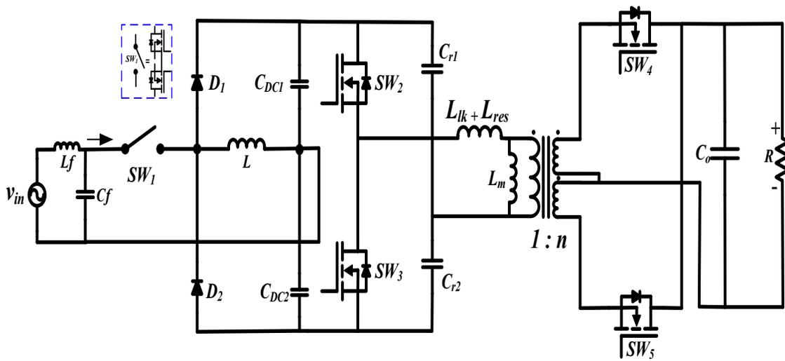
Fig. 4. 5. Proposed two-stage isolated EV charger configuration
