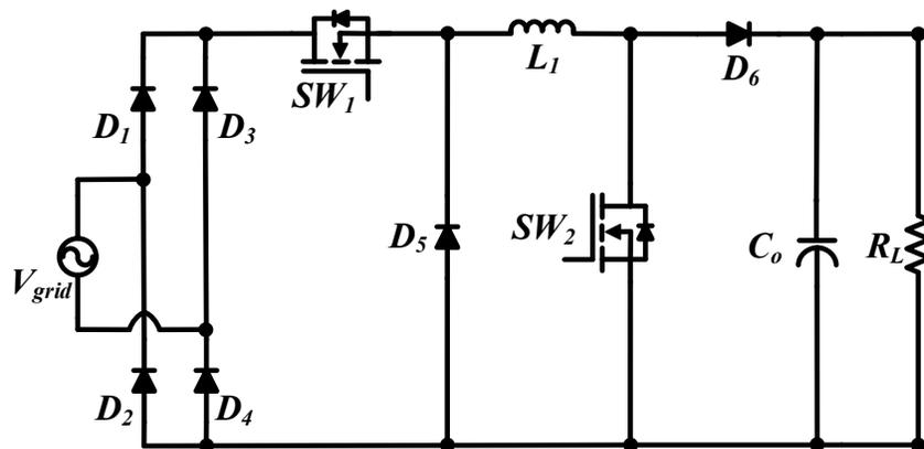
Fig. 2. 2. Non-inverting buck-boost converter
