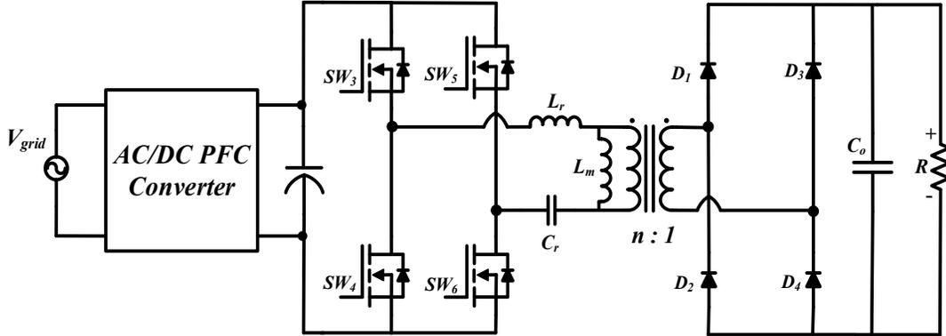
Fig. 4. 4. Full Bridge LLC Resonant Converter
