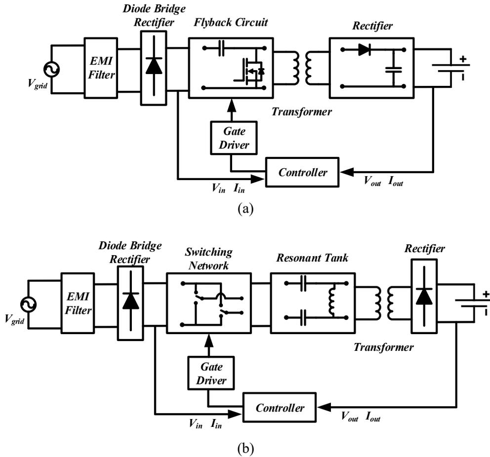
Fig. 1. 3. Single Stage (a) Isolated flyback converter; (b) half bridge isolated DC/DC resonate converter
