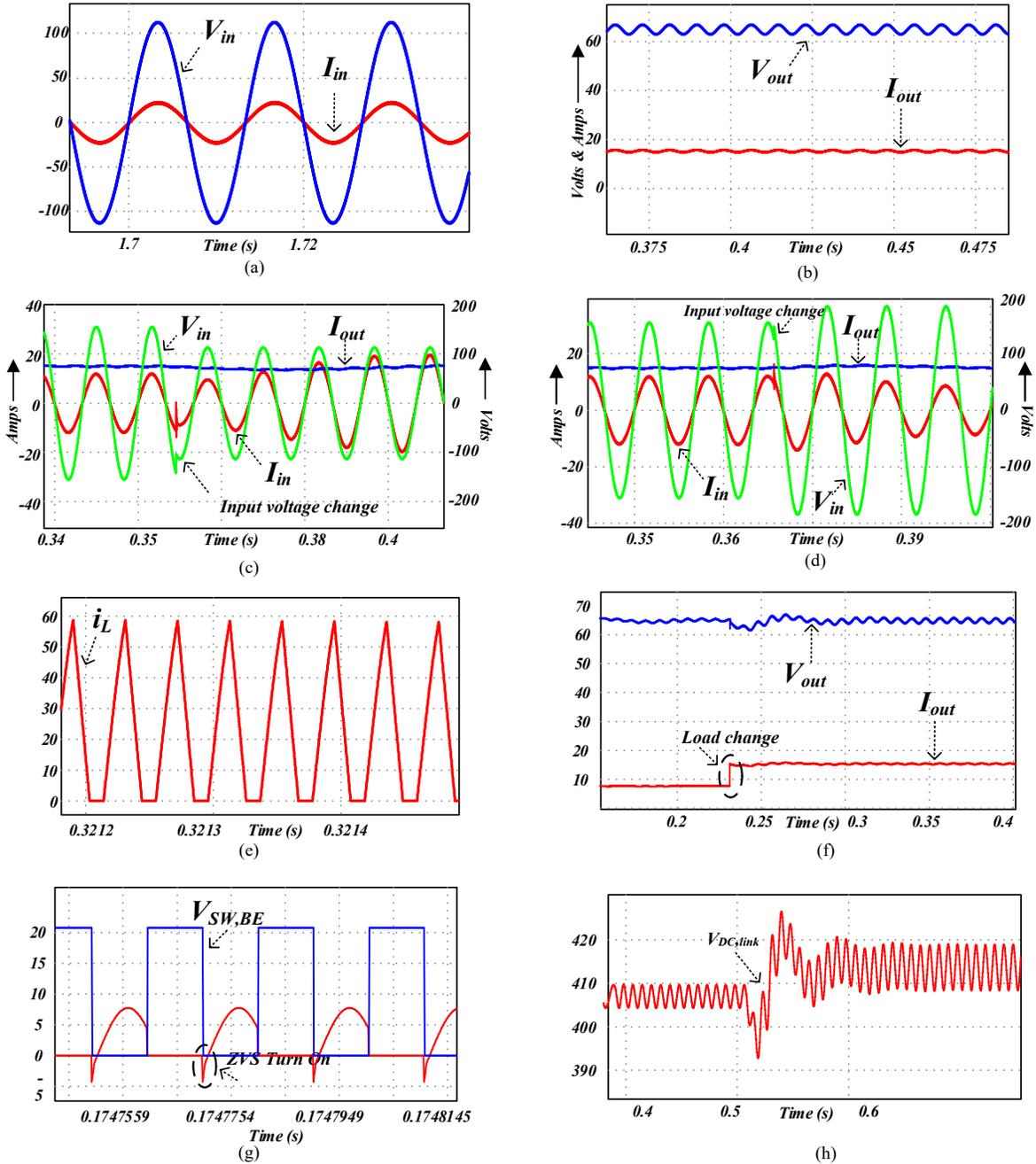
Fig. 4. 8. Simulation results (a) input voltage and current. (b) output voltage and current. (c) input voltage change from 110 V to 80 V. (d) input voltage change from 110 V to 130 V. (e) inductor current. (f) load change from 50% to 100% . (g) ZVS turn-on of half-bridge switch. (h) DC-link voltage variation during load change.
