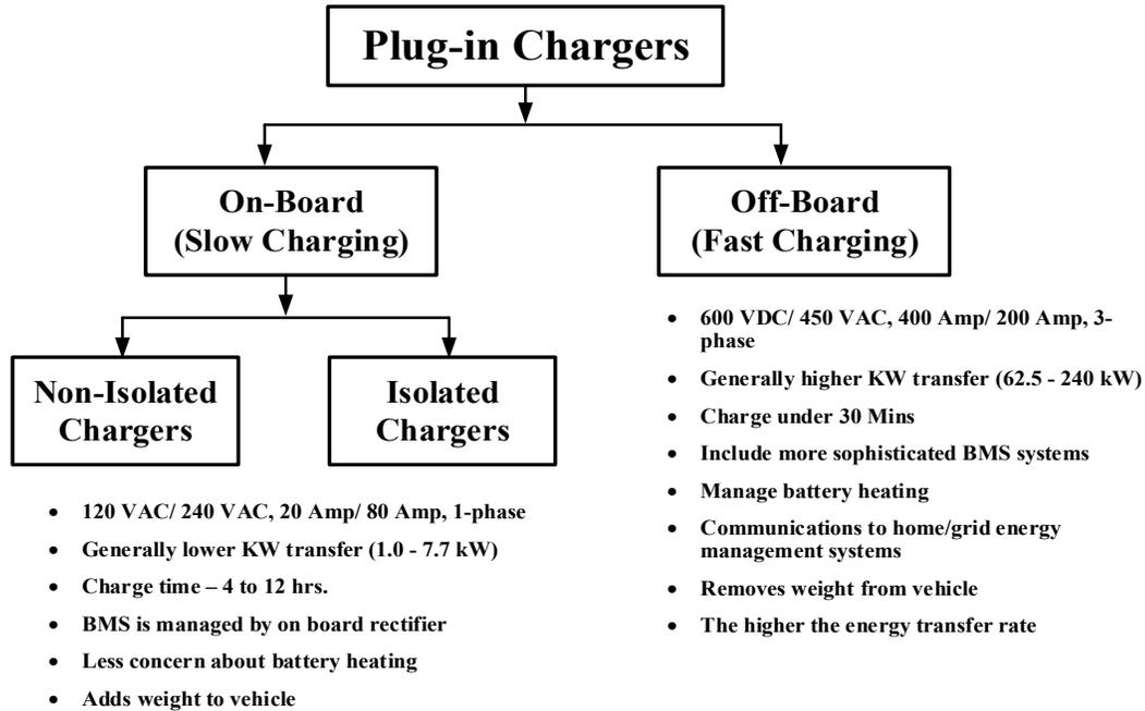
Fig. 1. 2. Classification of plug-in chargers
