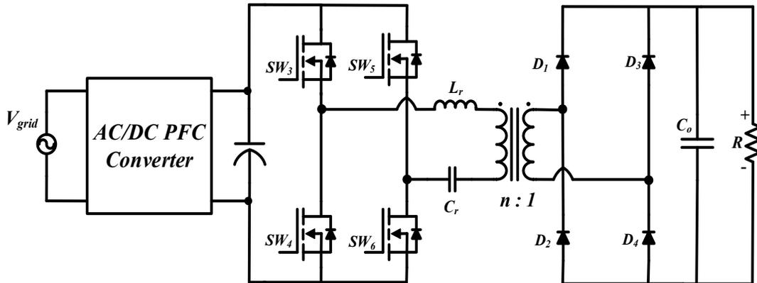
Fig. 4. 3. Full Bridge Series Resonant (FB-SRC) converter
