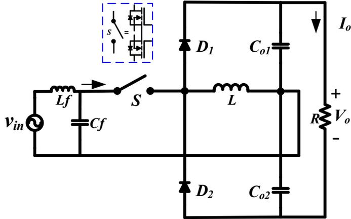
Fig. 3. 6. Proposed single-phase switched-mode bridgeless AC-DC buck-boost derived PFC converter
