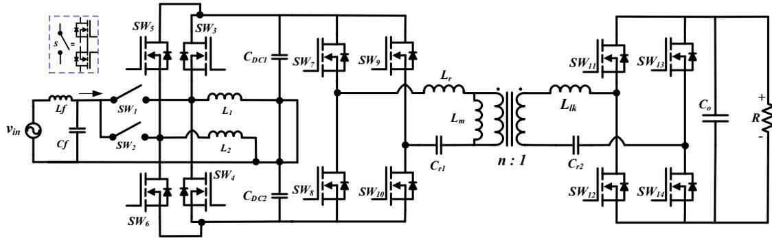
Fig. 5.2. Schematic of Interleaved Bridgeless PFC and Full-Bridge LLC Resonant converter
