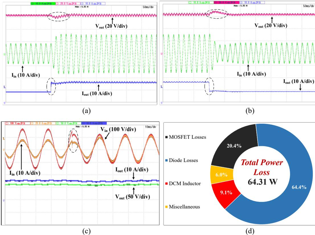
Fig. 2. 14. Converter response (a) load change from 500W to 1.0 kW, (b) load change from 1.0 kW to 500 W, (c) input voltage swell, (d) Power loss distribution of converter at 1.0 kW.
