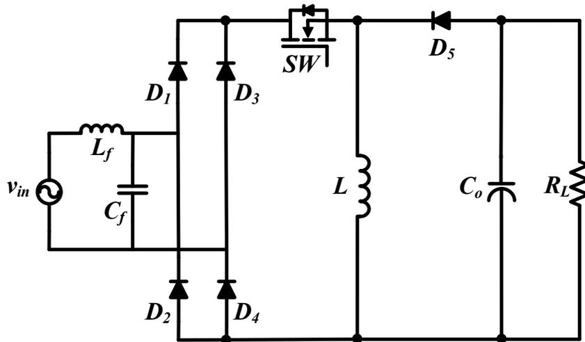
Fig. 2. 5. Non-isolated single-cell buck-boost converter
