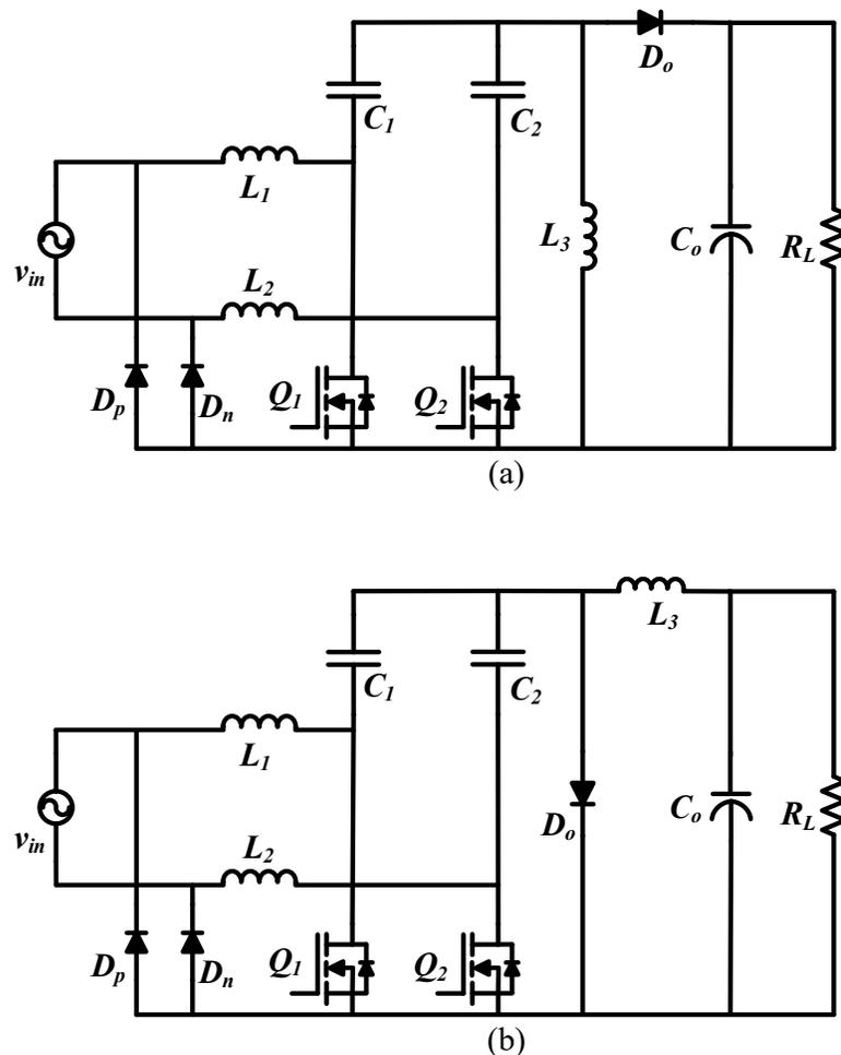
Fig. 3. 5. Converter configuration (a) Bridgeless Sepic, (b) Bridgeless Cuk
