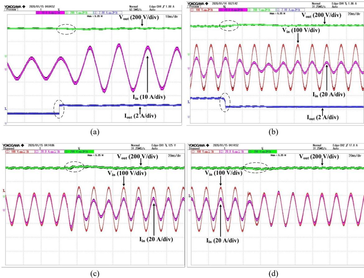
Fig. 3. 16. Converter response (a) load change from 500W to 1.0 kW; (b) load change from 1.0 kW to 500 W; (c) input voltage swell. (d) Input voltage dip
