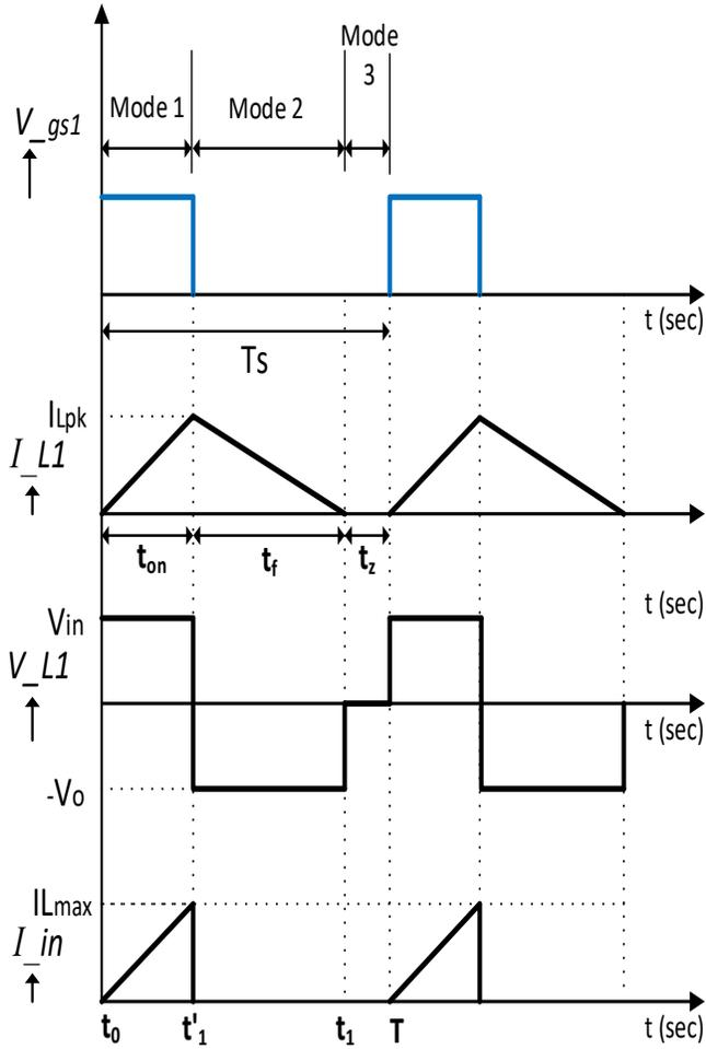
Fig. 2. 7. Waveforms for one switching cycle
