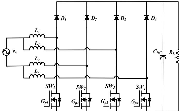
Fig. 3. 3. Bridgeless Interleaved Boost PFC converter
