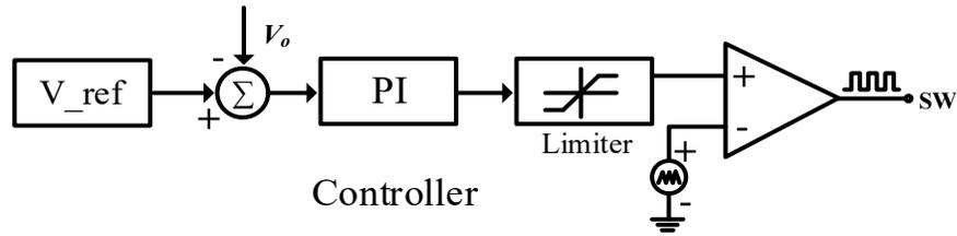
Fig. 3. 7. The control circuit for the proposed converter.
