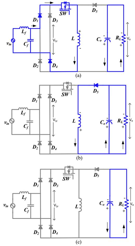
Fig. 2. 8. Equivalent circuits during positive half-cycle; (a) Mode-1; (b) Mode-2; (c) Mode-3.
