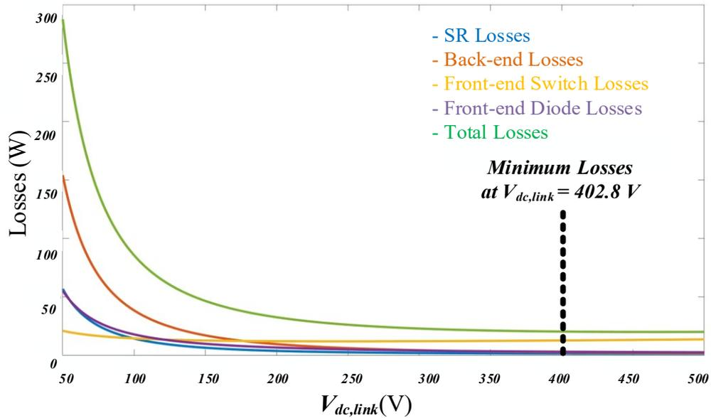
Fig. 4. 6. Calculated Losses according to various DC-Link Voltages.
