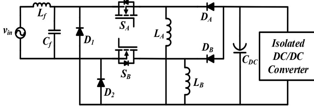
Fig. 3. 4. Single phase bridgeless buck-boost PFC converter
