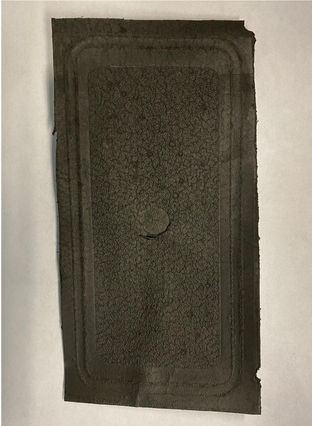
Figure 22 Photo of the conductive membrane surface. Note the markings left by the compressed seal around the outer edges of the membrane surface, indicating no water losses. This MWNT Carbon Buckypaper was backed by the Ultrafiltration membrane. This conductive surface came in direct contact with the wastewater and acted as the anode in electrochemical processes
