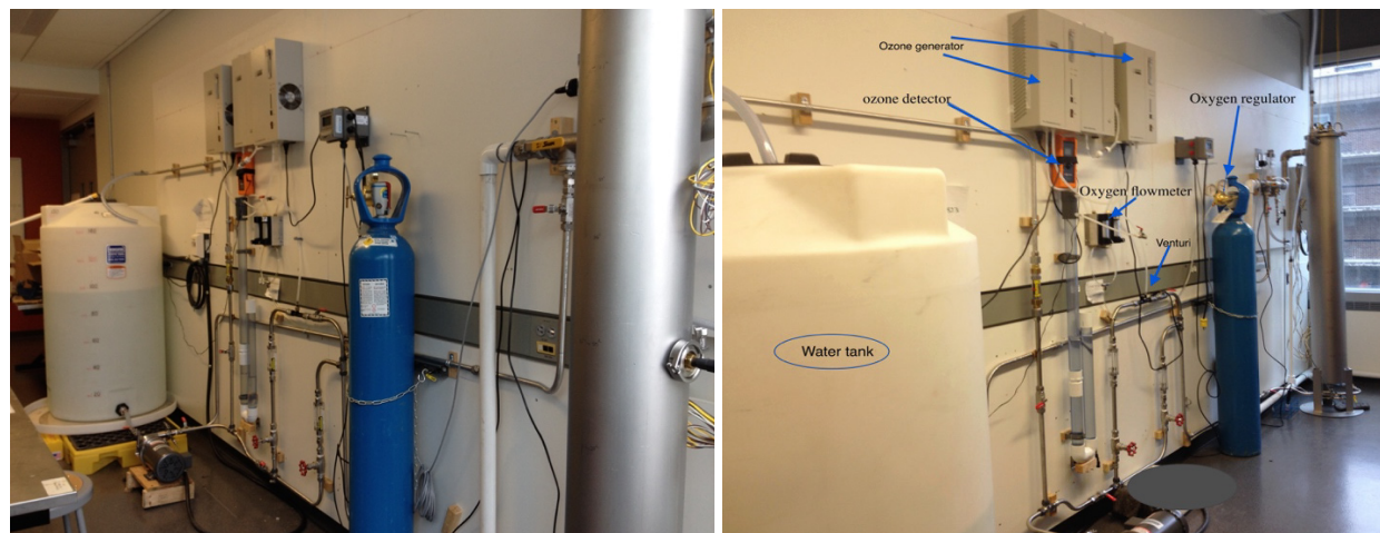
Figure 3.6. UV/O 3 -H 2 O 2 AOP experimental pilot plant setup
