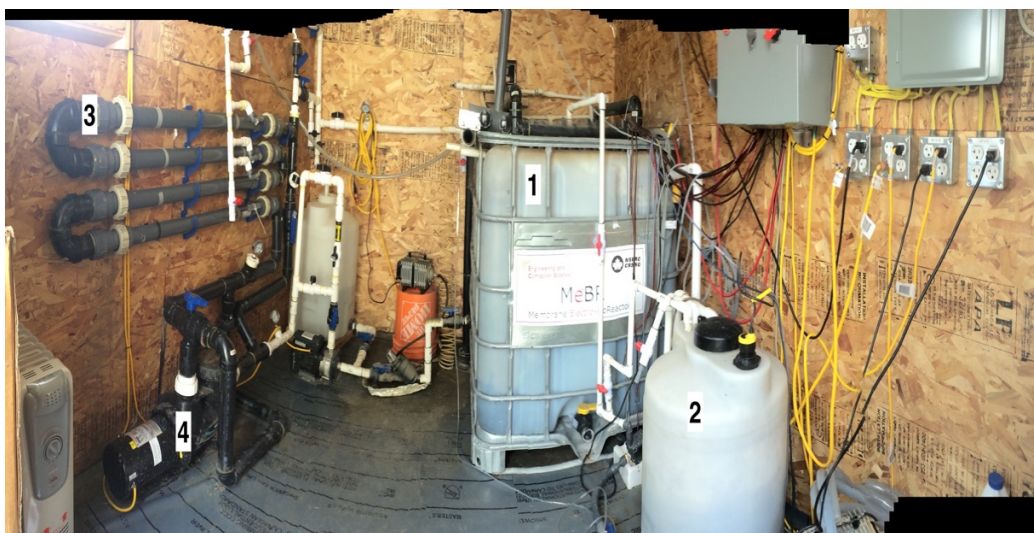
Figure 3.7. Pilot MEBR system in a self-standing cabin (Elektorowicz et al. 2017) 1- Elector bio- reactor 2- Wastewater input 3- Membrane 4- Pump
