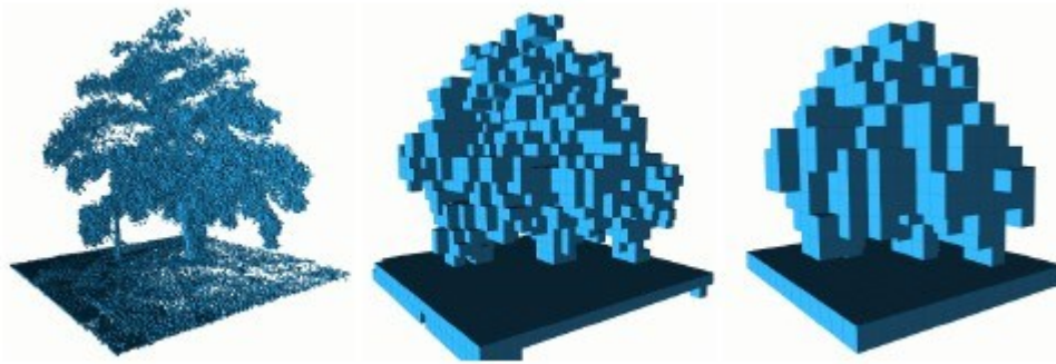
Figure 2.2 By limiting the depth of a query, multiple resolutions of the same map can be obtained at any time. Occupied voxels are displayed in resolutions 0.08m, 0.64m, and 1.28m.
