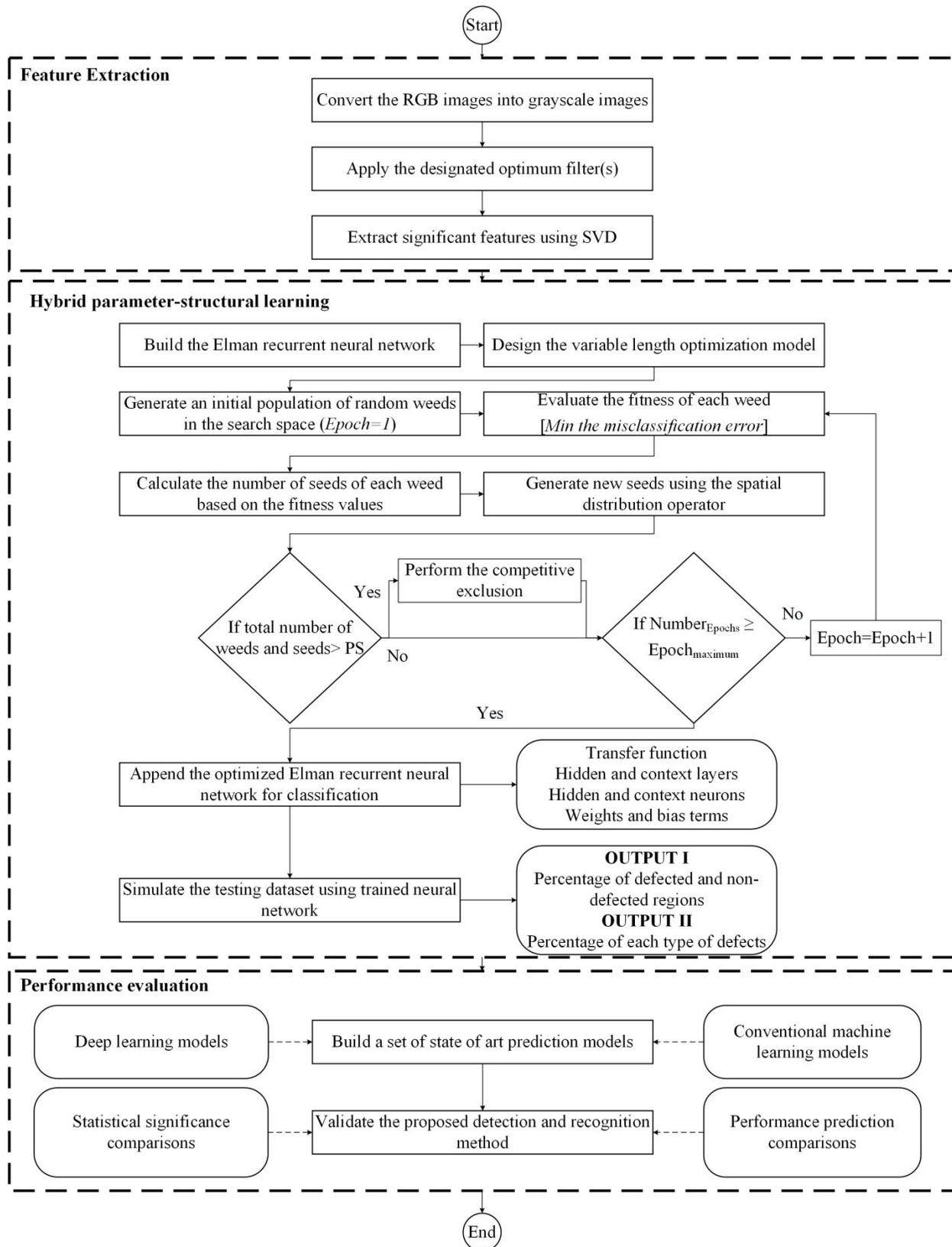
**Figure 3.4: Flowchart of the developed defects' detection and recognition method**
