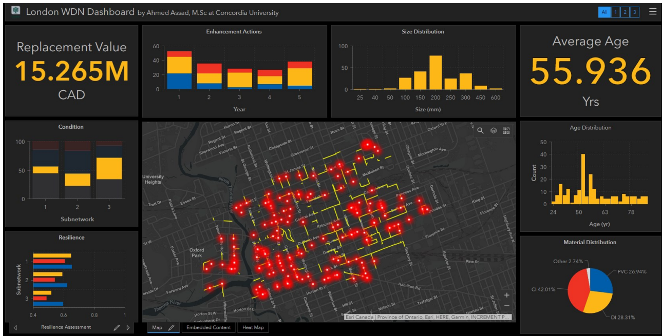
Figure 4-28: Segments in Poor Condition View of London WDN Dashboard
