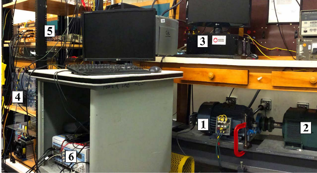
Fig. 2.12: Experimental setup. (1) Test SynRM. (2) dynamometer. (3) Real-time controller. (4) Inverter. (5) Sensors. (6) Data Acquisition System.
