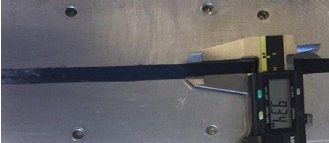
Figure 29 Towpreg expansion over a high compaction Force
