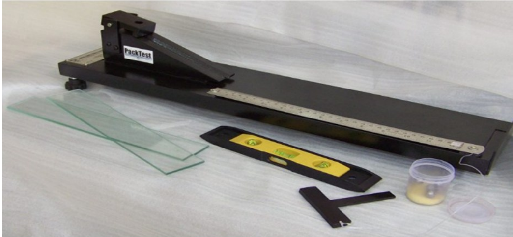
Figure 2 Rolling ball tackiness measurement method
