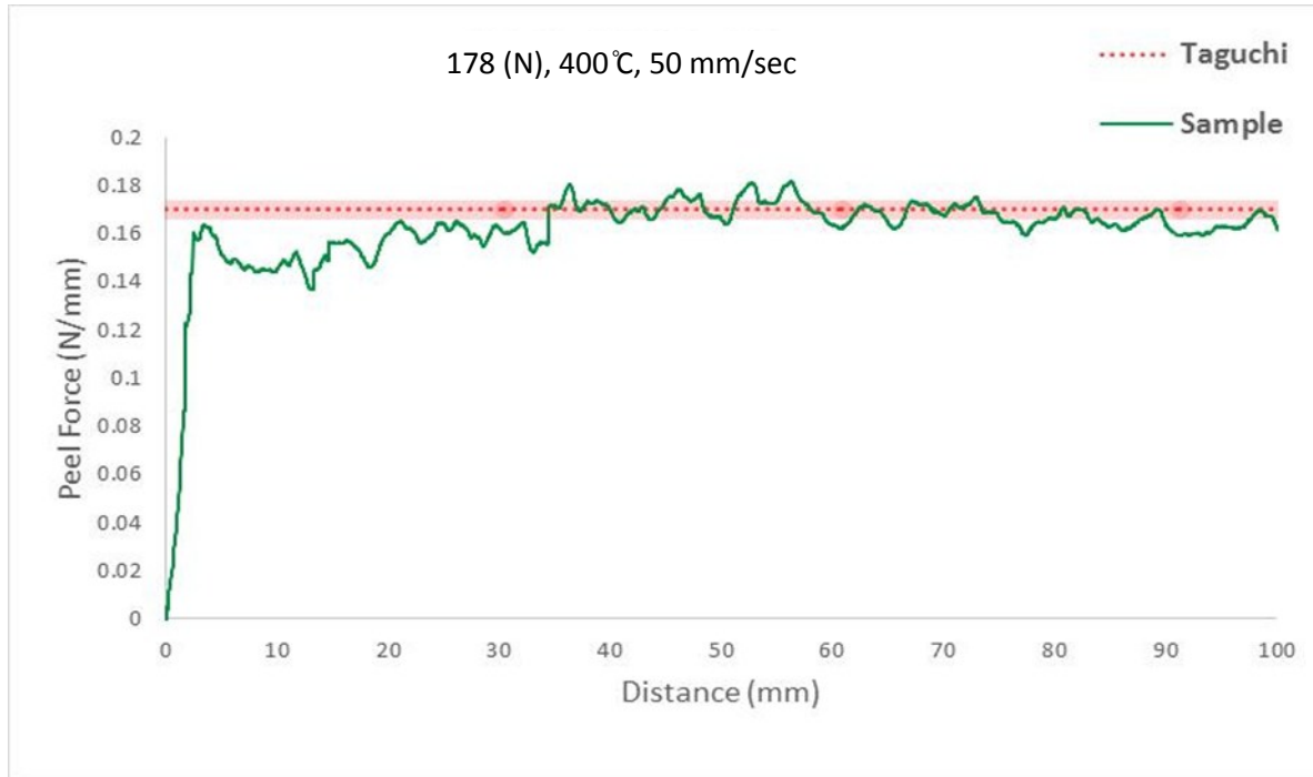
Figure 21 Taguchi prediction vs real test
