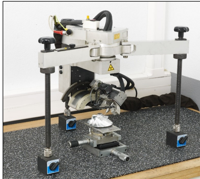
Figure 18: Schematic image of a residual stress analysis device by x-ray diffraction - Stresstech Xstress 3000 G2R (EUROPE TECHNOLOGIES SONATS, 2020)
