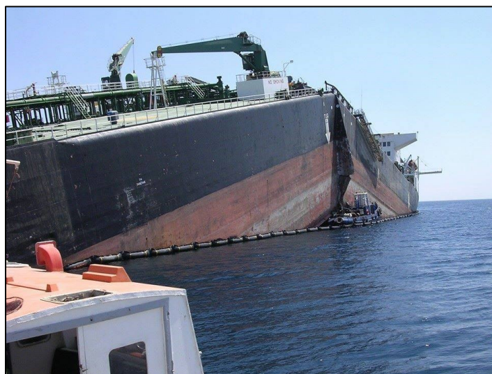
Figure 4: Schematic picture of a recent propagation of cracks incident in marine industry – Courtesy: FIVEOCEANSALVAGE / Hasan Saad
