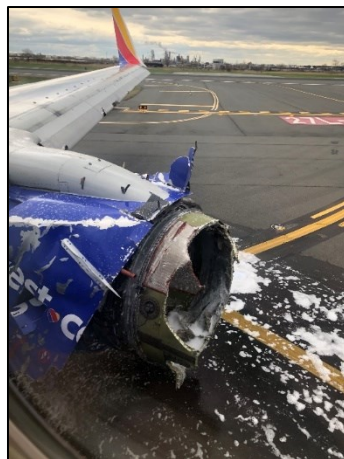
Figure 2: Schematic illustration of a recent metal fatigue incident in aerospace industry reported by American National Transportation Safety Board (NTSB) back in August 2016 – Courtesy: NTSB NEWS AND EVENTS
