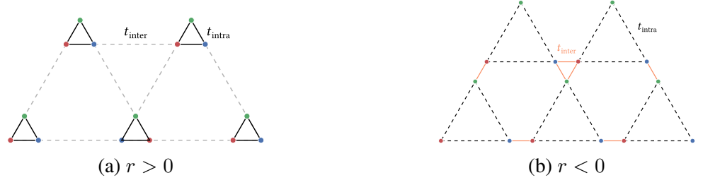
Figure 25: Increasing t_{intra} in r > 0 and increasing t_{inter} in r < 0 have the same effect on the energy.
