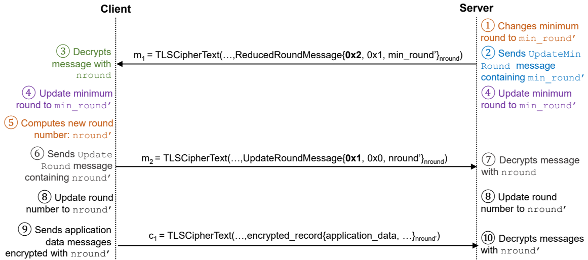
Figure 7: Reduced-round Round Configuration Update on TLS 1.3.
