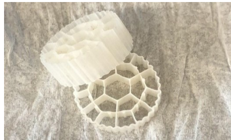
Figure 3-1 Image of plastic media used in this study
