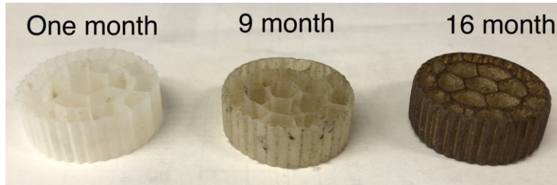
Figure 4-26 Media biofilm development throughout the study
