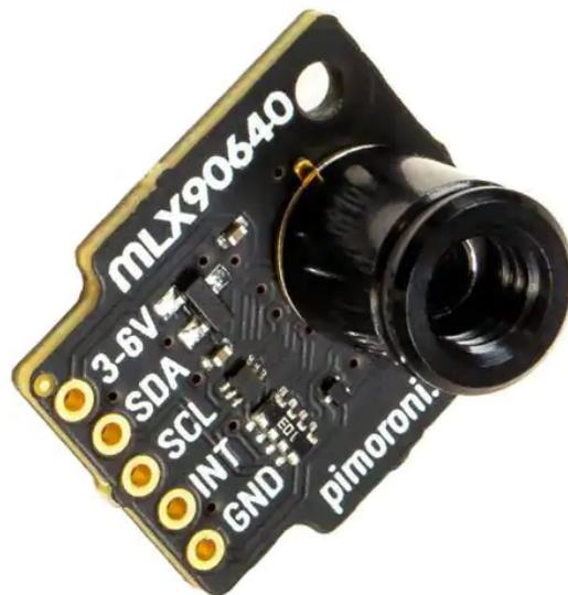
Figure 3.4: MLX90640, 32\*24 pixels thermal camera
