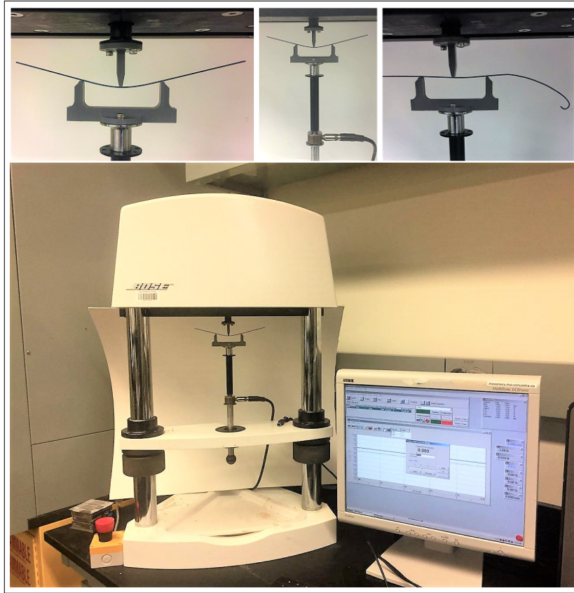
Figure 8: Three point bending test setup
