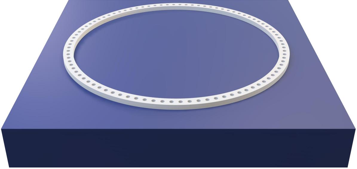
Figure 14: A photonic crystal ring resonator composed of a standard ring resonator with an overlying photonic crystal lattice.
