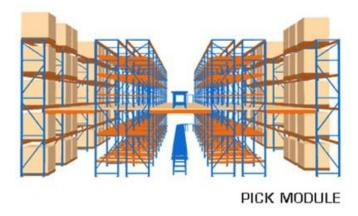
The conveyor system collects cases and totes from 10 pick modules composed of a total of 34 levels. The conveyor operates inside each level and the cases are stored on both sides of the conveyor. These items are further consolidated on a single line through multiple merges and channelled to their sorters according to their designated store. Example of a merge is provided in Figure 2 (*Lineshaft Roller Conveyor Merges*, n.d.).
