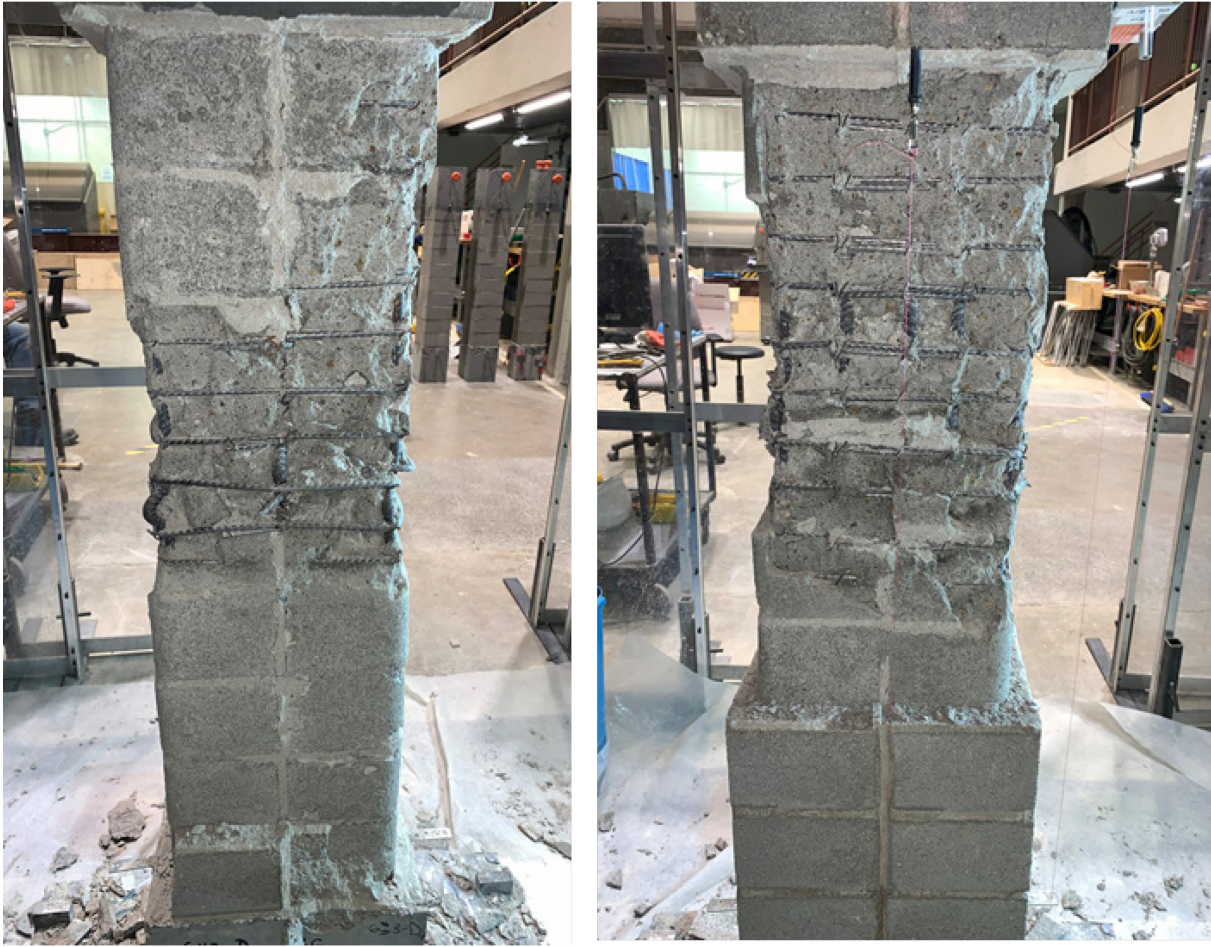
Figure A.23 Typical final damage state at 75% strength degradation of rectangular RMBEs with 6#3 and 12#3 vertical steel bars
