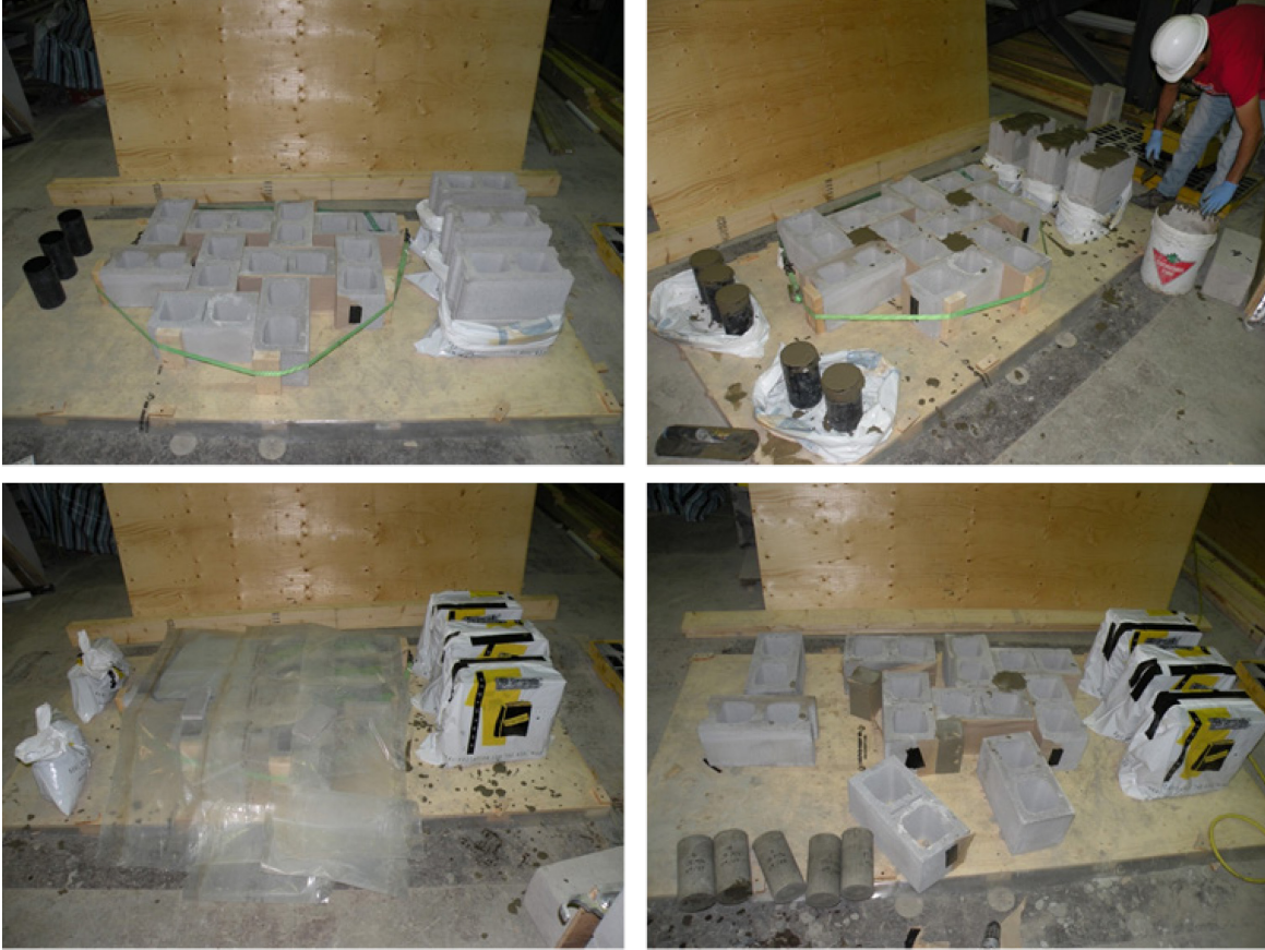
Figure A.2 Typical grouting of masonry prisms and sampling of block moulded grout and cylinders
