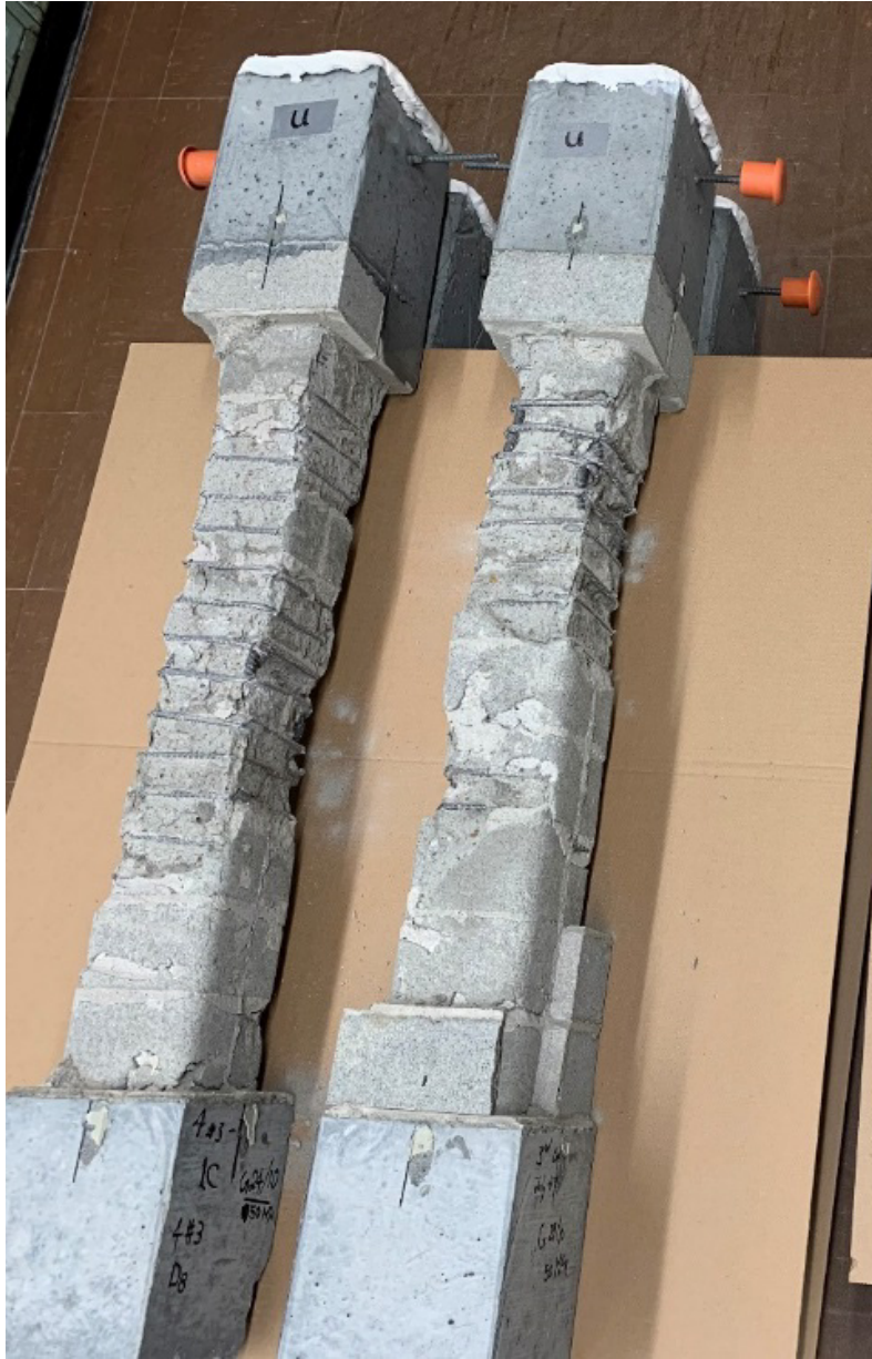
Figure A.24 Typical final damage state of square RMBEs
