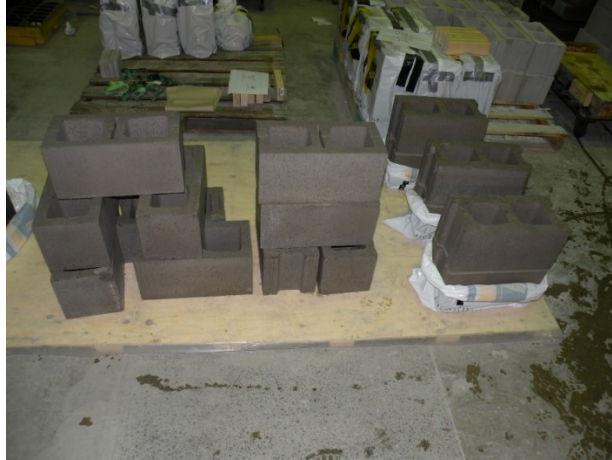
Figure A.3 Pre-wetted masonry prisms and masonry blocks before grouting
