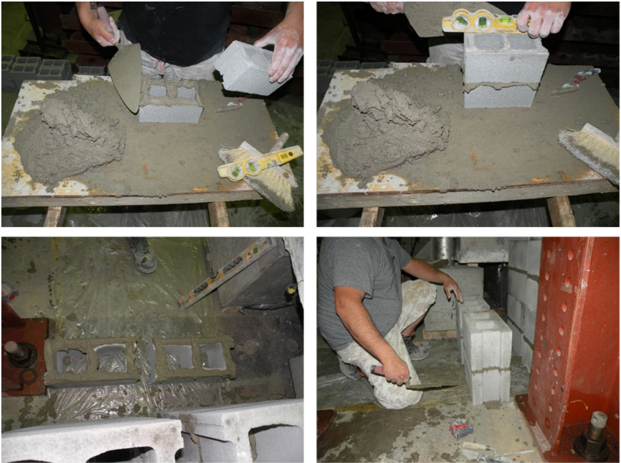
Figure A.1 Typical construction of half-scale and full-scale masonry prisms
