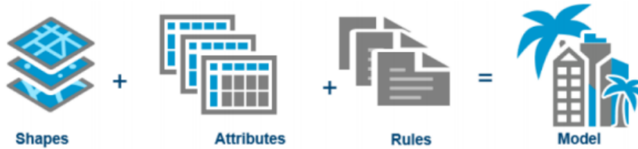
Figure 39: 3D city modeling workflow in ArcGIS CityEngine using the contribution of 2D model, supplementary attributes, and predefined rules
