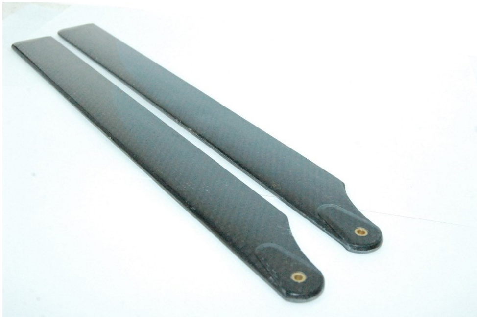
Figure A.2 Rotor blades for drone made from epoxy-graphite composite material [53]
