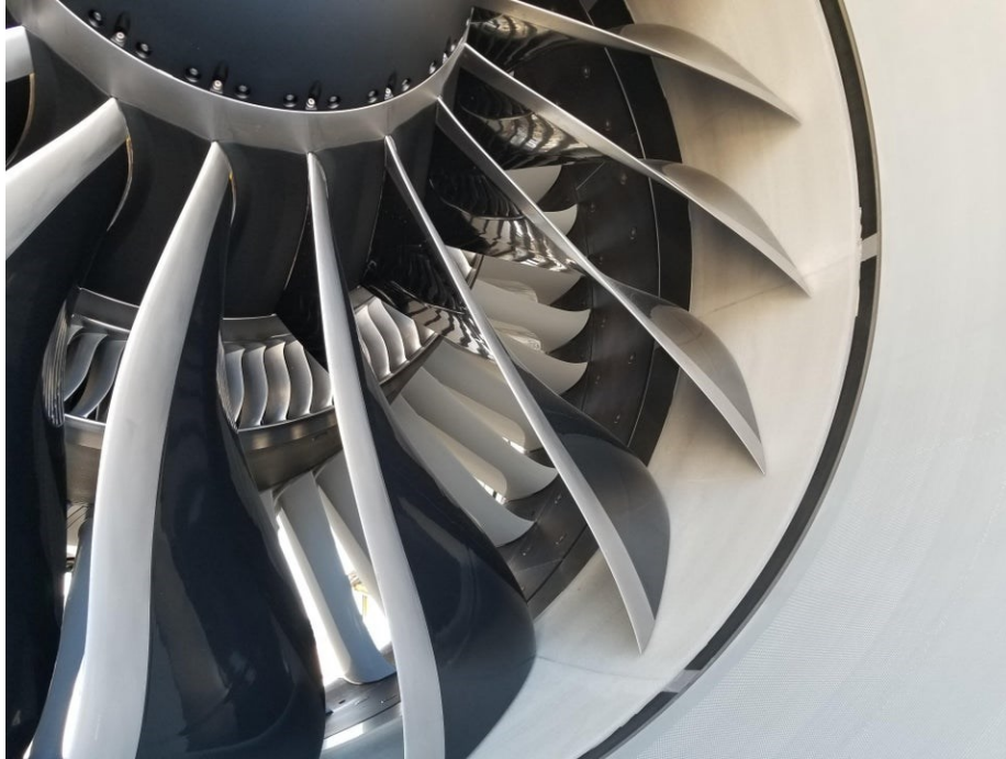
Figure A.1 Turbine blades for aircraft engines made up of composite material made up of composite material [54]
