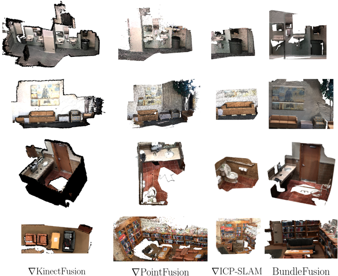
Figure 20: Qualitative results of running several differentiable SLAM systems ( \nabla KinectFusion, \nabla PointFusion, and \nabla ICP-SLAM [9]) on the ScanNet [11] dataset sequences. Due to GPU memory constraints, only parts of the scene were reconstructed. Reconstruction results of BundleFusion [12] are also shown for reference. Figure courtesy of \nabla SLAM [9].
