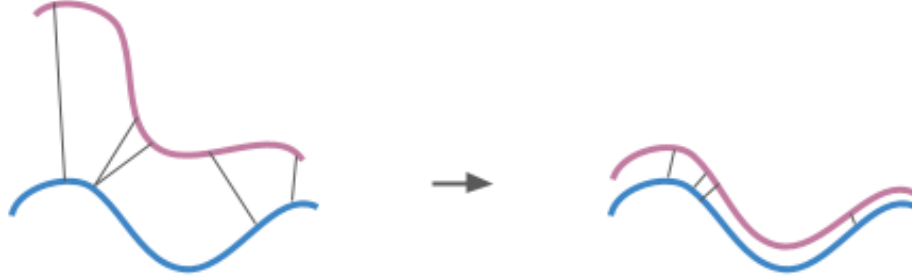
Figure 14: Iterative closest point algorithm. Minimizing the error function moves the source curve (pink) towards the target curve (blue).
