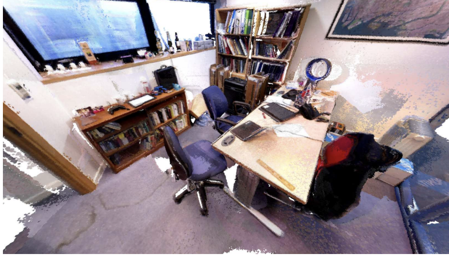
Figure 13: An example surfel-based map reconstruction using dense visual SLAM. Figure courtesy of [2].
