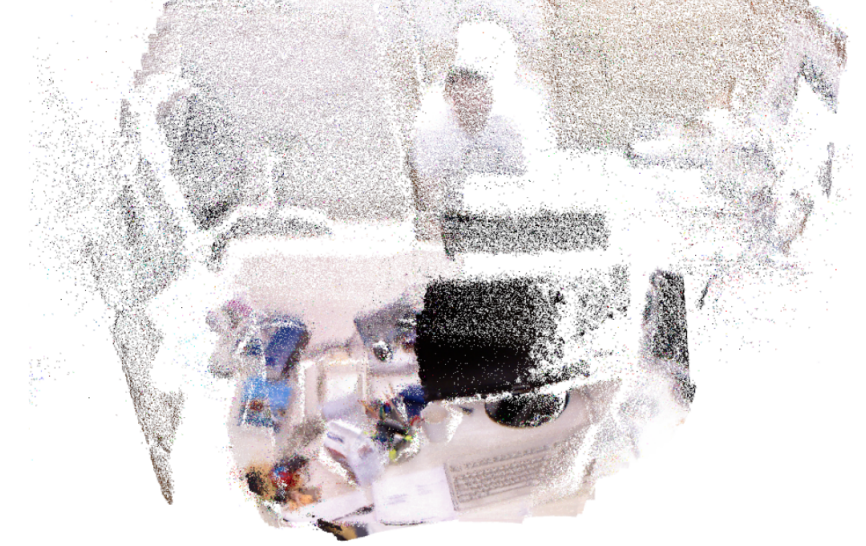
Figure 19: Reconstructed pointcloud by running \nabla ICP-SLAM on a sequence from the TUM RGB-D dataset [10]. Figure courtesy of \nabla SLAM [9].
