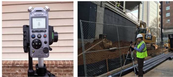
(a) Microphone placing at the jobsite for collecting audio files
