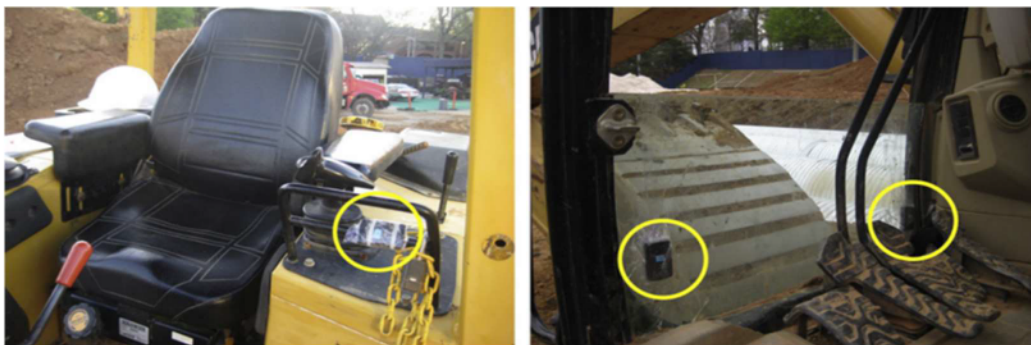
(a) GPS sensor mounted on the equipment
