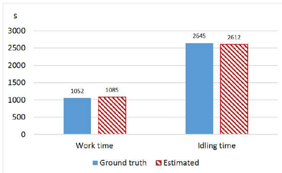
Figure 5-3 Estimated excavator idling and working time with ground truth (Case Study 1)
