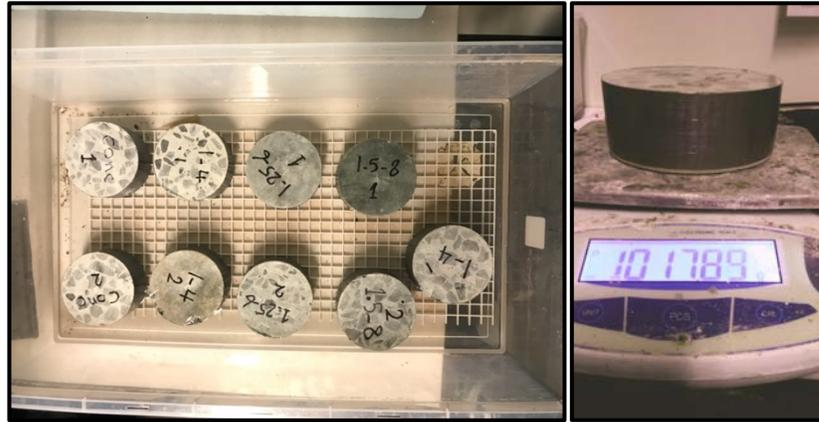
**Fig. 3.16 Water absorption test method.**
