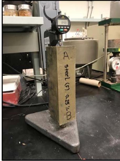
**Fig. 3.15 Shrinkage micro-strain test setup.**
