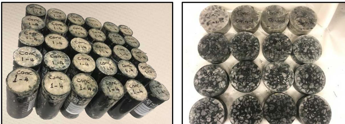
**Fig. 5.1** AAS and OPC prepared concrete specimens.
