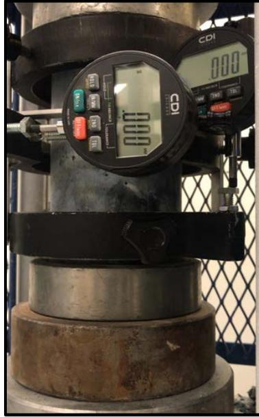
**Fig. 3.14 Modulus of elasticity test setup.**
