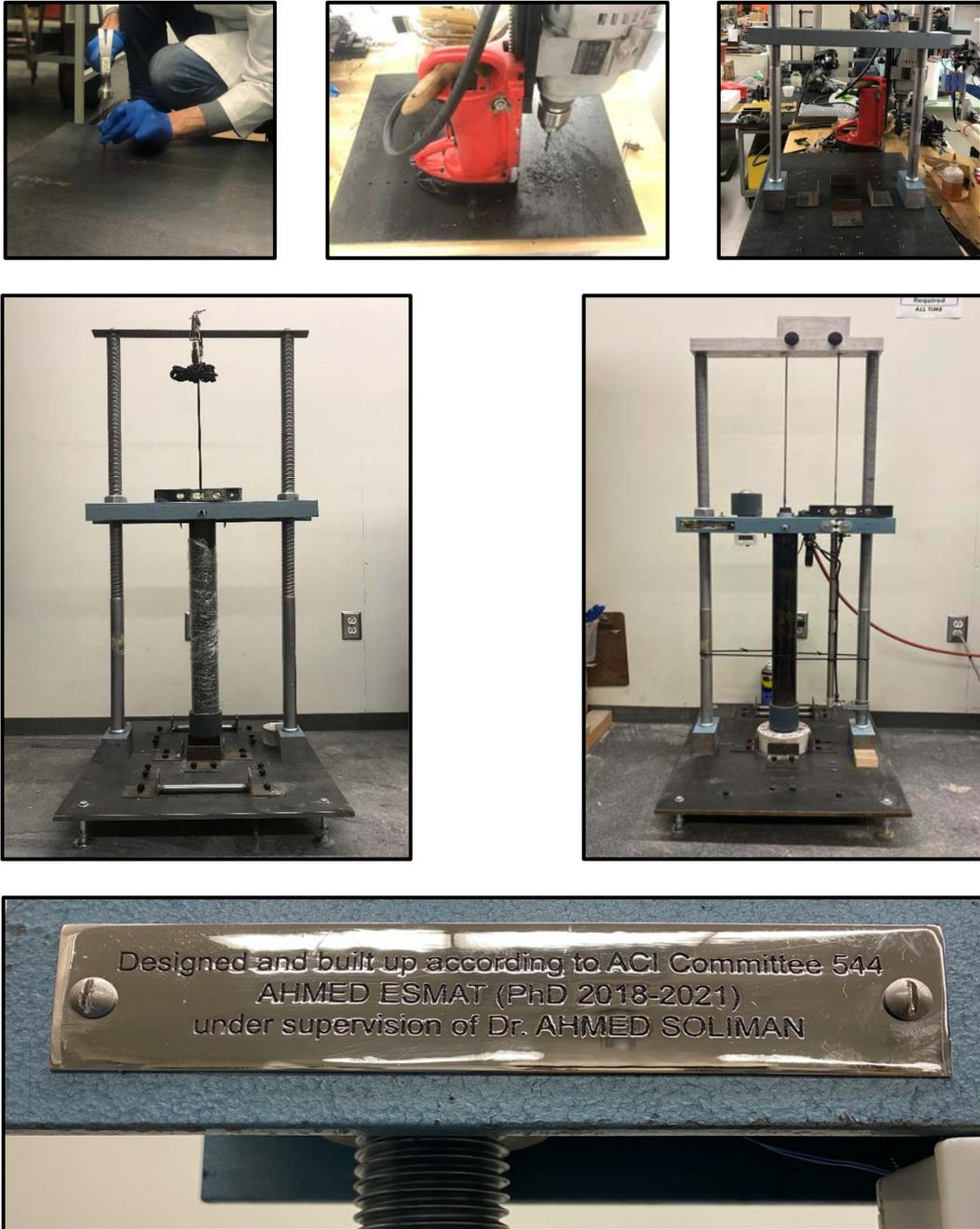
Fig. 3.19 Drop weight impact test machine.
