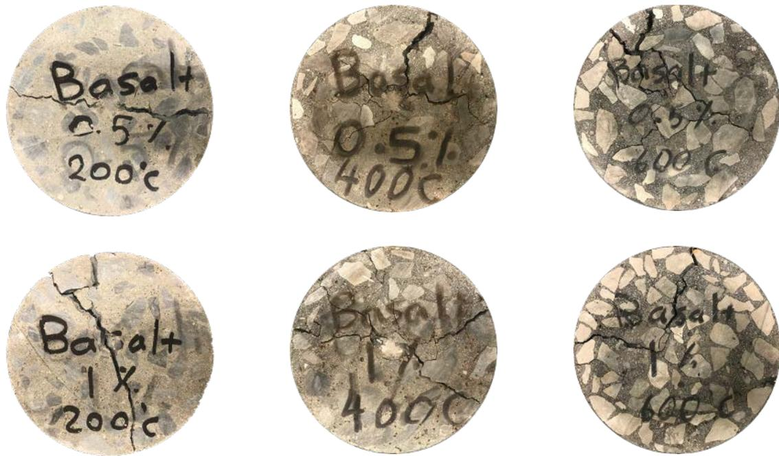
**Fig. 7.28 Failure of AAS basalt fiber concrete with different fiber contents.**
