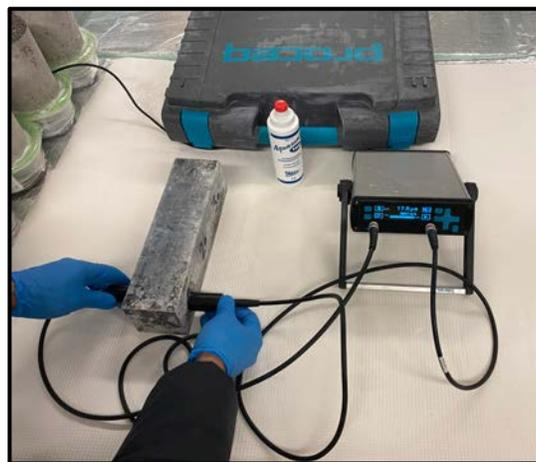
**Fig. 3.17 Ultra-sonic pulse velocity (USPV) test.**
