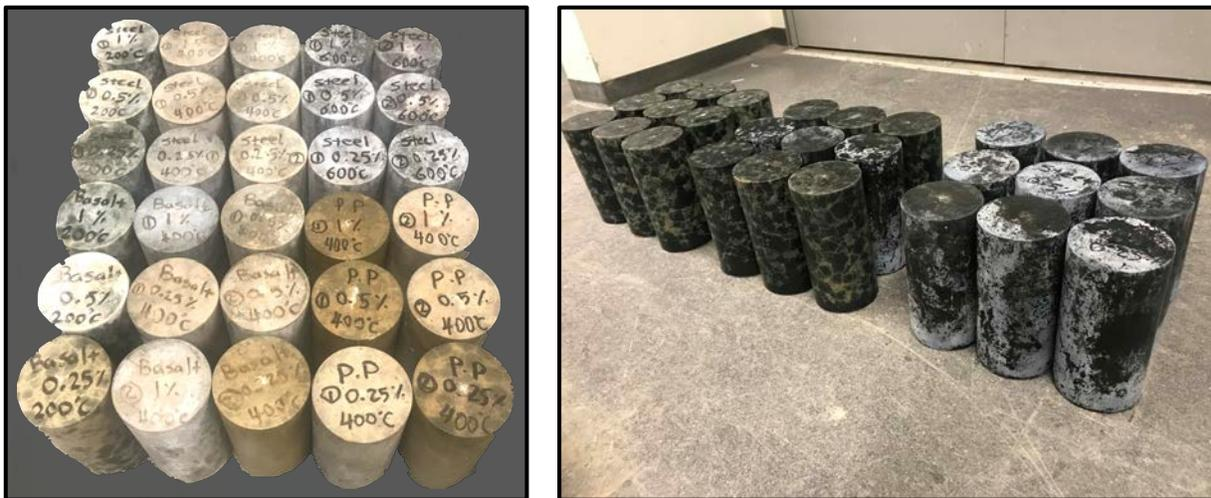
**Fig. 7.1** Cylinder fibre reinforced AAS concrete specimens before and after exposure to elevated temperatures.
