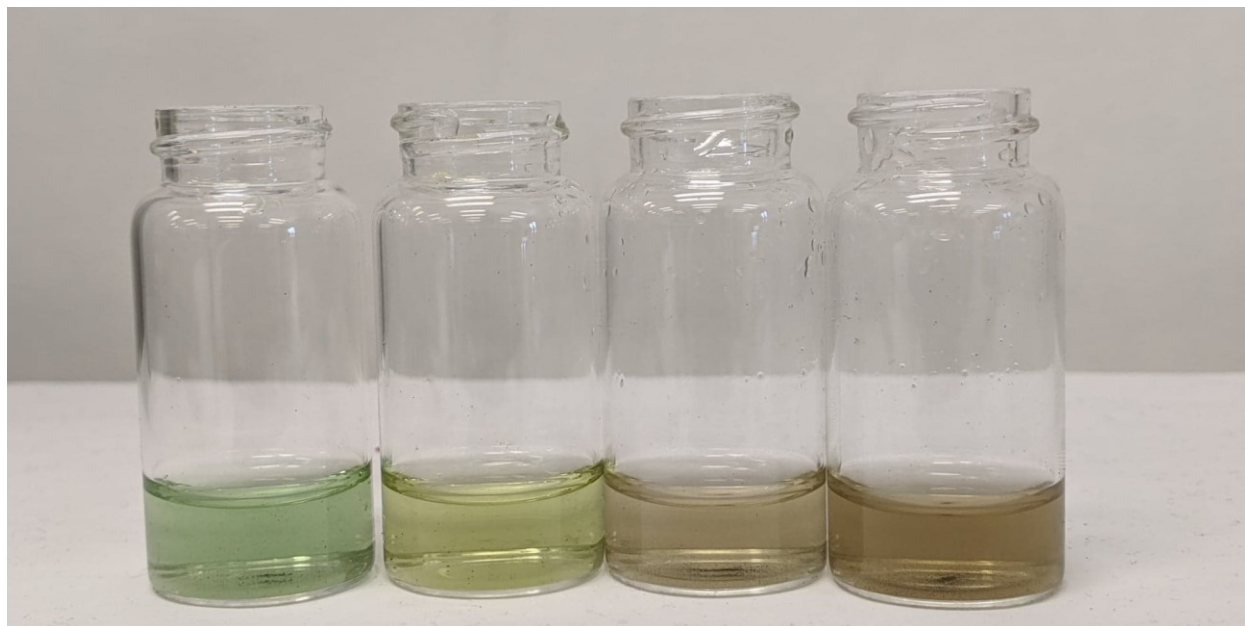
Figure S2.1 Colloidal dispersions of CD-1, CD-2, CD-4 and CD-8 (left to right) representing 1, 2, 4 and 8-hour reaction times, respectively. The colour of the carbon dot dispersion changes from green to brown suggesting an increase in carbonization with increasing synthesis time.
