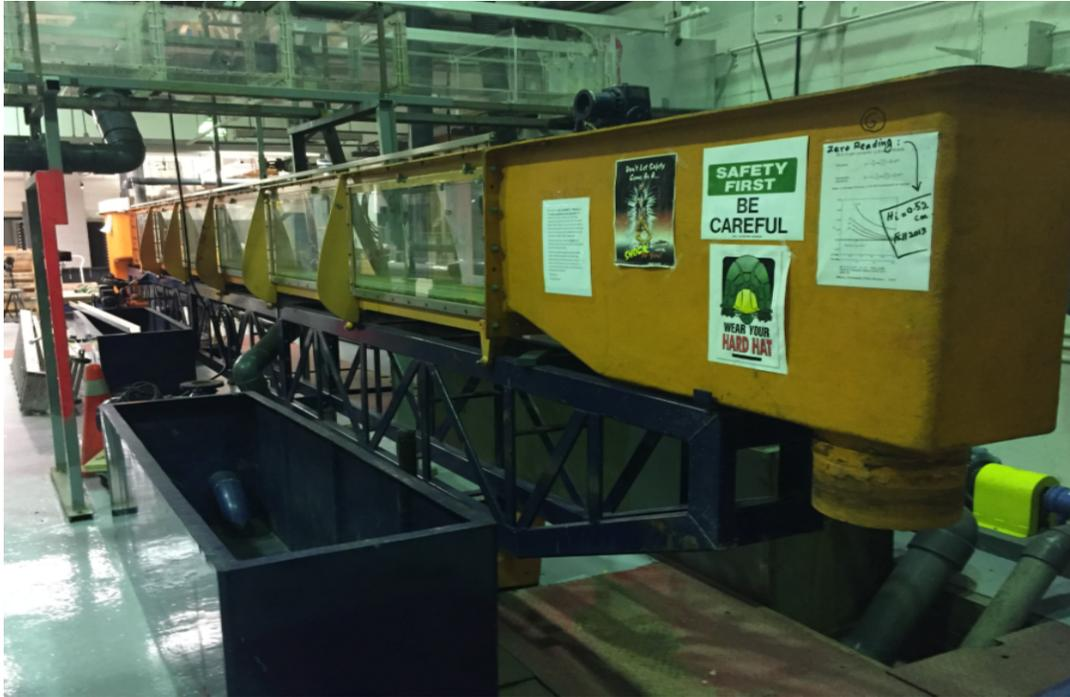
Figure 3-2 Photo of the hydraulic flume in the Water Resources Laboratory at Concordia University. The flume was used for experiments of siphon flow in this study.
