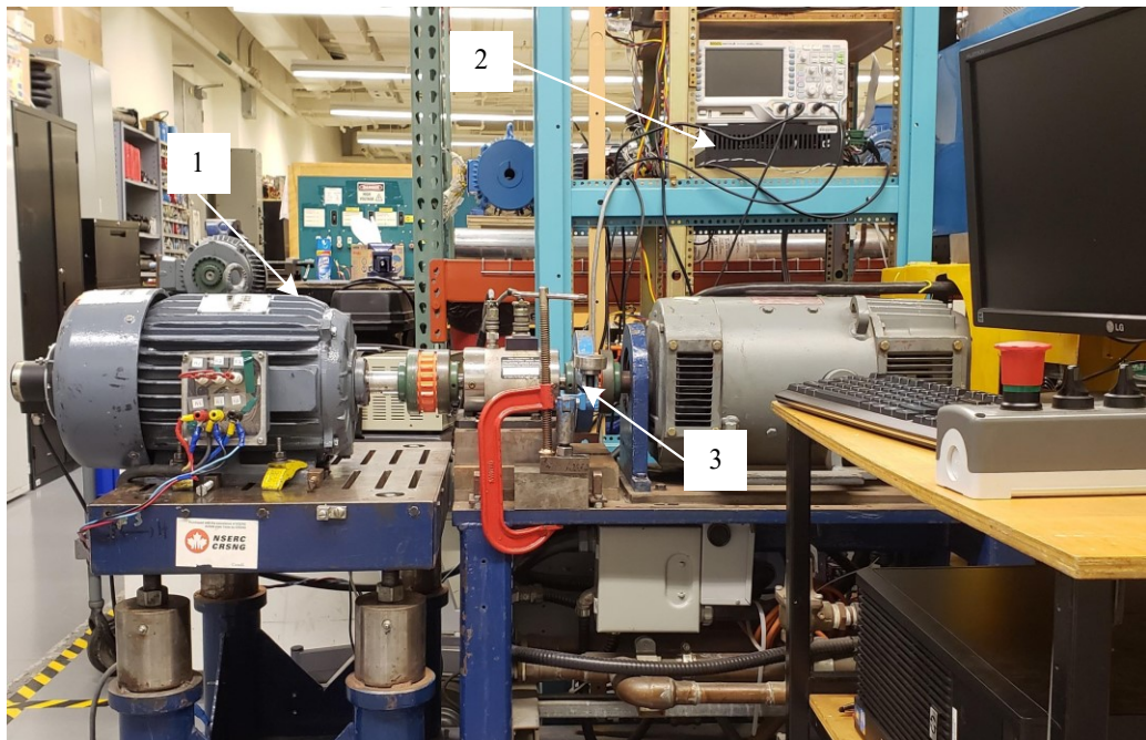
Fig.4-4. VF-PMSM test setup. (1) VF-PMSM (2) Real-time simulator (3) Rotor lock mechanism.
