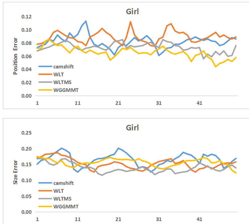
Figure 3.10: Performance (girl) of camshift, WLT, WLTS and WGGMMT in terms of position and size error
