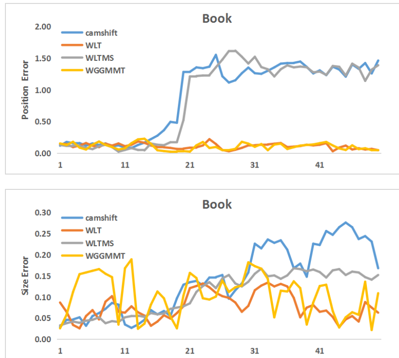
Figure 3.9: Performance (book) of camshift, WLT, WLTS and WGGMMT in terms of position and size error
