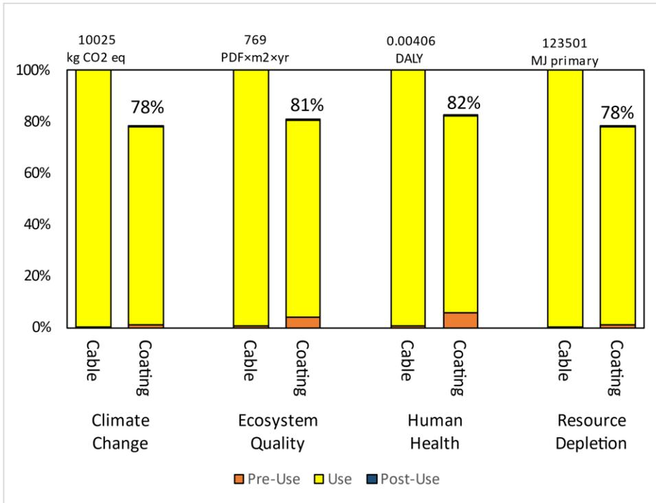
Figure 6 - Comparison of the potential environmental impacts for the two heating systems, with results shown for 5-meters of freeze protection for ten years in Alberta
