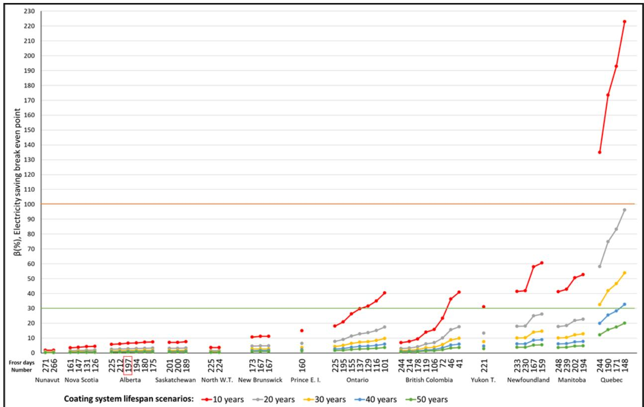
Figure 11 - Electricity saving break-even point of coating system sensitivity to coating system lifespan
