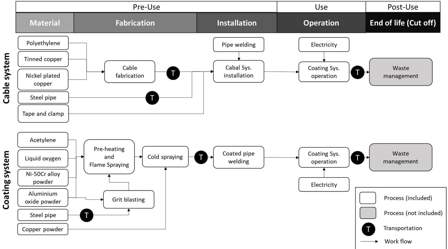
Figure 4 - Life cycle stages of heating systems
