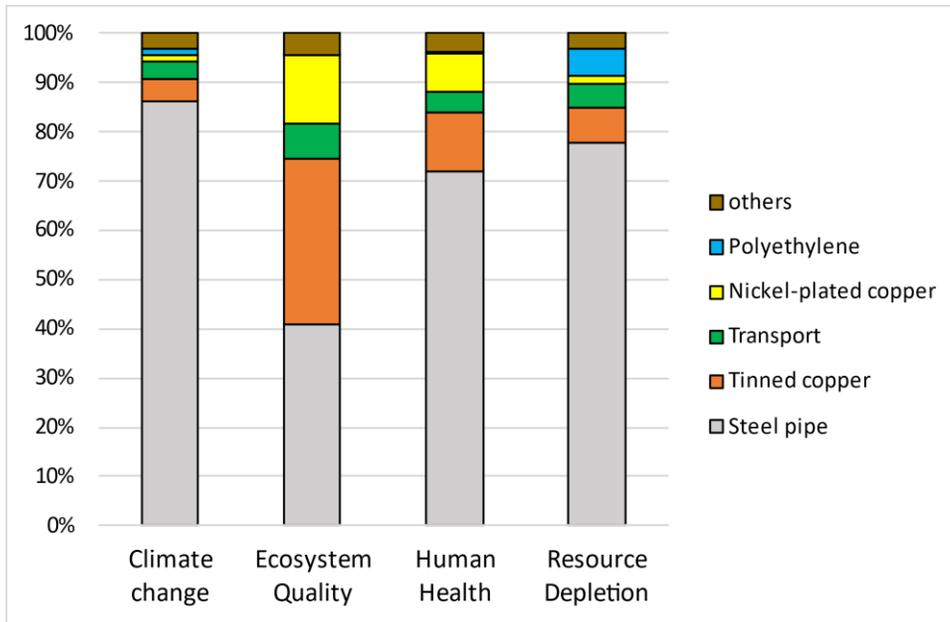
Figure 7 - Cable system impact contribution in production and installation phases
