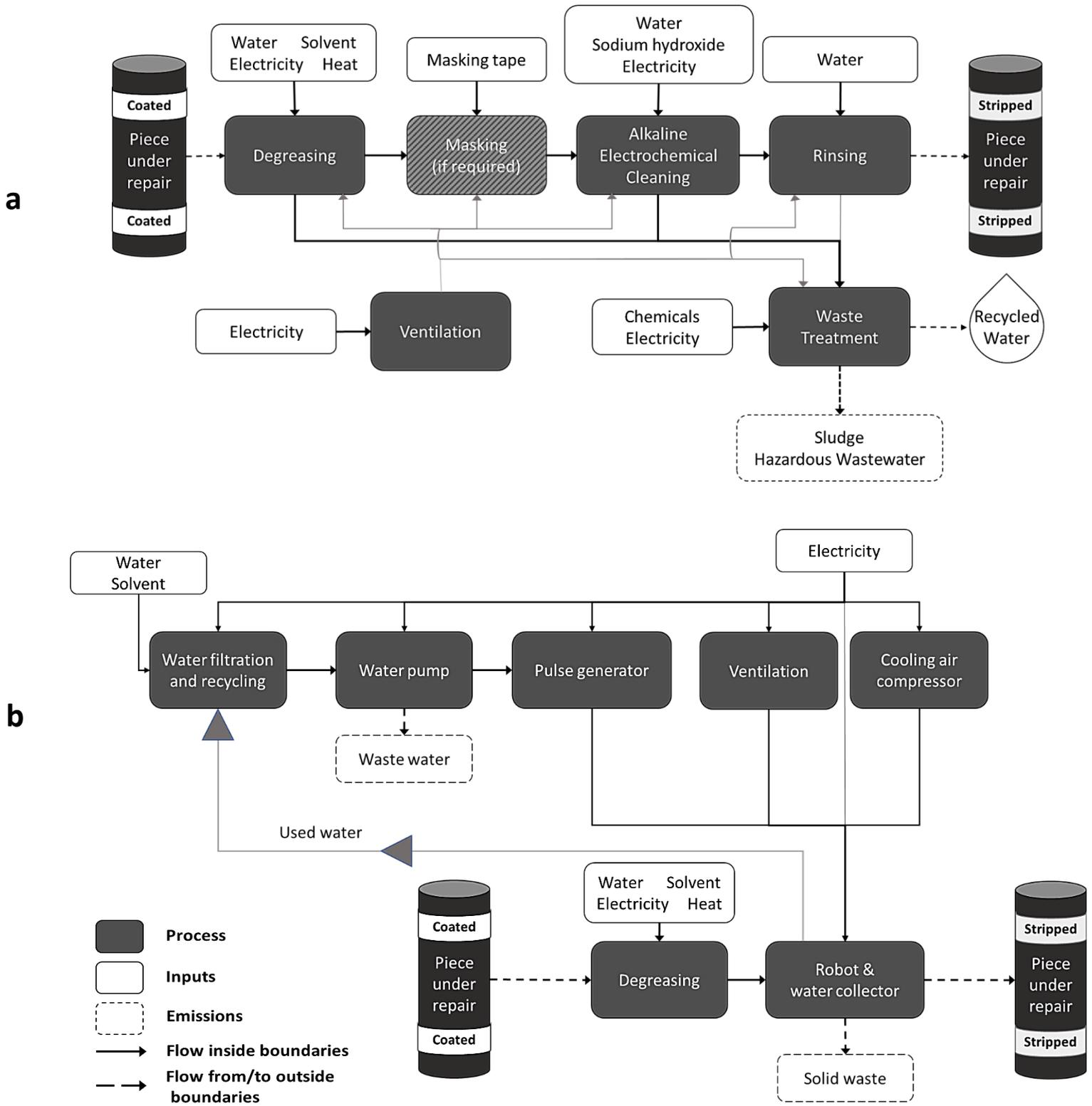
Figure 14 - Removal process flow a) Alkaline electrochemical cleaning, b) Pulse water jet
