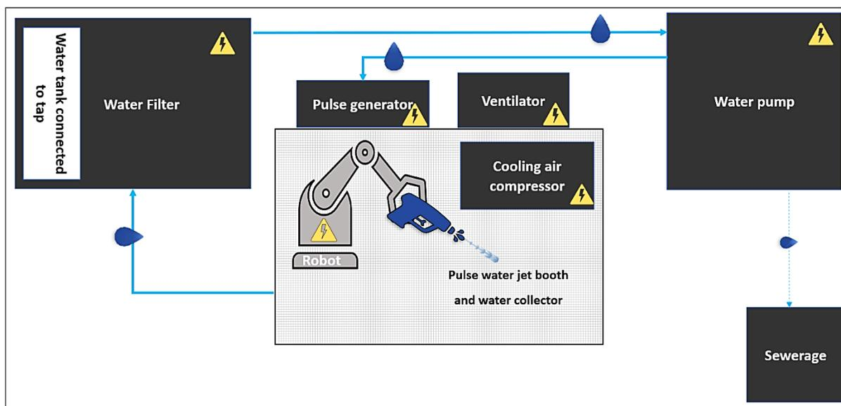
Figure 13 - Pulse Water Jet technology schematic sub-systems' layout
