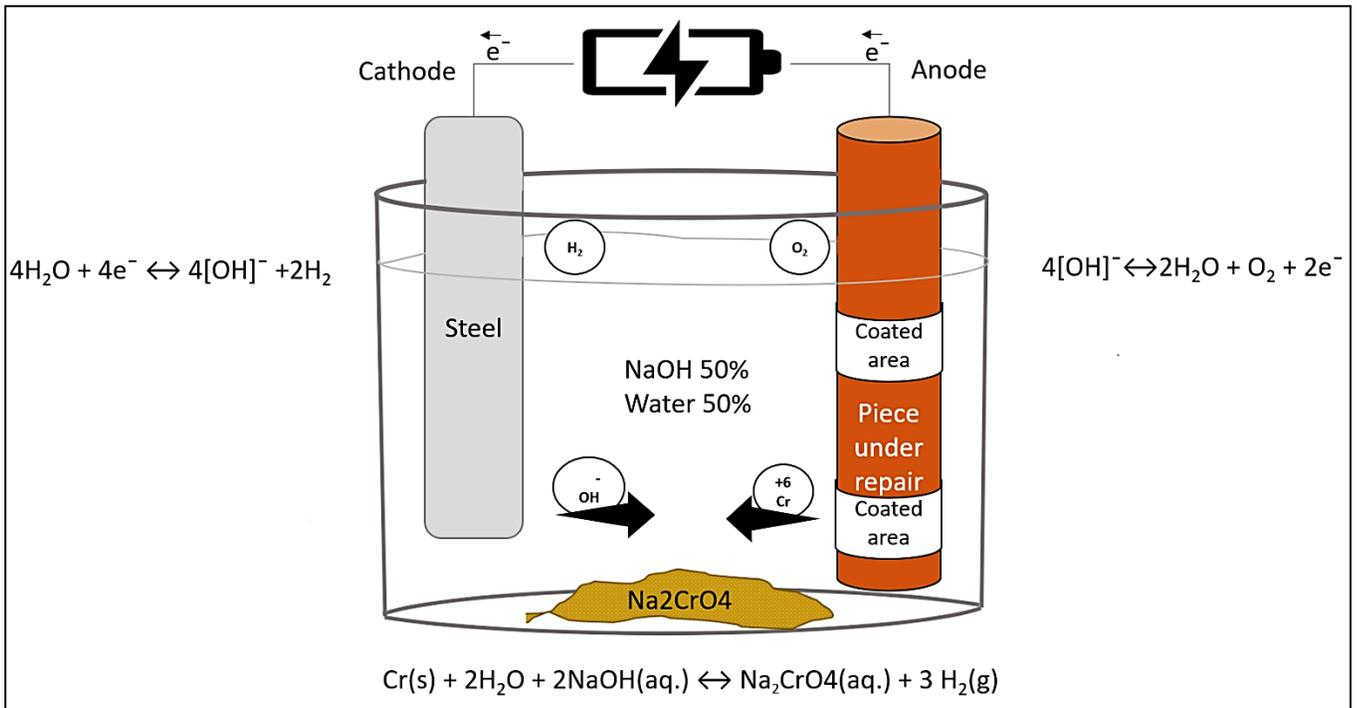
Figure 12 - Alkaline Electrochemical Cleaning, schematic electrolytic system
