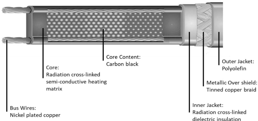
Figure 2 - Schematic picture of heating cable layers
