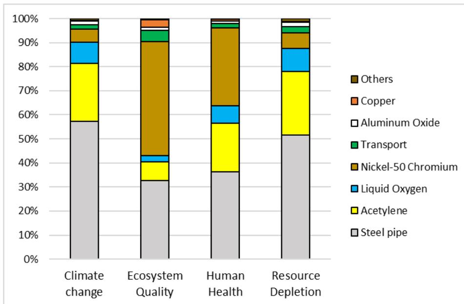
Figure 8 - Coating system impact contribution in production and installation phases
