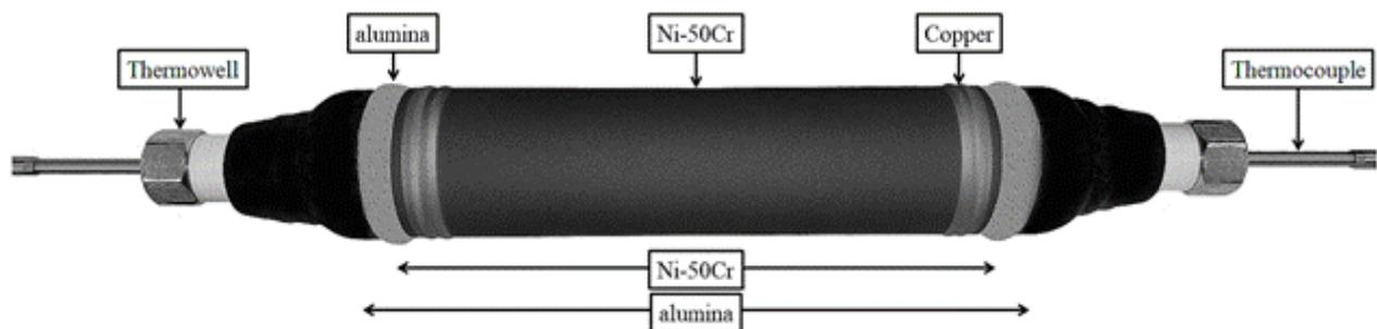
Figure 3 - Schematic of coating system layers
