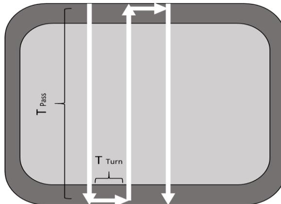
Figure 16 - Illustration of the time needed for pass and turn in PWJ
