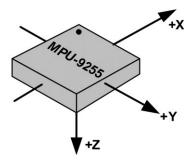
Figure 2.7: MPU-9250 Magnetometer Axis
