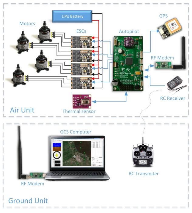
Figure 7.15: System architecture, air, and ground
