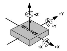
Figure 2.6: Axis of the Accelerometer and Gyroscope
