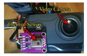
Figure 7.12: Thermal sensor and video camera installation
