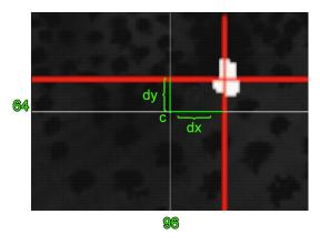
Figure 7.5 High-temperature area's centroid
