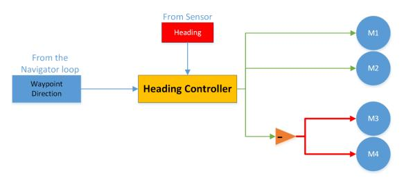
Figure 7.4: Navigation loop direction controller diagram
