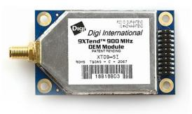
Figure 5.4: Wireless data module
