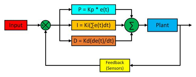
Figure 6.3 PID controller
