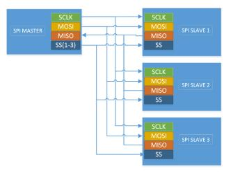
Figure 6.4 SPI BUS Block diagram
