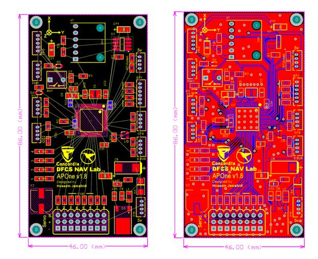
Figure 2.12: APOne v1.7 PCB before connecting the components
