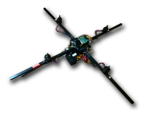
Figure 7.16: Assembled drone
