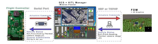
Figure 5.1: The components' connection diagram
