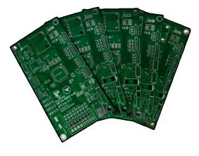
Figure 2.14: APOne v1.7 Printed board before assembly
