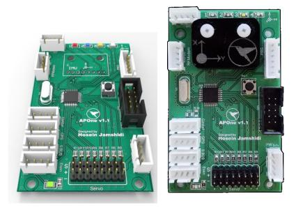
Figure 2.4: APOne v1.1 board and the PCB layout
