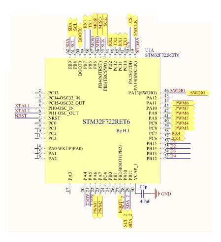
Figure 2.11: APOne v1.7 Microcontroller Pin Allocation
