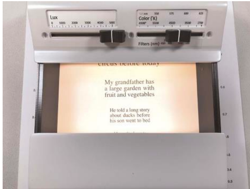
Figure 1. The LuxIQ. The LuxIQ is a standardized assessment tool that can be used to determine optimal colour and illumination to facilitate reading in individuals with low vision. Reading material, e.g., the MNread, is placed under the LuxIQ, then patients are instructed to adjust the sliders on the top of the device to their preference. The slider on the left controls luminance; luminance values range from 0 to 5000 lux. The slider on the right controls colour temperature and/or hue; colour temperature values range from 2700 to 4500 kelvin and colour hue values ranges from 525 to 625 nanometers.
