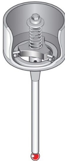
Figure 1.2: Interior of typical kinematic touch trigger probes
