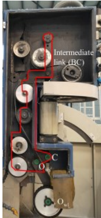
Figure 2.31 The intermediate rod on the other side of the pseudo headstock
