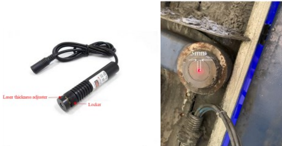
Figure 2.28 Laser transmitter and linkage center hole
