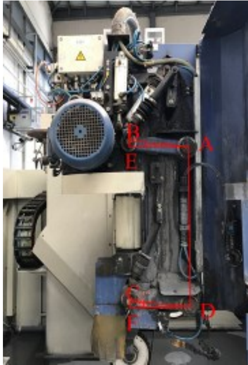
Figure 2.29 Four-bar linkage mechanism
