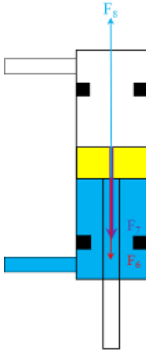
Figure 2.10 Piston force analysis
