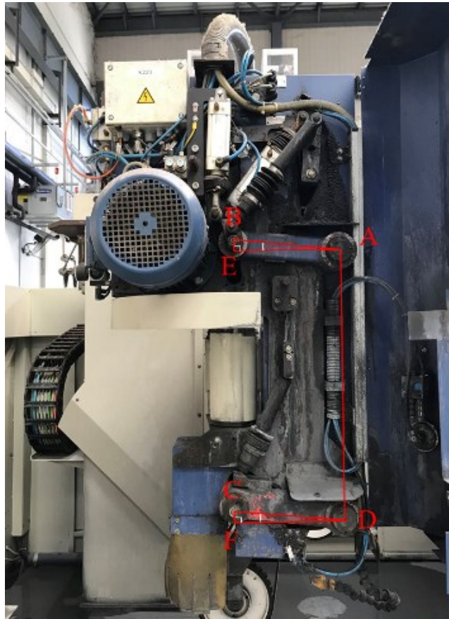
Figure 2.25 Four-bar linkage mechanism of the sanding belt wheel
