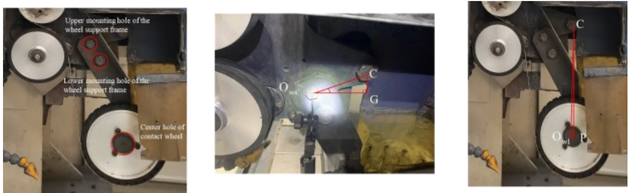
Figure 2.30 Geometric illustration of the support frame
