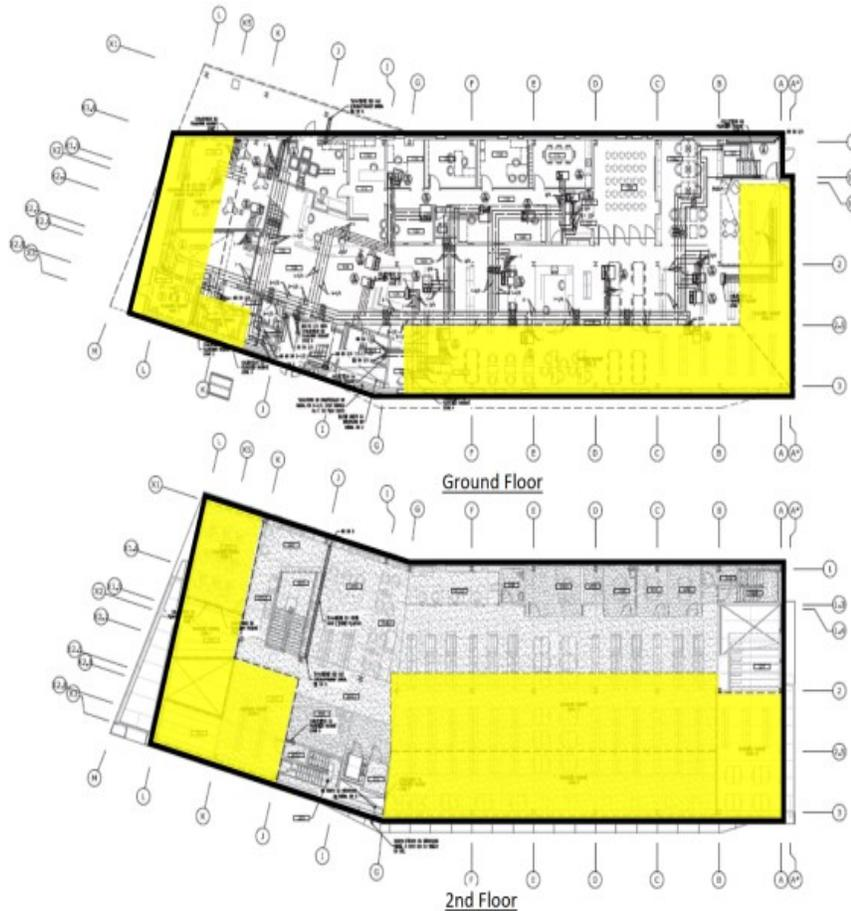
Figure 3-2: Architectural plan view with yellow area highlighting hydronic radiant slab (Dermardiros, 2020).
