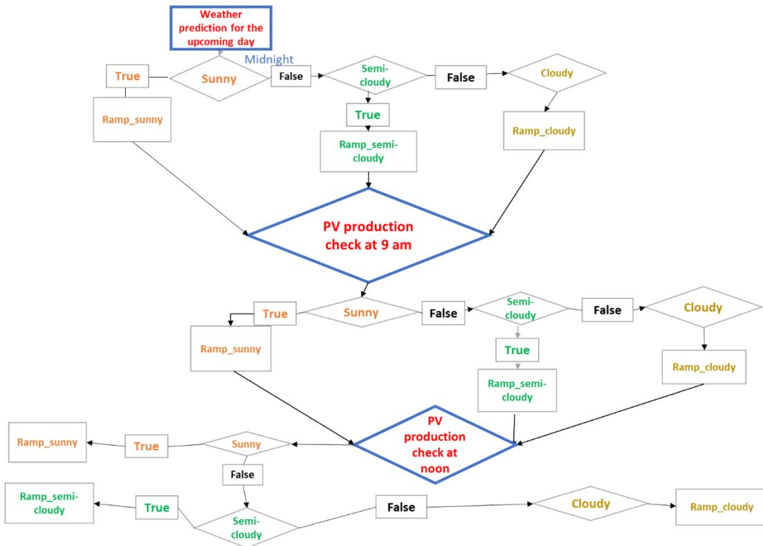
Figure 4-11: High-level control algorithm for very cold days. Initial one-day ahead weather prediction is verified through PV power generation data at 9 am and at noon.
