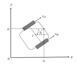
Figure 20: Schematic of Pioneer P3-DX robot.
