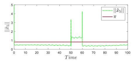
Figure 12: Residual signal of agent 5 in case 2: attack on sensor channel of agent 5.
