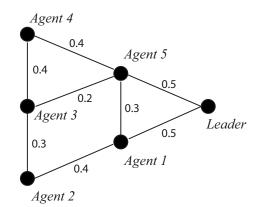
Figure 5: Communication topology and formation shape.
