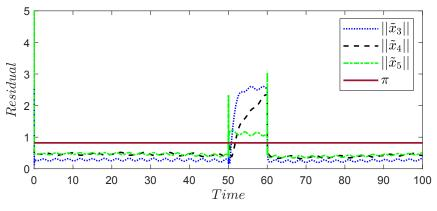
Figure 16: Residual signal of under attacked agents.
