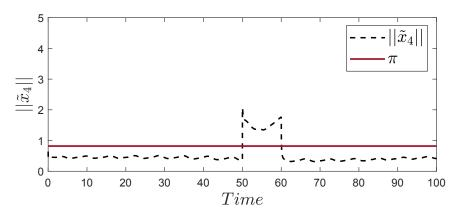
Figure 14: Residual signal of agent 4 in case 3: attack on the neighbouring communication channel of agent 4.
