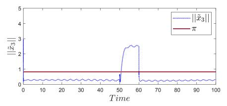
Figure 10: Residual signal of agent 3 in case 1: attack on the actuator channel of agent 3.
