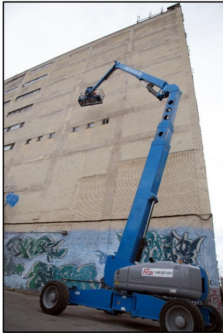
Figure 2.23: Genie telescopic boom lift. Mural Festival 2017. Photo by Kris Murray.
