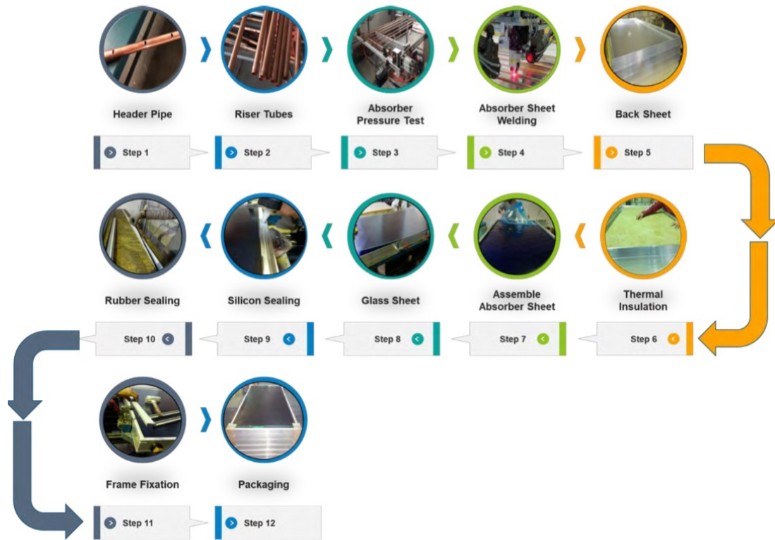
Figure 20 Flow chart of flat plate collector manufacturing[55]
