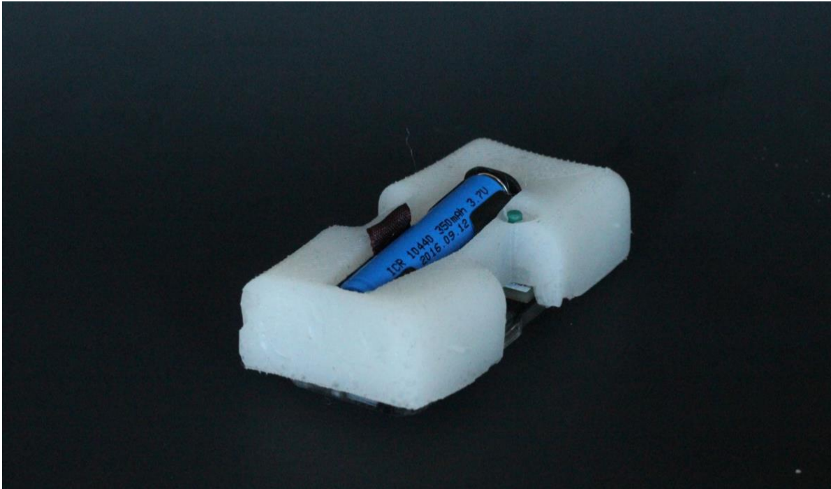
Image 3.2: A Vibropixel module in silicone casing
