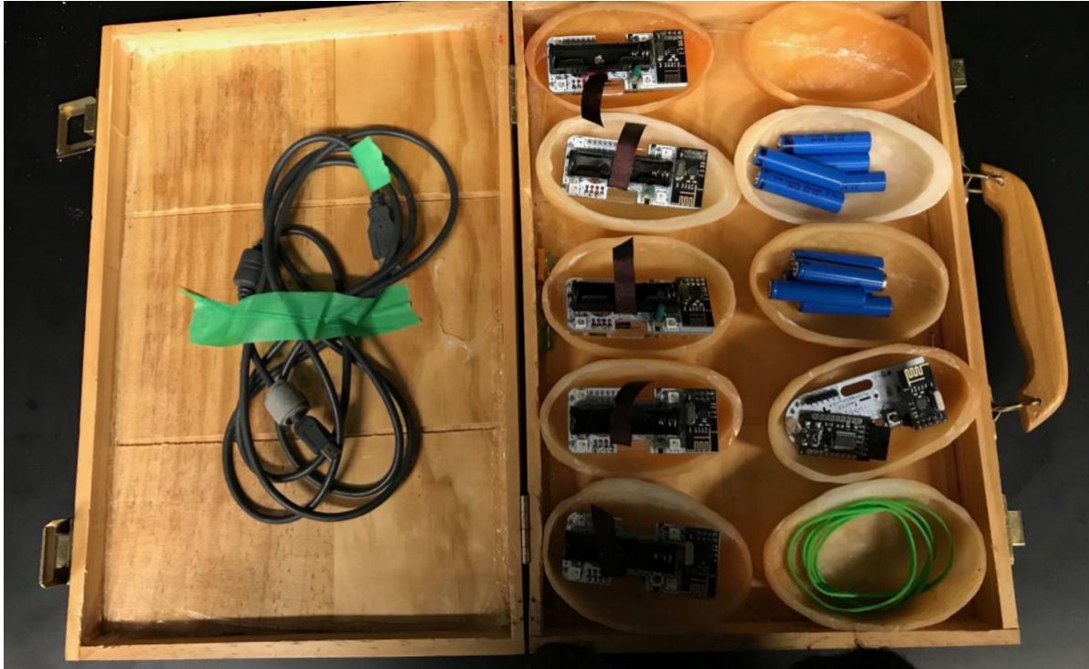
Image 3.3: A set of five Vibropixels, antenna, batteries, cables and early DIY casing
