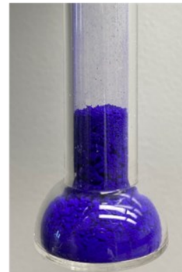
HKUST-1 (STEPOSOL) post-activation, 1.2 g (under vacuum and heat)
