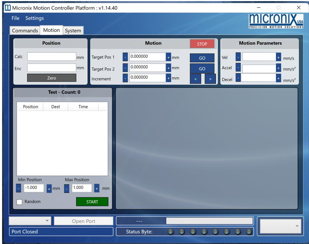
Figure 2.12: The image shows the graphical user interface of the precision positioner control software. Control software allows control of the precision positioner in three directions with the step size as small as 1 nm.
