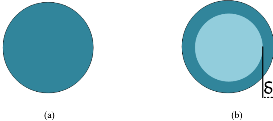
Fig. 2.19 The current distribution in a conductor: a) uniform distribution occurring at dc, and b) skin effect where the current density is reduced with the direction of the inductor core.
