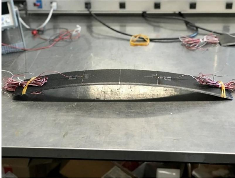
*Figure 1.1: A curved leaf spring made using 4D printing*
