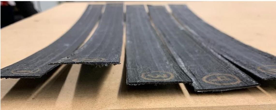
*Figure 2.1: Distortion of composite laminates during and after manufacturing process*
