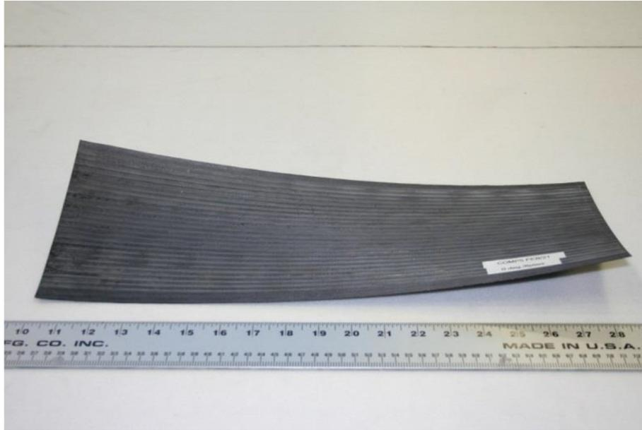
Figure 1.3: A deformed unidirectional thermoplastic laminate made by AFP process
