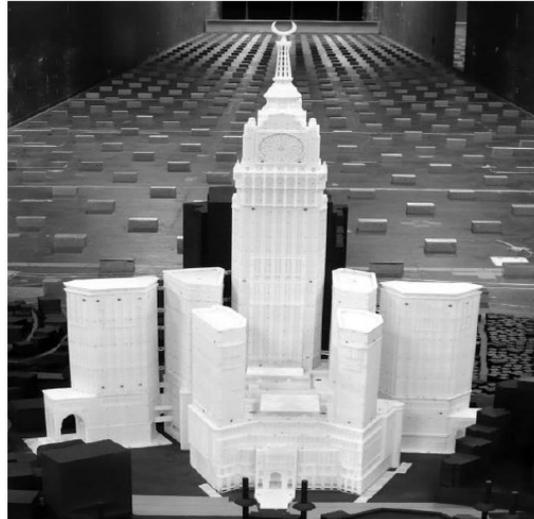
Fig. 2.13. Wind tunnel test for a tall building in a compound (El Damatty and Elezaby, 2018).
