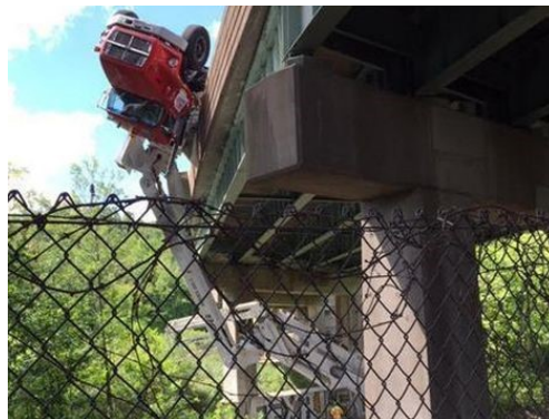
Figure 1-2. Failure of a cherry picker during under-bridge inspection (The Vertikal Press, 2015).
