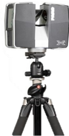
(a) TLS using tripod (FARO Technologies Inc., 2012)
