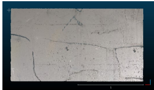
Figure B-1. A segment of a concrete bridge including defects in Cloud Compare.
